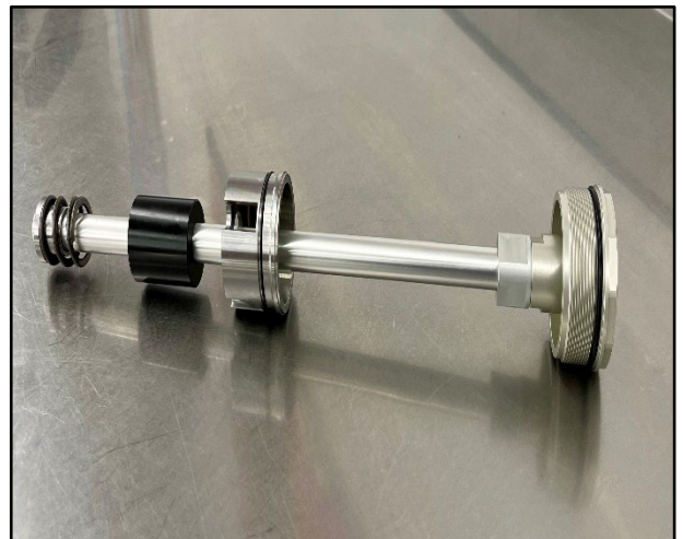
Cartridge rod assembly with X-Pro fork lowering spacer.
