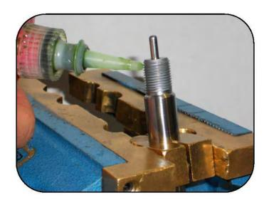
Apply a few drops of high strength thread locker to the shaft threads.
