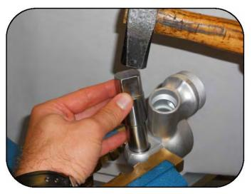
Flip the base and secure in the vise. Using the correct size metal tool, tap out the uniball. Note: The uniball can only be removed from the side with the snap ring groove.
