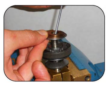
Remove the rebound valve stack of shims.
