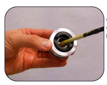
Grease the guide shaft seal circumference with Nitrile rubber O-ring grease .
