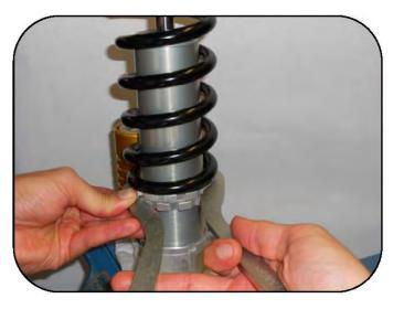
Using 2 wrenches (00529000087), tighten the preload ring against the counter preload ring.
