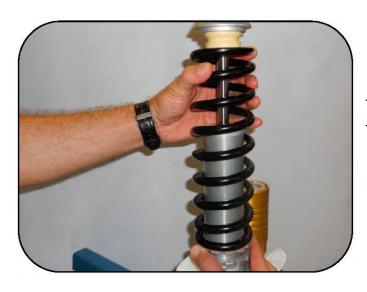
Unscrew the preload ring far enough to reveal the rubber bumper over the top of the spring.
