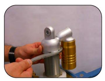
Tighten the lock ring on the base using your preload spanner wrench (00529000087)
