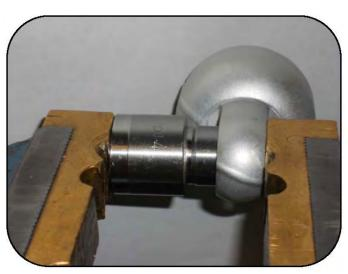
Using a vise, press the uniball into the base from the side that has the snap ring groove.
