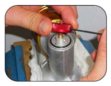
Place the compression adjuster knob on the assembly being sure to align the locking screw with the locking hole on the assembly.
