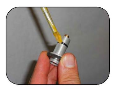
Lightly grease the O-ring on the compression assembly.
