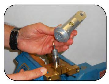
Remove the clevis from the shaft.
