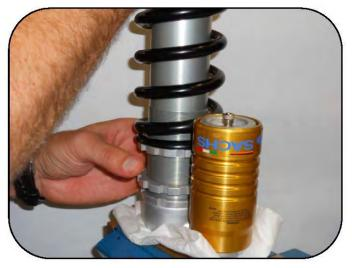
Tighten the spring preload ring by hand and switch to the wrench (005299000087) when it starts to load.
