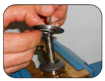
Remove the compression valve stack of shims.
