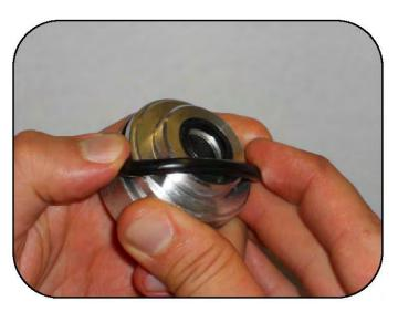
Install the outer shaft guide O-ring.
