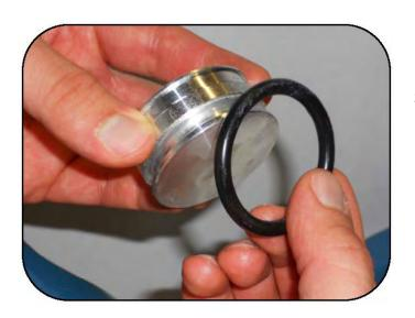
Remove the O-ring from the diaphragm separator.
