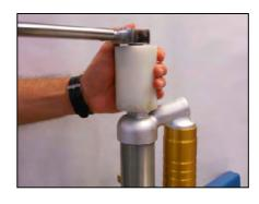
Shock base to shock body 150Nm
