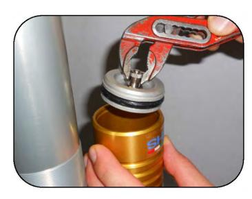
Using pliers, pull up on the tank valve cap until it is removed from the tank.
