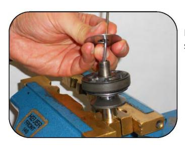
Install the calibrated rebound shim stack onto the shaft assembly.
