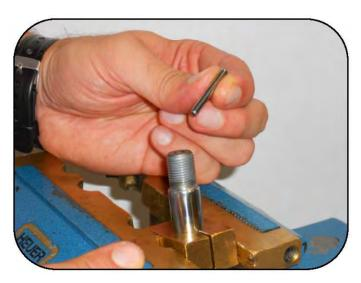
Remove the rebound regulating pin from the hole in the end of the shaft.
