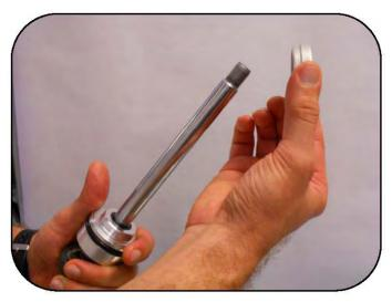
Remove the body end cap from the shaft.
