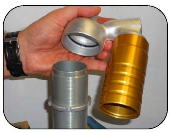
Remove the base form the shock body.
