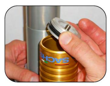
Insert the cap into the tank.
