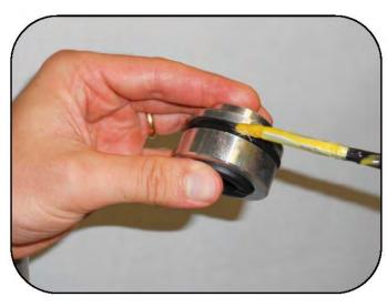
Using the same grease, apply to the entire circumference of the O-ring.
