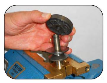
Insert the piston on the shaft making sure the 4 square holes are facing downward.
