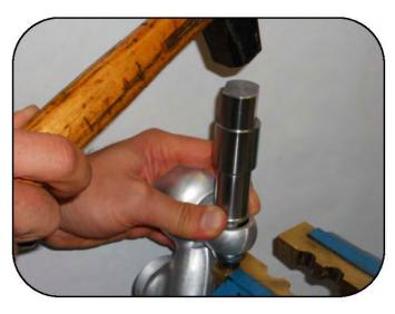
Tap the sleeve with a hammer until the bushings are completely seated.
