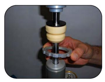
Remove the counter preload ring.
