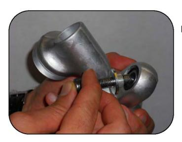
Insert the flange bushing using a bolt.
