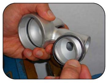
Remove the O-ring from the tank side of the base.
