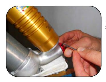
Use an Allen wrench to loosen the high speed compression dial lock nut.
