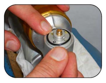
Place the O-ring onto the compression assembly.
