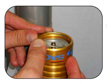
Insert the clip into the seat making sure it is installed completely.
