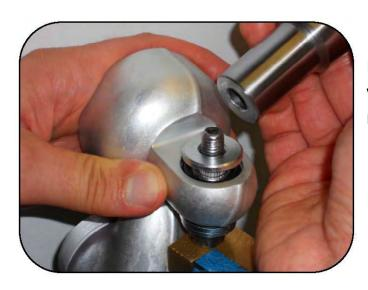
Resting the head of the bolt on the vise, place a metal sleeve over the bolt resting against the flange bushing.
