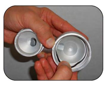
Insert the O-ring into the base, making sure it is seated completely.
