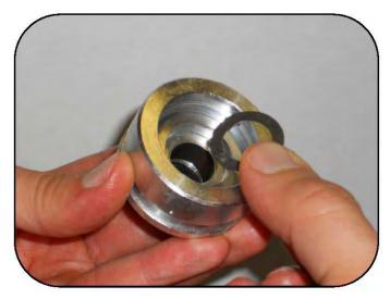
Place the oil seal support washer into the seat.
