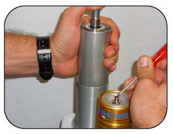
While keeping the shaft pushed down, push on the gas valve to release any trapped air.
