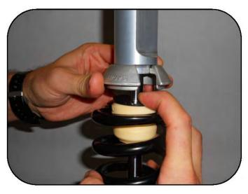
Push down on the plastic washer and rubber bumper to make room to remove the spring collar.
