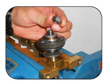
Remove the nut from the assembly.
