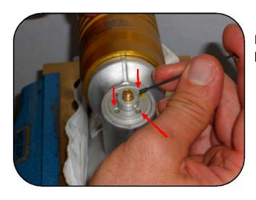
Insert the springs into the greased holes.
