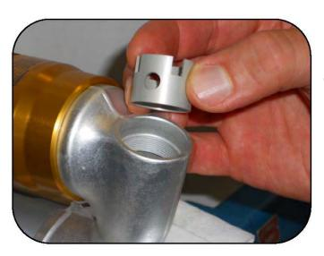
Insert the compression adjuster observing the orientation In the photo.
