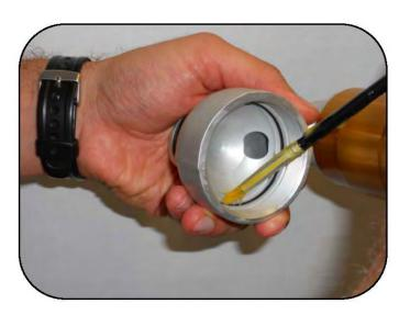
Lightly grease the inner base O-ring area.
