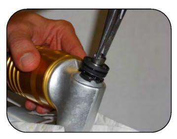
Remove the compression valve assembly.
