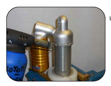
Using a torch, heat the base locking ring.
