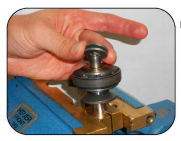
Place the 2 spacers onto the shaft.
