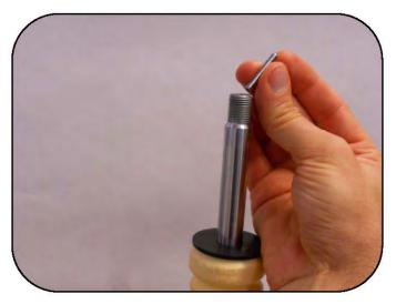
Install the shorter steel adjustment rod.
