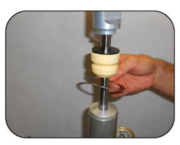
Now that the spring is off the shock, remove the spring washer from the preload ring.
