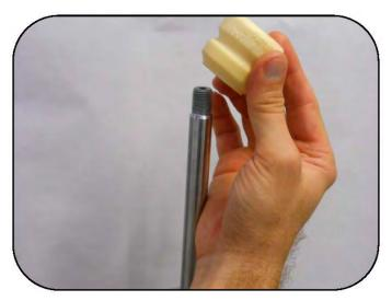
Install the bumper stop on the shaft.
