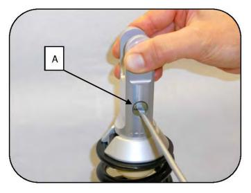
Check and record the location of the rebound adjustment. To do this, turn the dial clockwise until it stops, noting the number of "clicks" made by the dial (A). Then turn the dial counter clockwise until fully open.
