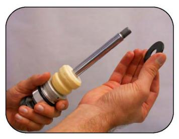
Remove the bumper plastic washer from the shaft.
