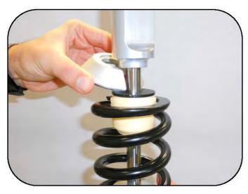
With the rubber bumper out of the way, lower and slide out the spring support collar.
