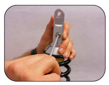
Turn the rebound adjusting screw all the way in then back out the number of clicks recorded before removal.
