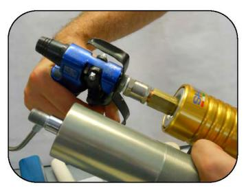
Pressure the tank with nitrogen to 130+/- 25 PSI for the 2T and 145+/- 25 PSI for the 4T.
