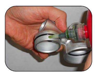
Apply a medium strength thread locker to entire circumference on the threads of the tank side of the base.
