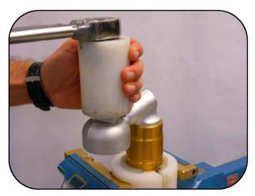
Secure the tank in a vise using the shock body plastic jaws (00529000089)
