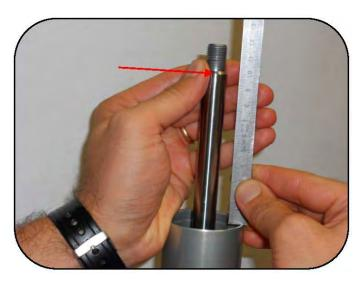
Position the shaft so the chamfer just below the threads is 100mm from the edge of the body.
