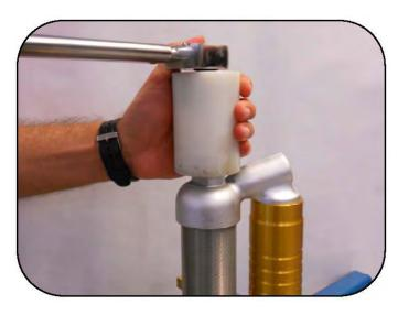
Secure the damper body to the vise using the plastic jaws (00529000089). Using the base socket bushing (00529000090) and a torque wrench, tighten to 150Nm.
