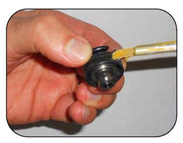
Lightly grease the O-ring on the compression valve assembly.
