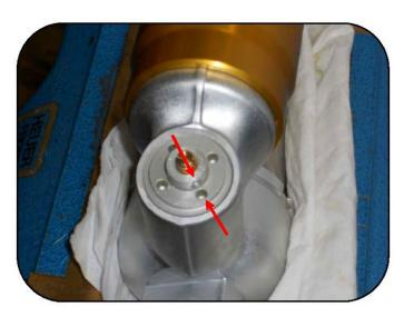
Align the locking hole of the knob with one of the 4 holes on the compression assembly. Note the arrows in the photo.
