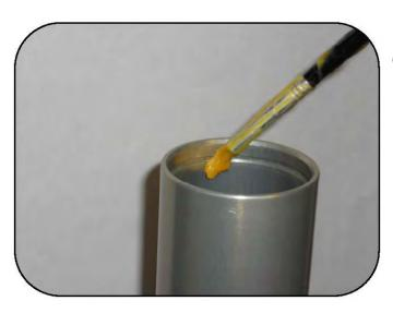
Grease the inner edge of the damper.
