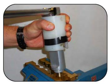
Being careful that the clevis is hot, loosen the clevis form the shaft using the clevis socket bushing tool (005299000090)
