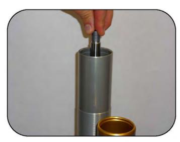
Push the shaft in until it rests on the bottom of the shock body.
