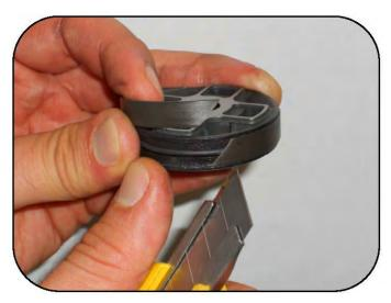
Use a cutter to remove the Teflon band from the piston.
