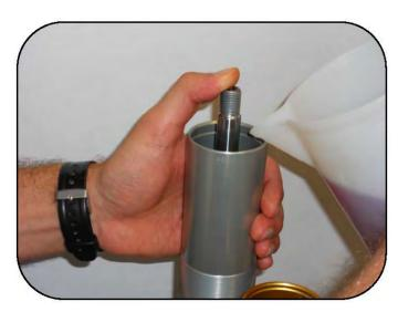
Keeping the shaft seated, fill the body with oil.
