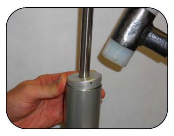
Place the body cap on the shaft. To seat the cap, place it on the shock body and lightly tap around the circumference with a rubber mallet.
