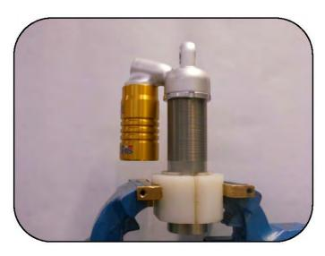
Using the plastic jaws (005299000089) secure the shock body in the vise.
