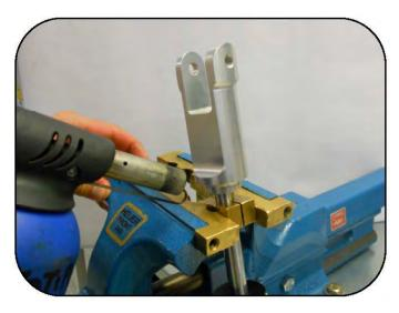
Heat the junction of the shock clevis and the shaft with a torch.
