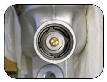
Note that the square edges of the assembly fit into the grooves on the adjuster.
