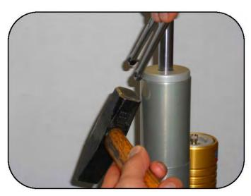
Insert the round end of a wrench or use a punch and lightly tap to raise an edge of the shock body cap.
