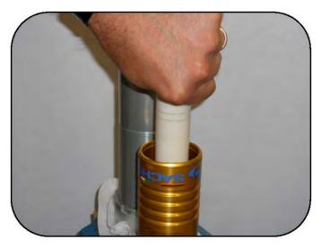
Keeping the shaft seated, push the diaphragm in until it stops against the bottom of the tank.
