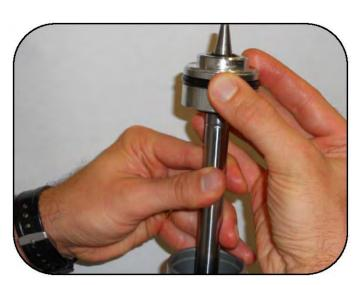
Keeping the shaft position fixed, slide the guide onto the shaft observing the orientation in the photo. .
