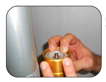
Push down on the reservoir tank cap to expose the snap ring.
