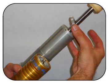
Slide on the spring counter preload ring and screw it down toward the base.
