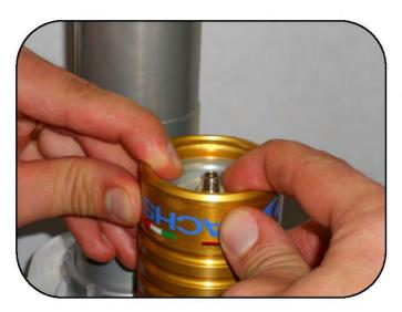
Push the cap in enough to expose the snap ring seat.
