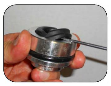
Pry off the rubber extension limiter from the shaft guide.
