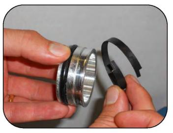
Remove the Teflon coated band from the diaphragm separator.
