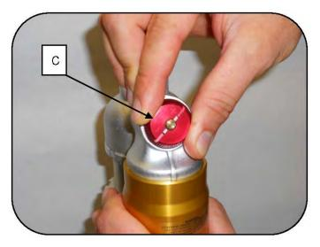
Check and record the position of the high speed compression dial (c). To do this, turn the dial in until it stops, noting the number of "clicks". Then turn the dial counter clockwise until fully open.
