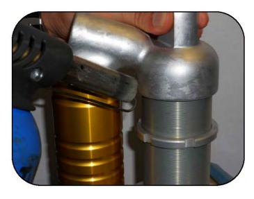
Heat the junction of the base and shock body with a torch.
