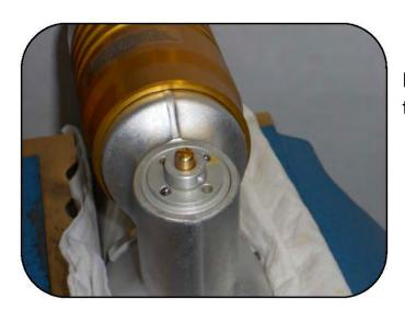
Insert the bearings into the holes with the springs.
