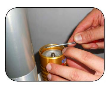
With a screw driver, pry up on the tank snap ring being careful not to scratch the inner side of the tank.
