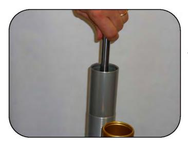
Raise and lower the shaft a few times making sure the piston never leaves the oil. This will help to bleed out any air trapped below the piston.
