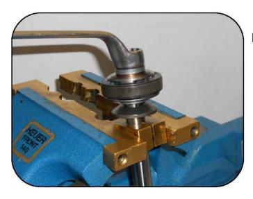
Loosen the nut on the piston assembly.
