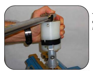
Tighten to 70Nm using the shock clevis socket bushing (005299000090) and a torque wrench.
