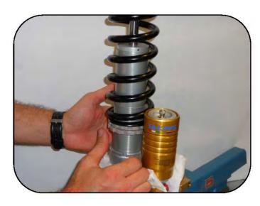
Spin the spring counter preload ring up against the preload ring.
