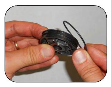
Remove the O-ring from the piston. Always replace the O-ring as it is always damaged from cutting off the Teflon band.
