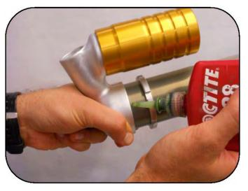
Apply a high strength thread locker to the external threads on the body near the base.
