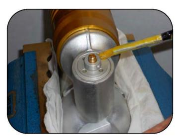
Lightly grease 2 holes opposite each other perpendicular to the locking screw hole.
