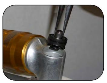
Place the compression valve assembly into the base opening noting the orientation in the photo.
