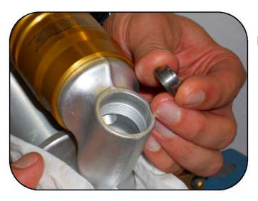
Remove the spring guide bushing.
