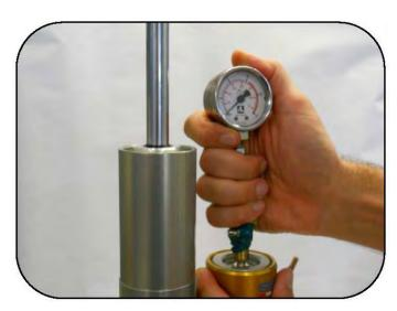
Check the pressure with a reliable and calibrated gauge.
