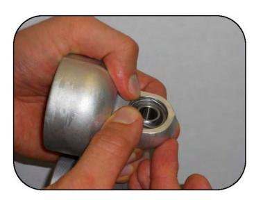
Install the snap ring making sure it is seated the entire circumference of the groove.
