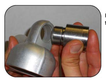
Place the uniball at the side of the base that has the snap ring groove.
