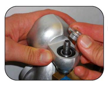
Insert the other Flange bushing on the bolt.
