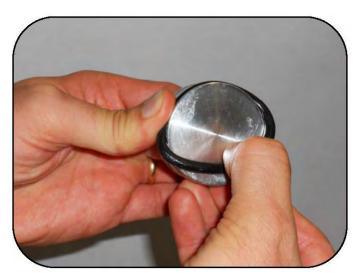
Install the outer diaphragm O-ring.
