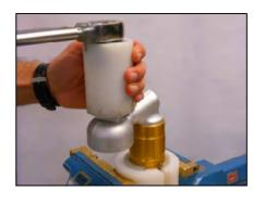
Shock base to reservoir tank 50Nm
