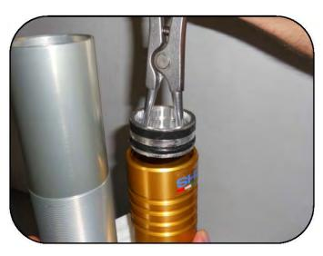
Using reverse needle nose pliers or snap ring pliers, remove the separator diaphragm completely from the tank.
