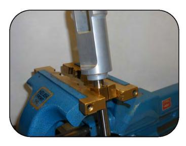
Lock the shaft into the vise using the brass shaft jaws (005299000091)
