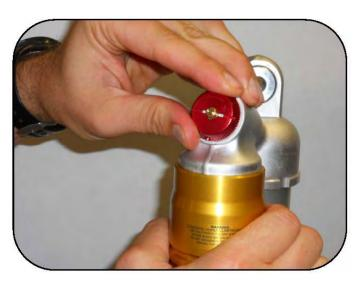
Turn the high speed compression adjuster all the way in then back out to the pre removal setting.
