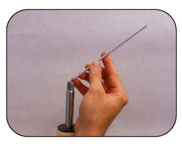
Install the aluminum rebound adjustment rod.
