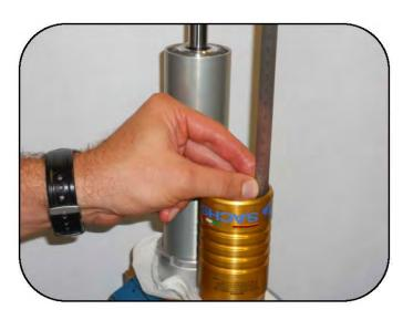
The diaphragm pushed all the way in should be 65mm measured from the edge of the tank .
