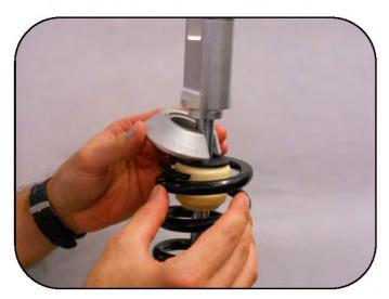
Slide in the spring support collar and center it on the clevis.
