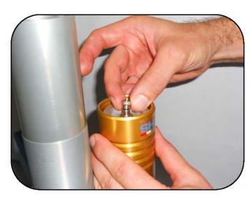
Screw the cap back on the tank valve.
