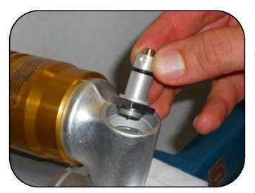
Insert the compression assembly into the base.
