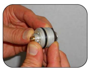
Hold the assembly and with your thumbs, push on the center removing it from the housing .
