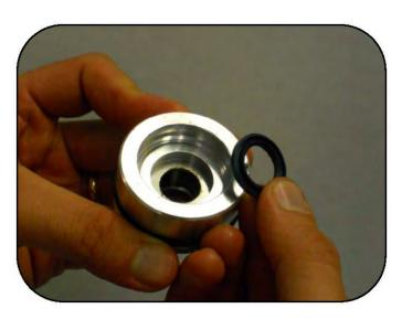
Remove the oil seal from the shaft guide.
