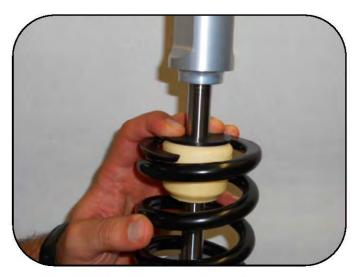
Slide the plastic washer and bumper down to make room for the spring support collar.
