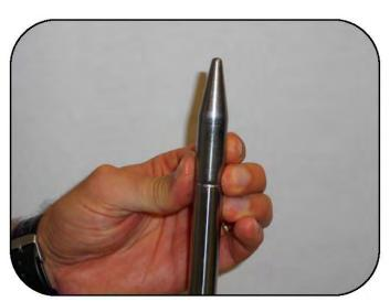
Apply the shaft sleeve to the end of the shaft. (005299000093)
