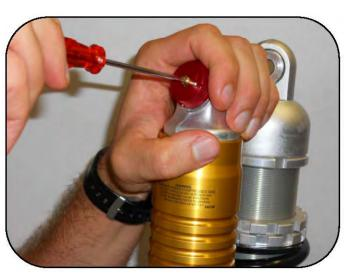
Turn the low speed adjuster all the way in and then back out the number of clicks recorded before removal.
