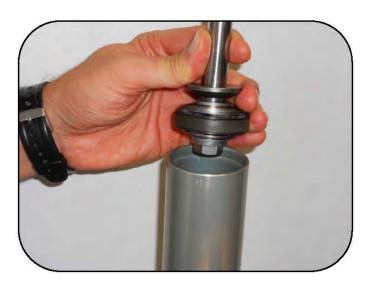
Insert the piston into the shock body.
