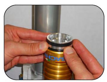
Insert the diaphragm into the tank with the hollow side up.
