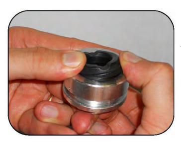
Place the rubber extension limiter into the guide.
