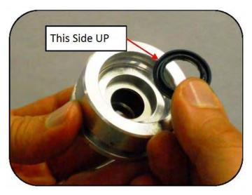
Insert the oil seal into it's seat with the grooved side facing up.
