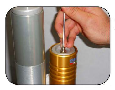
Press the center of the valve to release all pressure from the tank.
