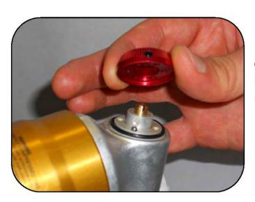
Remove the high speed compression dial making sure not to loose the 2 bearings and 2 springs located underneath.
