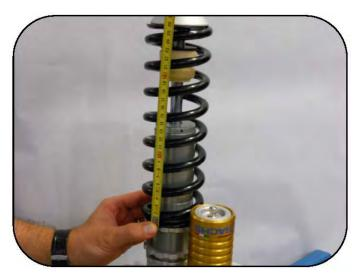
Tighten the spring preload ring until the spring is at the pre removal length.
