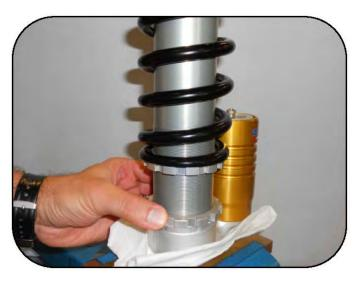
Screw the counter ring down towards the base to unload the rings.
