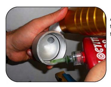
Apply a medium strength thread locker to the entire circumference of the inner threads of the base.
