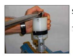
Shock clevis to shock shaft 70Nm
