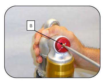
Check and record the position of the low speed compression dial adjustment. To do this, turn the dial (B) clockwise until it stops, noting the number of "clicks". Then turn the dial counter clockwise until fully open.
