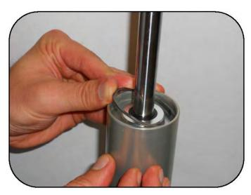
Insert the guide snap ring into the seat making sure it is installed completely.
