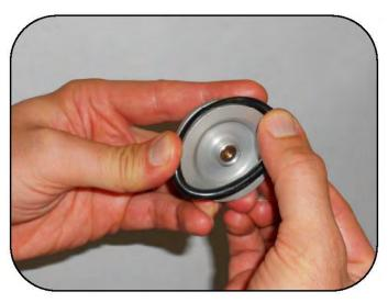
Install the O-ring on the outer edge of the reservoir cap.
