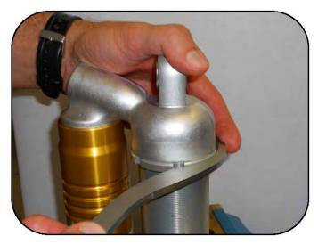
Being careful that the base is hot, use the preload spanner wrench (005299000087) to loosen the base lock ring.
