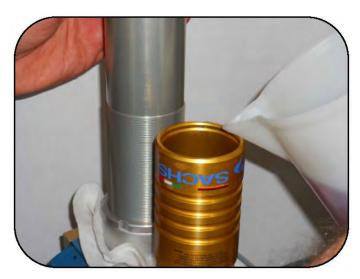
Secure the shock at it's base in a vise putting an absorbent rag between the jaws. Using Motul VI400 2.5-20W or an equivalent, fill the reservoir until it is flush with the edge.
