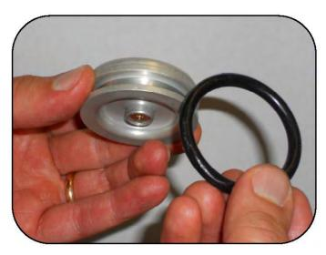
Remove the O-ring form the tank cap.
