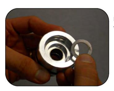
Remove the oil seal support washer from the guide.
