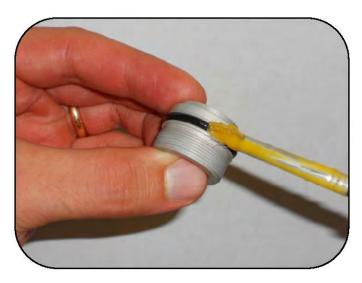
Lightly grease the O-ring on the outer edge of the compression housing.
