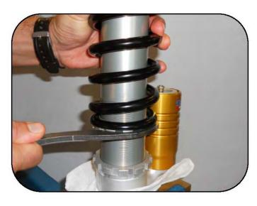
Unscrew the next ring towards the base to completely remove the spring preload.
