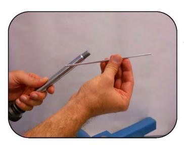
Remove the rebound adjuster rod from the hole in the end of the shaft.
