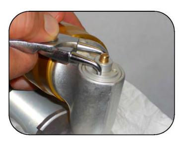
Using the compression assembly nut tool (AVT-0127-002-T01-3) or round nose pliers, unscrew the compression adjuster assembly.
