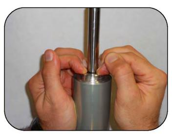
After the outer diaphragm O-ring has entered the body and has sealed, continue to push the guide down far enough to expose the snap ring seat. At this point, the shaft position is no longer critical.
