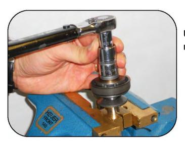
Using a torque wrench, tighten the nut to 40Nm.
