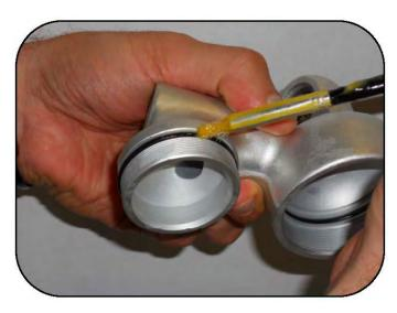
Apply a light coating of rubber nitrile grease to the tank side O-ring.
