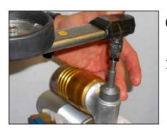
Compression adjuster assembly 14Nm
