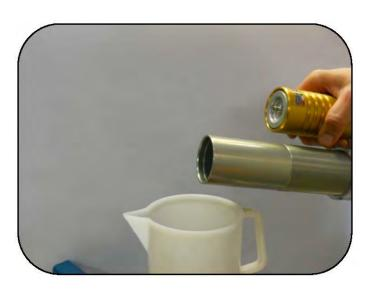
Drain the oil from the shock body.
