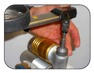
Tighten the compression adjuster assembly with the proper tool (AVT-0127-002-T01-3) and torque to 14Nm.
