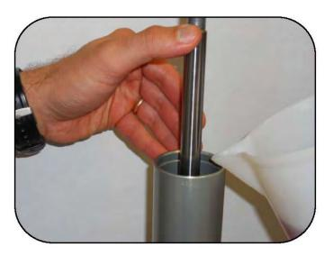
Keeping the shaft position fixed, fill the body with fluid until flush with the edge.
