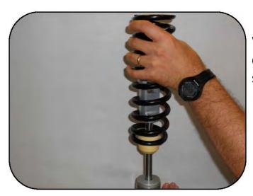
With the spring collar removed, you can now raise the spring off the shock.
