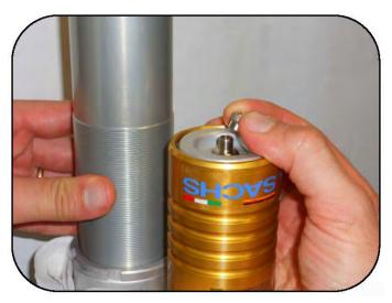
Screw the valve cap on and make sure it is tight.
