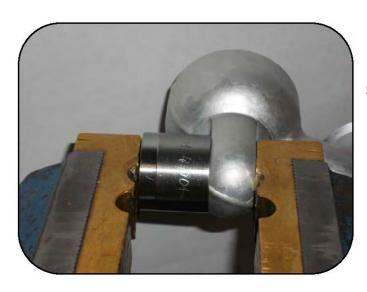
Press the uniball into the base until it slightly touches the bottom of the seat.
