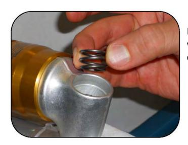
Place the conical spring in the opening with smaller diameter facing downwards.
