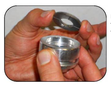
Insert the guide washer making sure the 4 groves are facing down toward the seal.
