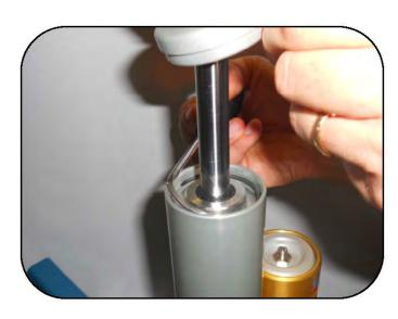
With a screw driver, pry up on the snap ring being careful not to scratch the inner side of the shock body.
