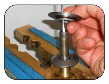
Lock the shaft into the vise using the brass jaws (005299000091), then install the calibrated compression shim stack.
