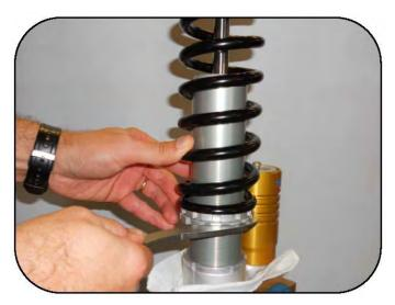
Secure the shock in the vise upside down then remove the spanner rings using the preload spanner wrench (005299000087).
