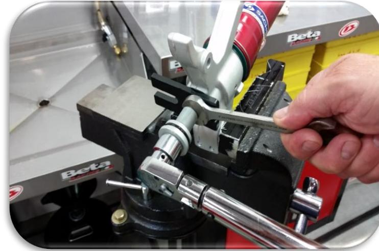
Turn the 15mm jam nut counterclockwise holding the rebound assembly with a torque wrench. Tighten to 10Nm.
