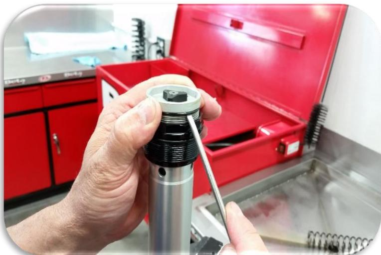
Carefully use the clip tool to help lift the compression assembly out of the cartridge.
