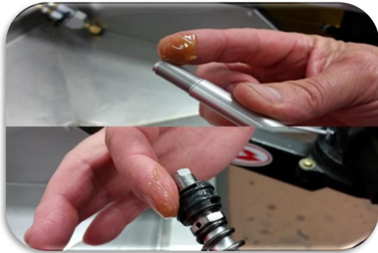
Apply seal and O-ring grease to the rebound rod (the rod, not the threads) and a small amount on the piston to hold the band in place.
