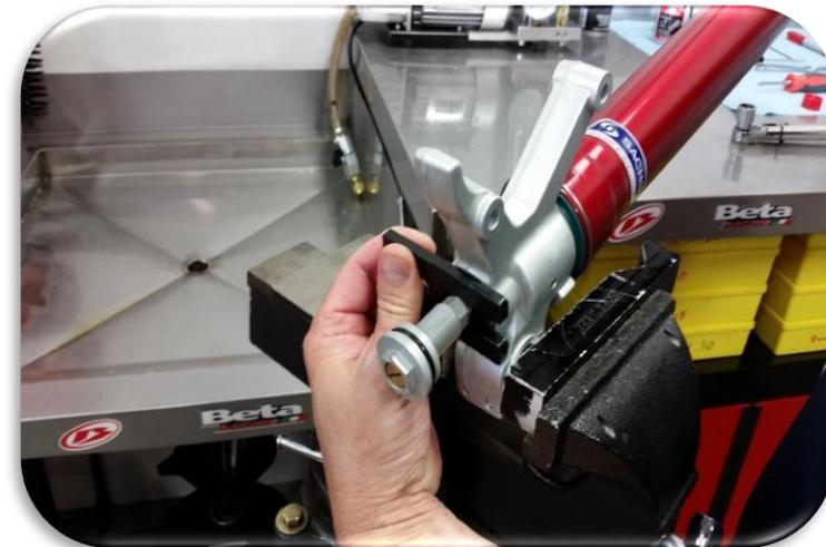
Press in on the cartridge and remove the holding tool.
