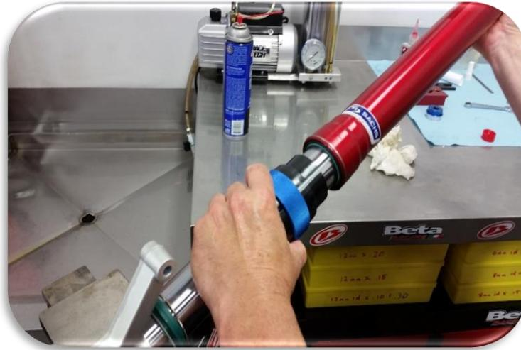
Install the fork seal and bushing into the outer tube using the seal driver.
