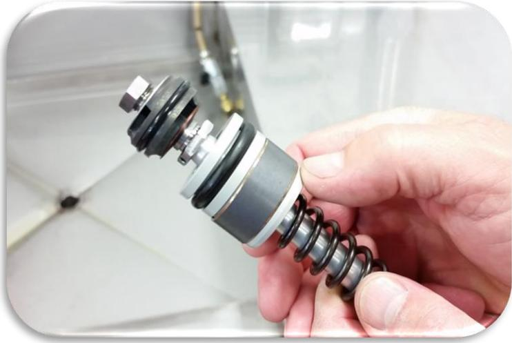
Inspect the O – ring and bushing, replace if damaged or worn.
