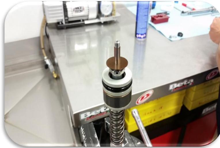
Clean the post then reinstall the shims in the order they were removed.
