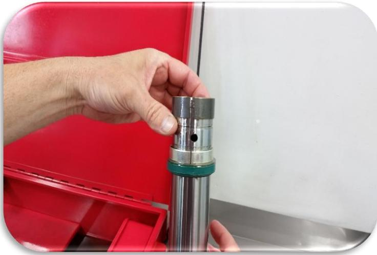
Remove the bushings, retaining washer, fork seal, retaining clip and dust seal paying attention to the order of removal and orientation.
