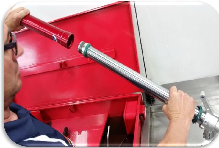
While holding the outer tube in one hand and the lower leg in the other, use one swift- strong motion to pull the outer tube off the lower leg.
