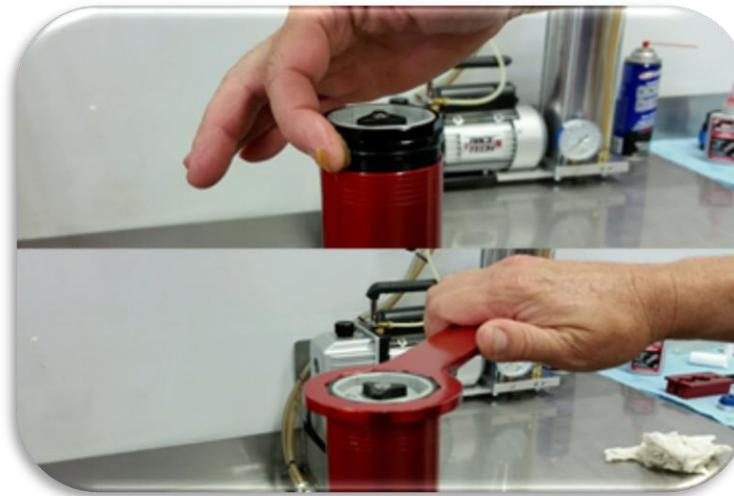
Secure the outer tube in the soft jaw vise. Apply seal and O-ring grease to the top cap O-ring and threads.
