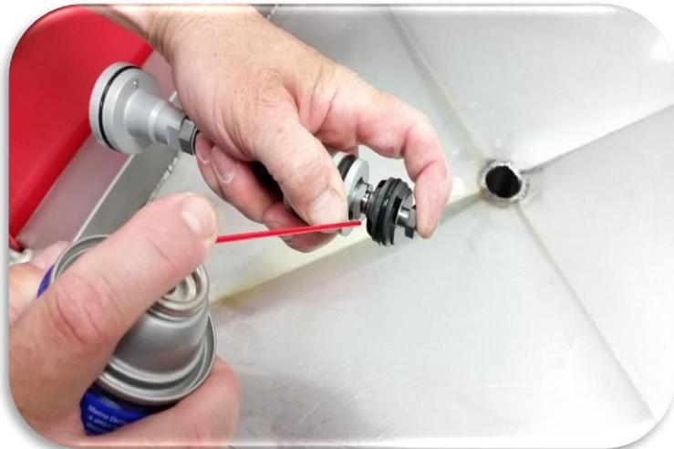
Install the check plate and nut **without** the spring loosely then clean the shim stack with contact cleaner then blow off with air.
