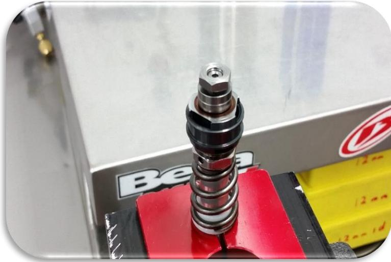
Remove the nut and apply 1 drop of red loctite. Carefully check that the delta shim is aligned then install the nut and torque to 5Nm.
