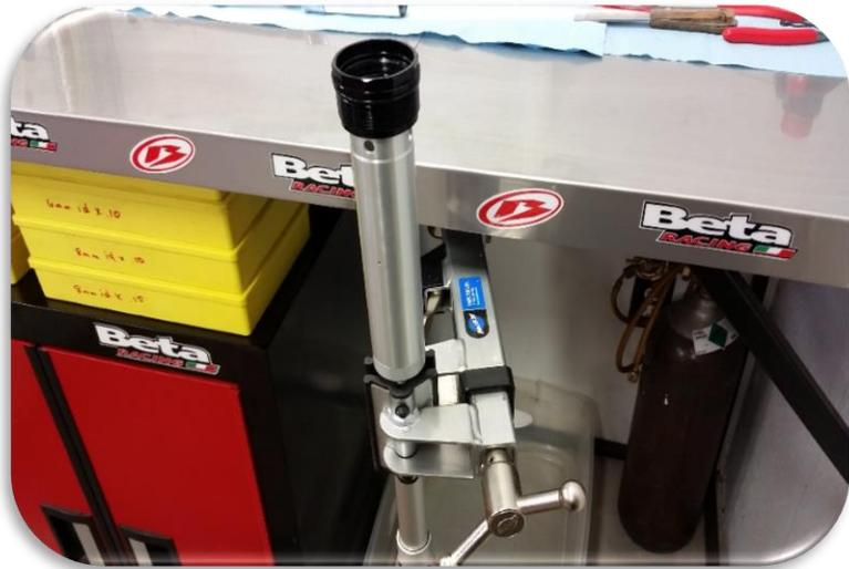
Secure the inner cartridge with a soft jaw vise or clamp.
