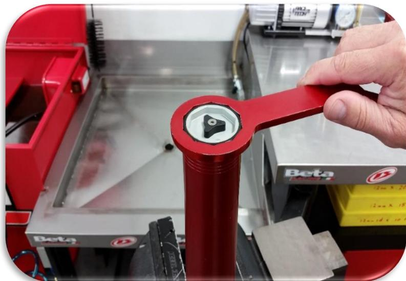
Unscrew inner cartridge from outer fork tube.
