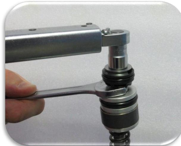
Reinstall the nut with the spring and tighten to 5Nm while holding the 17mm on the dampening rod post.
