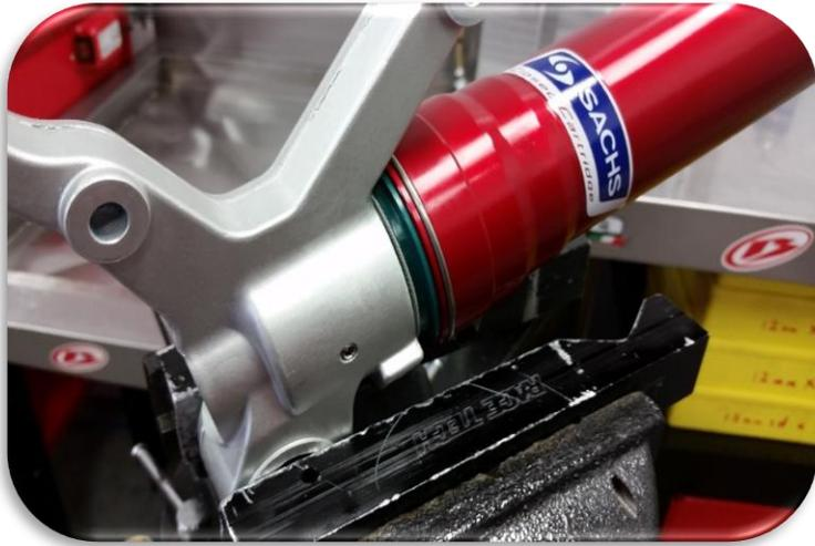
With the dust seal sitting against the fork lug, slide the outer tube down until the dust seal is seated.
