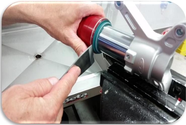
Separate the dust seal from the outer tube.
