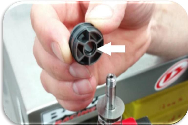
Install the rebound piston with the recess facing down.
