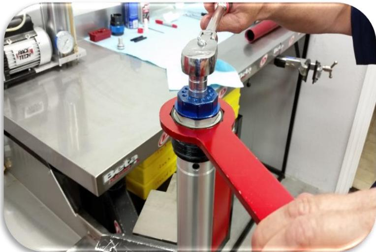
Unthread the compression assembly from the cartridge.
