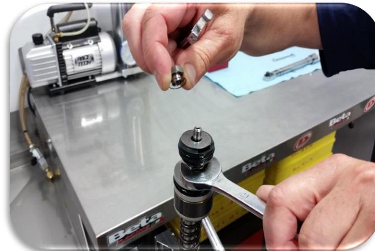
While holding the 17mm hex on the post, loosen and remove the 13mm shoulder nut.
