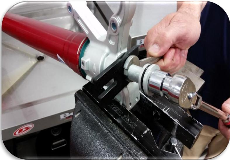
Loosen the 15mm jam nut from the 19mm hex and remove the rebound assembly.
