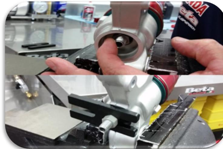
While pushing down on the cartridge, use your index finger to guide the rod through the bottom of the fork leg.
