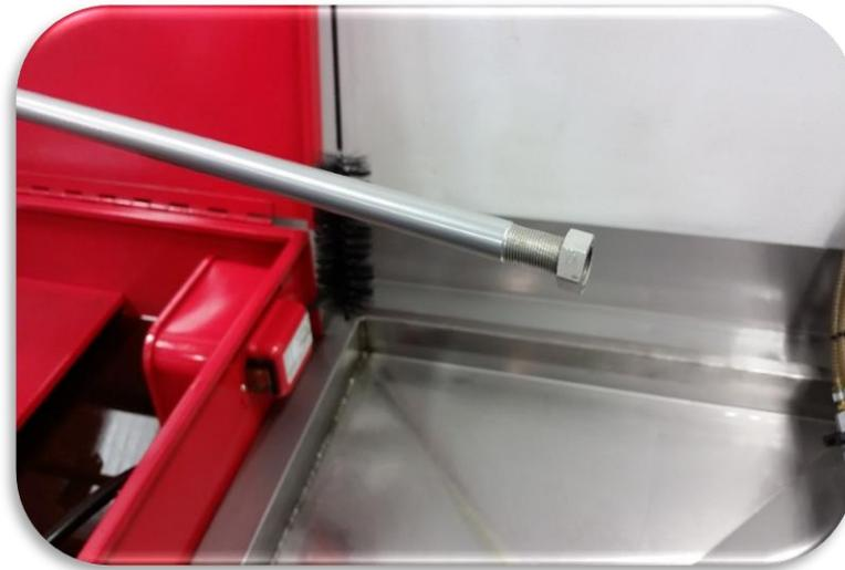
Thread the 15mm nut all the way onto the rod until it stops.
