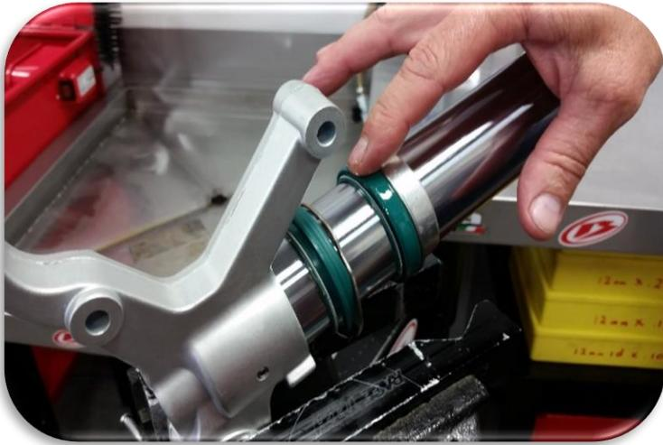
Apply 5w fork oil to the outer edge of the fork seal.
