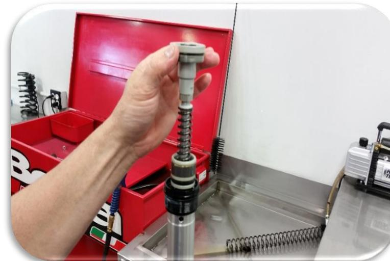
Remove the compression assembly from the cartridge.
