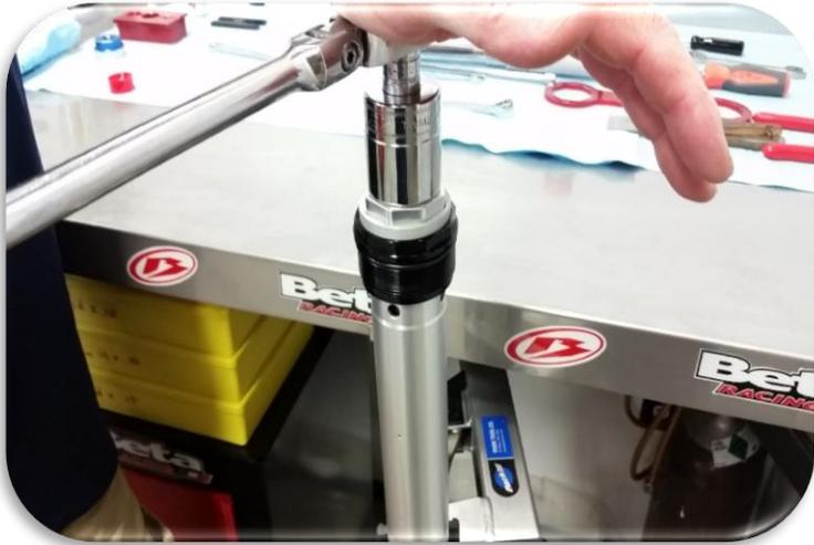
Using the compression assembly holding tool, apply pressure while turning to thread the compression assembly into the cartridge.
