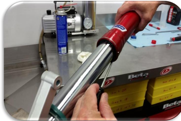
Install the retaining clip making sure it is fully seated into the groove.
