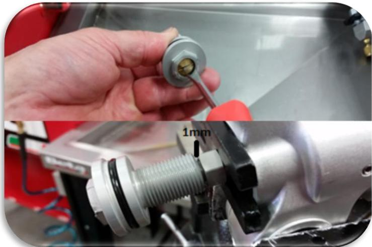
Back the rebound adjuster all the way out (counter clockwise).
