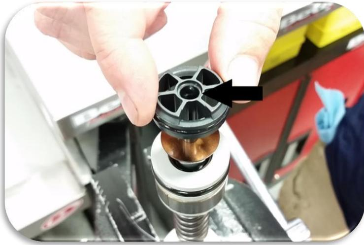
Install the compression piston with the recess facing up.
