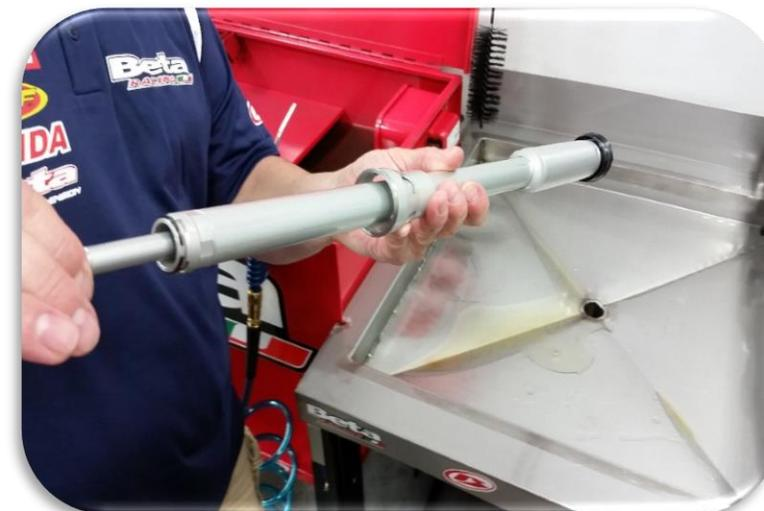
Drain the oil from the cartridge.
