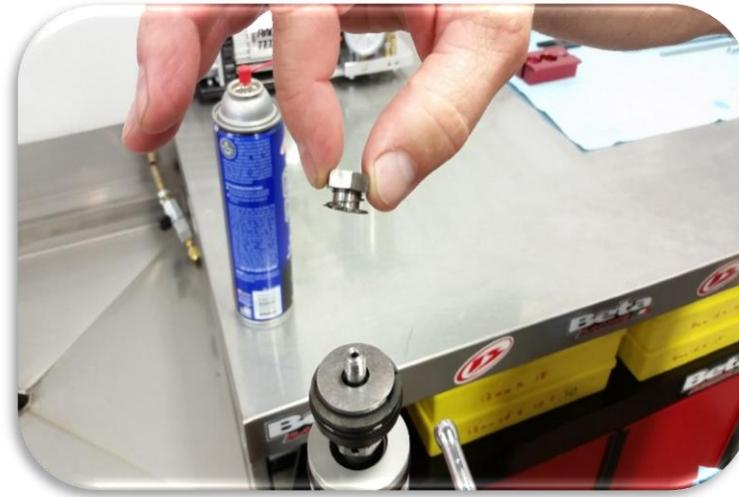
Remove the nut and apply one drop of red loc tight to the threads. Position the spring with the small end against the nut.
