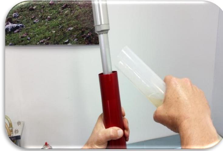
Measure out 350cc's of high quality 5w fork oil and pour it into the outer fork tube.
