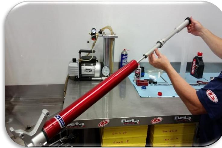
Carefully slide the cartridge assembly into the fork.
