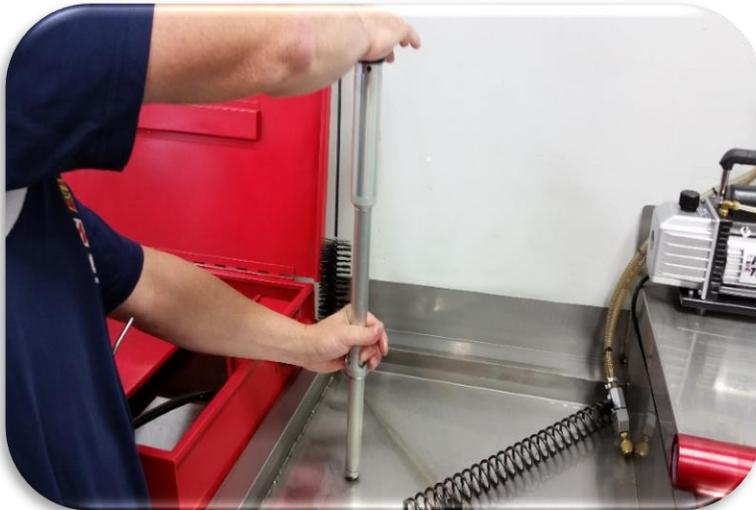
Stroke the dampening rod 2 times making sure it fully extends on its own. If it does not, check for a leaky cartridge seal or damaged floating piston seal.
