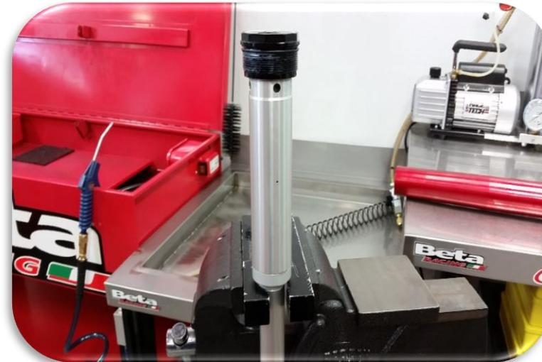
Secure the cartridge in the soft jaw vise.
