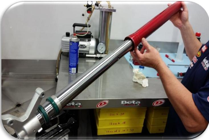
Clean the outer tube and slide it over the lower leg.
