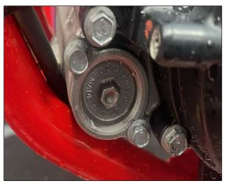
7. Install new oil filter cover o-ring. Re install cap. Tighten to 10 Nm.
