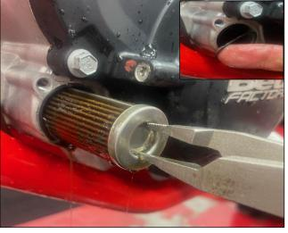
2. Remove both 8mm oil filter cover bolts, have drain pan in place to catch oil drippings.
