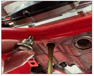
5. Remove transmission oil drain bolt. Allow transmission oil to completely drain into catch pan.
