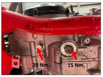
Re install drain bolts tighten engine drain bolt to 15 Nm.
