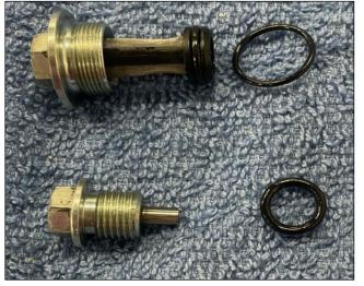
8. Install new o-rings on the transmission and engine oil drain bolts..
