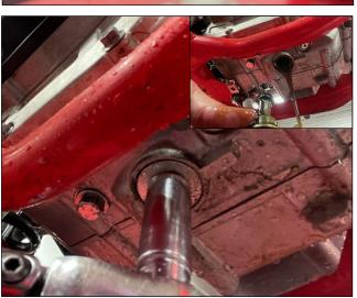
3. Remove oil Filter and the cover oring. Leave uncovered to help with oil drainage.
