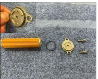
6. Reinstall Oil filter. Make sure the open end of filter is facing toward engine and the solid end is facing the filter cover.
