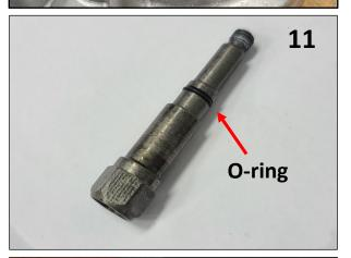
11. Install the new O-ring on the water pump shaft.
