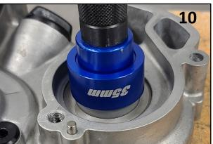
10. Drive the new seal flush with the housing.
