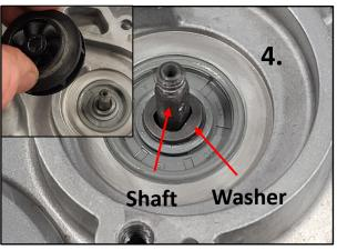
4. Remove the impeller, washer and shaft. The shaft can be removed by pressing the threaded side towards the inside of the clutch cover.
