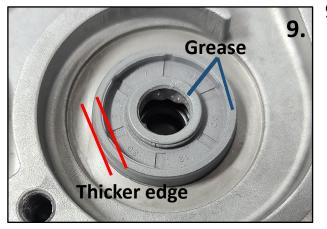
9. Grease the inner and outer lips of the seal.
