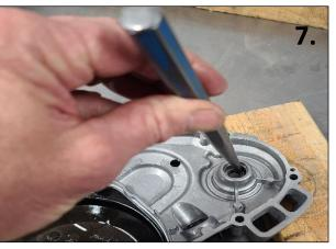
7. Flip the case over then remove the outer bearing using the same method.
