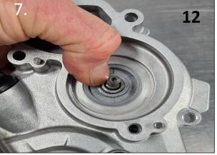
12. Apply grease to the shaft O-ring then fully insert the shaft through the bearings.
