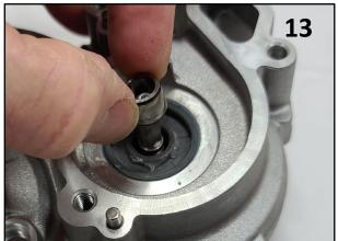
13. Install the shaft bushing pushing it into the grease seal.
