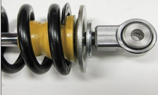
Steel washer fitment sequence:
