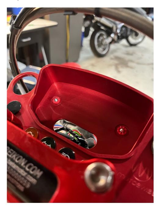
11. Pass the Voyager wires through the cable recess in the floor of the Dash making sure the temperature sensor also comes through. Make sure the MicroSD Card slot cover is seated properly and drop the Voyager into place. You will have to tip the Voyager slightly to the right to allow the slot cover rubber to slip into the recess in the housing. Reconnect the Voyager cables.
