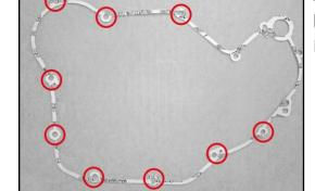
4.Remove the 9 inner clutch cover bolts at the locations seen in the photo. Remove the inner clutch cover.
