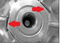
16. Using channel lock pliers, fold the locking tabs over against the nut.
