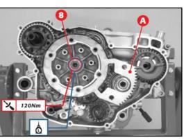
15. Make sure the needle bearing is lubricated then install the new clutch basket, spacer, inner hub and new tab washer.
