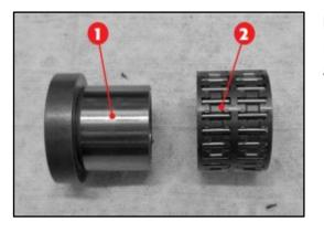
**Note:** Replace the clutch basket bushing and needle bearing if traces of meshing or abnormal wear are detected.
