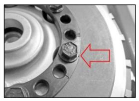
**Note:** The preload ring has three settings... III is the stock X trainer position and has the lightest lever pull and engagement.
