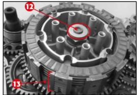
6. Remove the thrust bearing (fig12) along with all the clutch plates fig13.
