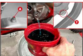
Remove the lower water pump bolt and washer to drain the coolant fig7.
