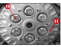
5. Remove the six bolts (fig10) holding the pressure plate (fig11) to the inner hub along with the washers and springs.
