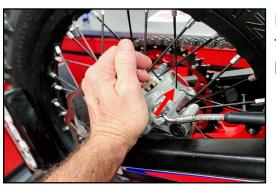
Note: Pressing on the rear brake caliper will allow the rear brake pedal to move to its lowest position making the clutch cover removal easier.
