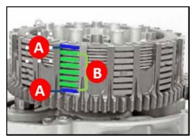
17. Soak the new fiber clutch plates in gear oil for at least 5 minutes.
