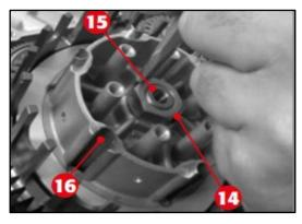
7. Use a hammer and chisel to bend the locking tabs (fig14) away from the clutch nut fig15.
