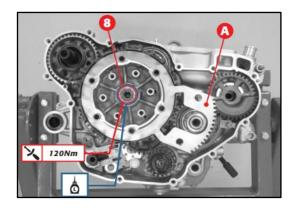
15. Make sure the needle bearing is lubricated then install the new clutch basket, spacer, inner hub (stock) and new tab washer.
