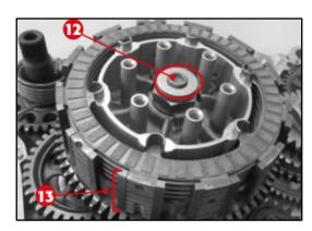
6. Remove the thrust bearing (fig12) along with all the clutch plates fig13.
