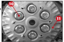
5. Remove the six bolts (fig10) holding the pressure plate (fig11) to the inner hub along with the washers and springs.
