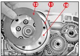
18. Reinstall the thrust bearing on to the transmission shaft. (not shown) Install the pressure plate (fig 10), the steel ring (fig 11) and the conical washer fig12.
