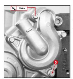
22. Install the water pump cover and 4 bolts making sure the copper washer is under the bottom bolt fig3. Torque all 13 clutch cover and water pump bolts to 10Nm in a criss cross pattern.
