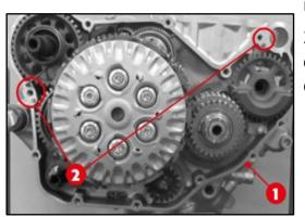
19. Start the first bolt in the desired preload ring position then add the other 5 bolts.
