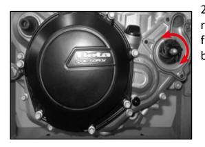
21. Install the clutch cover on center case rotating the impeller until the cover sits flush on the case. Install the 9 inner cover bolts leaving them loose.
