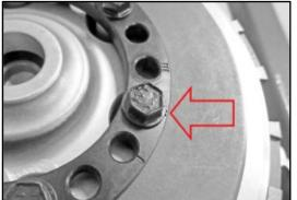
**Note:** The preload ring has three settings... III is the stock X trainer position and has the lightest lever pull and engagement.
