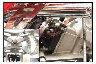
4. Lightly <u>pry</u> the oil line from the barbed fitting on the intake manifold. (Do not pull on the line or it can pull the barb from the manifold.)
