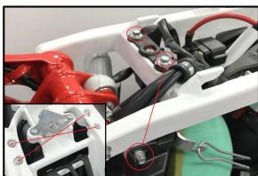
5. Remove the oil tank then reinstall the top of the sub-frame to the air box and supports using the bolts that were removed.
