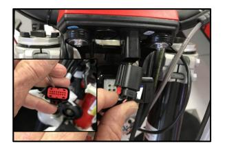
13. locate the black plug on the meter and unplug it by first sliding the red tab out then pull on the plug.
