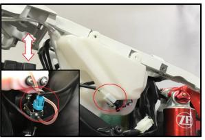
3a. Unplug the low oil sending unit and oil pump plugs from the harness.
