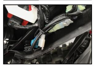
6. Relocate the oil tank and pump plugs and secure them with zip ties.
