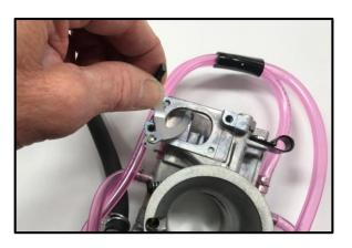
10. Remove the TPS actuator rod.
