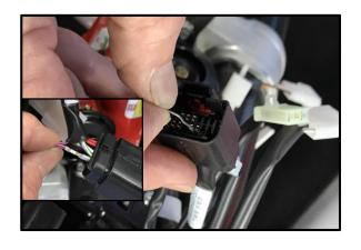
14. Locate the pink wire with a purple stripe. This wire must be unplugged or the engine warning light will stay on.
