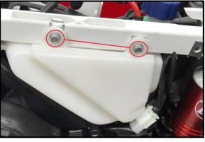
3. Remove the 2 oil tank bolts then lift the white plastic part of the subframe upwards.
