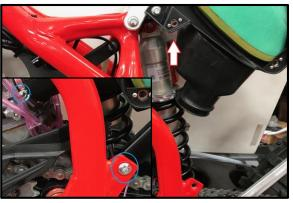
7. Loosen the hose clamp on the back of the carburetor then remove the 2 lower subframe bolts. Lift on the subframe assembly while rotating it up. Remove the hose clamp as soon as the boot pulls away from the carburetor as it will not want to pass the shock spring.
