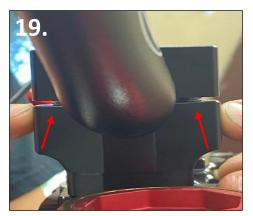
19. Re install handlebars, install top bar clamp with bolts finger tight so you can make necessary adjustments to bar position. Once you have them in desired position tighten top bolts. **IMPORTANT** be sure to evenly tighten top clamp bolts so you have an even distance on each side, see photo.
