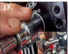
17. Now torque steering stem nut to 40nm. Rotate Steering to get bearings properly set. Once that is completed loosen steering stem nut and re torque to 30nm. Next you will tighten the steering stem pinch bolt to 20nm.
