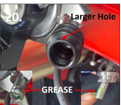
20. Next grease frame clamp and rod on stabilizer. Install rubber dust cover onto frame clamp, make sure larger hole is facing up. Install the stabilizer rod into frame clamp.
