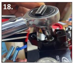
18. Begin installing Beta bar mounts Remove top clamp from bar mounts, apply blue Loctite to the handlebar clamp bolts then put clamp in position the kit is meant for and torque to 40nm.
