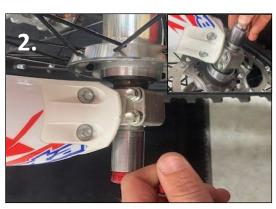
2. Next you will remove front wheel from the bike. Loosen axle nut & pinch bolts. Then remove axle
