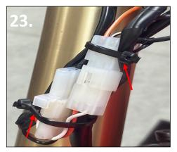
23. Re apply rubber handlebar straps for wiring then twist up the wires behind headlight mask and zip tie to keep from tangling.
