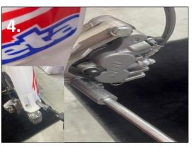
4. Remove front brake caliper assembly from fork and left fork guard and remove the brake line from the guide
