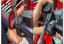
9. Loosen pinch all 8 pinch bolts **IMPORTANT:** hold fork with knee while loosening pinch bolts to prevent it from falling out and contacting the ground. Now remove steering stem bolt.
