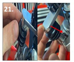
21. When mounting stabilizer to handlebar compress the stabilizer as low as it will go. Install front clamp for stabilizer while making sure it is centered between both bar mounts. Turn bars back and forth to check for steering fluidity
