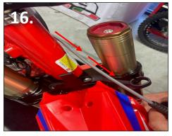
16. Line up triple clamp as you reinstall the right fork. Once the fork is in place tighten upper pinch bolt to 17nm and bottom pinch bolt to 12nm. For the left fork make sure the clutch line is in position while re installing the fork. Tighten pinch bolts to same specs as the right side, upper pinch bolt to 17nm and bottom pinch bolt to 12nm. **IMPORTANT** Please double check these bolts are properly tightened 2-3 times.
