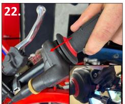
22. Install Throttle housing, front brake line assembly for this step be sure to have the brake line in the guide, mount clutch M/C to handlebar. Re connect kill & start buttons.
