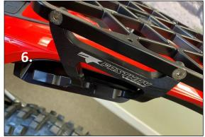
6. Place Plate on top on brackets and align the holes on either side. Fasten using the countersunk allen head bolts provided!
