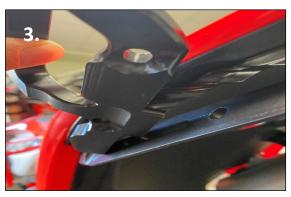
3. Take the plate holders and install into the machined groove in the underside brackets.
