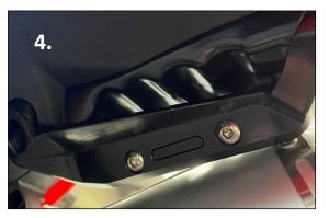
4. Fasten the two bolts on either side. Use the button head bolts provided!
