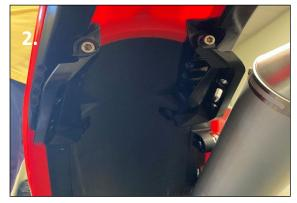
2. Install The underside brackets as shown in photo 2. Use bolts included with kit.
