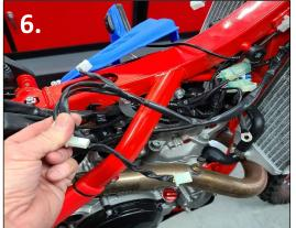
6. Unlatch the plastic harness holder and cut the zip ties to allow the rear section of the front harness to be pulled forward. You will need to unplug the rear harness and rear brake switch.
