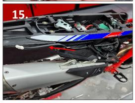
12. Run the long thin tail light lead to the rear right side of the subframe strut, same as the stock harness position.
