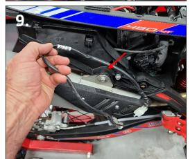
9. Unplug the rear brake light and remove the rear harness.
