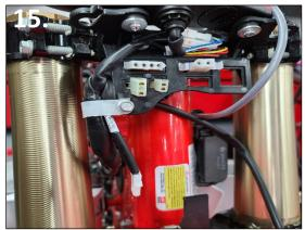
15. Run the harness forward to the speedometer bracket and insert the kill/light switch, front brake light and start plugs into the speedometer bracket. Attach the harness to the bracket using the stock holder and bolt. Leave the map switch plug running back down the main loom and under the holder.
