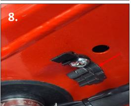
8. Unlatch the large plastic harness holder then remove the front harness.
