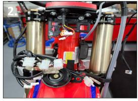
1. Remove Headlight mask, seat, fuel tank and rear fender.
