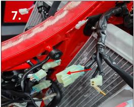
7. Push the locking tab then remove the 6 pin plug from the connector bracket. Then unplug the connector along with the yellow/red map switch wire and map switch plug.
