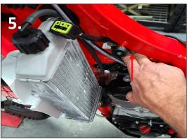
5. Unplug the regulator then push the connector bracket through the frame to access the plugs.
