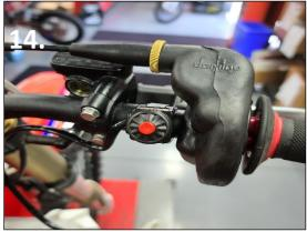
14. Install the new start switch next to the throttle grip.
