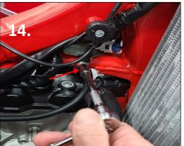
11. Reconnect the yellow/red map switch circuit wire then push the connector back into the frame. Connect the ground to the bracket bolt and torque to 10Nm.
