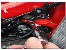
4. Remove the bolt holding the connector bracket in the frame center
