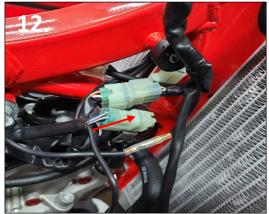
10. Connect the 6 pin plug from the new harness into the plug of the main harness. Re insert the plug onto the connector bracket.
