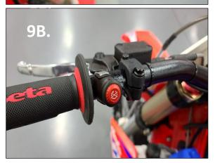
Install the new start (9A) and kill (9B) switches on the handles bars.
