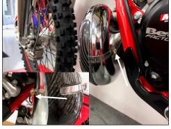
4. Place carbon guard onto pipe & tighten the clamps until snug. As both band clamps are tightened & mark clamp a half inch from screw and cut it off.
