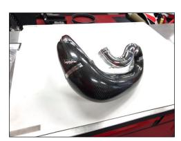
2. In determining band clamp positioning, ensure there's access to the screw adjusters for ease of assembly & disassembly.
