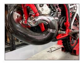
5. Once you're satisfied with the guard placement & clamp position, snug the band clamps securely but don't overtighten them.
