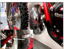
3. Route the band clamps through the carbon guard slots.
