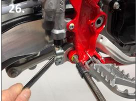
26. Install the brake pedal bolt and nut applying high strength Loctite to the threads. Re install brake pedal spring.
