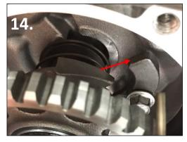
14. Install the kickstart assembly into the housing with the splined side facing outwards. Make sure the ramp is positioned straight up so once it is installed it will go behind the ramp on the case.
