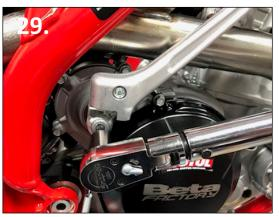
Install the kickstart lever. Install the washer and bolt using medium strength Loctite on the threads. Torque bolt to 25nm
