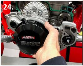
23. Clean the gasket area surfaces of the case and inner clutch cover. Install the gasket and the clutch cover assembly.
