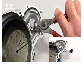
22. Remove the snap ring from the plug in the inner clutch cover then push the plug out, this is where the kick starter shaft will come through. Install the kickstart shaft seal.
