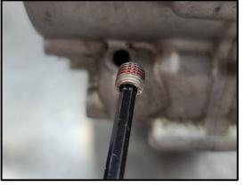
4. Apply the supplied thread locking sealant to the threads of the supplied tapered 8x1.0 set screw.
