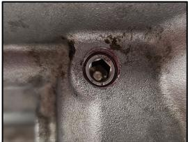
5. Thread the set screw in until it is fully seated and tight.
