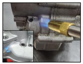
1. Apply heat to the area around the screw.
