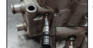
2. Use a hand impact driver to loosen and removed the leaking set screw.
