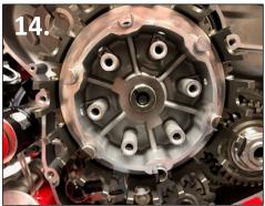
13.Install the large washer and the inner hub with the 6 sliding pins.
