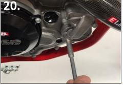
20.Install the water pump cover and the 3 bolts making sure the copper washer is on the bottom bolt. Tighten all bolts in a crisscross pattern to 10 Nm.
