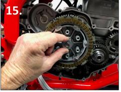
15. Re install the clutch plates noting the fiber plates with the blue mark go on the furthest out positions and the green marked plates going on the inside. The smooth or curved side of the plates will all be facing the engine.
