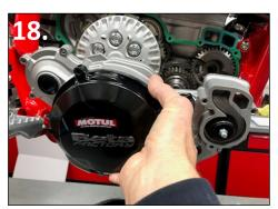
18.Clean the gasket area surfaces of the case and inner clutch cover. Install the gasket and the clutch cover assembly.
