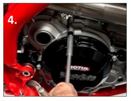
Remove the top 3 outer clutch cover bolts then remove the inner 8 clutch cover bolts. Remove clutch cover assembly.
