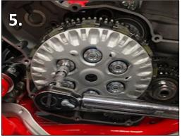
5. Remove the 6 clutch bolts, washer, springs, and the pressure plate.
