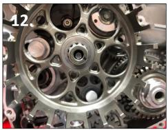
12.Re install the clutch basket. You will have to rotate the oil pump gears to get them aligned with the clutch basket. If you do not do this key step you may damage the oil pump gears
