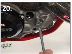
19. Insert the 3 bolts into the outer clutch cover and the 8 bolts on the inner cover leaving them loose.
