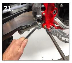
21.Install the brake pedal bolt and nut applying high strength Loctite to the threads.
