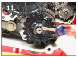
11.Use a small flat blade screw driver to lightly pry the E clip from the shaft holding the small oil pump gear. Apply Pressure to the clip with your finger to make sure it doesn't fly away. Remove the small gear and install the new steel gear. Reinstall the E clip making sure it is fully seated.
