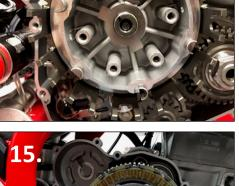
14.Install the new safety washer and lock nut. Apply medium strength Loctite to nut and with the holding tool in place torque the nut to 120 Nm. Then fold the tabs on the safety washer over the lock nut.
