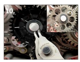
10. Remove the snap ring and thrust washer from the large oil pump gear. Remove the gear and install the new steel gear. Re install the thrust washer and snap ring making sure it Is fully seated.
