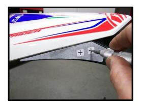
1) Hold the template provided to the mid fender to mark your holes with a sharp pic or other pointed device. Flip the template over and mark the other side of the fender. It is very important that the holes are drilled equal on each side to insure the turn signals will be mounted level.
