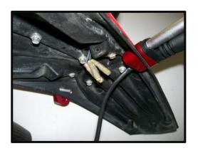
3) Insert the wire through the inner wedge on the inside of the fender and install the turn signal by threading the supplied 6mm bolt into the inner wedge. Repeat this step for the other side. Connect the turn signal wires to their correct side.
