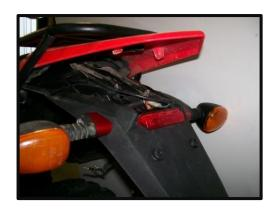
4) After both wedges have been installed, reinstall the rear mid fender making sure that no wires are in the way of the screws holding the mid fender to the rear fender.
