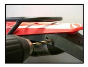
2) Drill the two holes on each side with a 1/4" drill bit.
