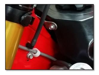
Step 7: Install the left side fuel hose to the carburetor. Route the fuel hose from the right side over the top engine support (head stay) and connect the quick release connector. Make sure the fuel hose is free of the cylinder or any sharp objects.
