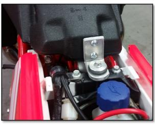
Step 6: Install the two 6x12 flange bolts to the front mount and tighten.
