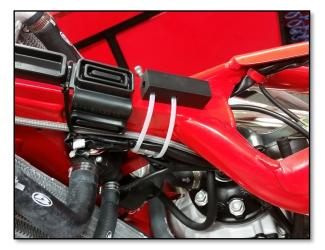
Step 4: Install the two L brackets into the existing lower radiator shroud mounting spot using the aluminum spacer and the 6x25 button head allen bolts as shown. Install the tank onto the motorcycle and install the L bracket to the fuel tank using the 6x12 flange bolts.
