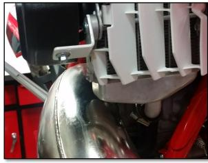
Step 5: Install the rear mount to the tank using the two 6x16 button head allen bolts. Install the rear mount to the subframe using the stock mounting spacer and rubber cushion.
