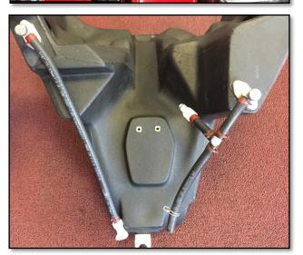
Step 3: Install the square support block to the frame as shown in the photo with the two zip ties.
