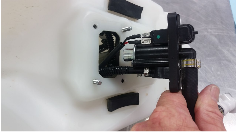
Unbolt and remove the rear fuel pump
