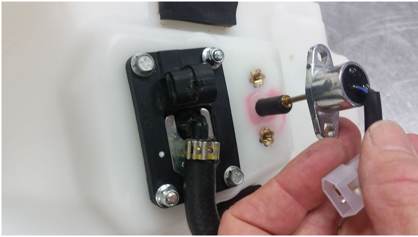
Unbolt and remove the Fuel Level Sensor.
