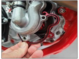
5. Slide the spacer behind the water pump cover with the rubber gasket facing outwards.
