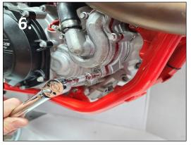
6. Install the new longer water pump cover bolts making sure the copper washer is on the bottom bolt. Torque to 10nm.
