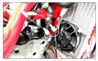
The Beta Manual Radiator Fan Kit allows for manual switching On & Off of the radiator cooling fan, useful when expecting hotter than normal riding &/or engine temps. The manual fan switch enables manual activation of the fan, but it won't override (manually turn off) the cooling fan's normal automatic cooling cycles that are triggered @ 219-221° F operating temp.
