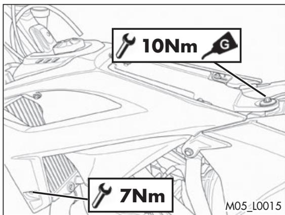
Push the tank towards the front of the vehicle and down.
