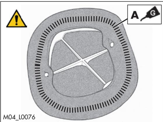
Note: before refitting the filter to the vehicle is recommended to apply a long-term grease in the area **A**.
