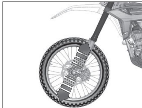
Tighten the wheel bolt and the screws of the foot-legs.
