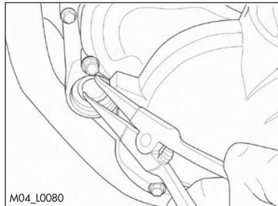
Mount the new paper filter, close the oil tap to engine, tighten the screws at 10 Nm.
