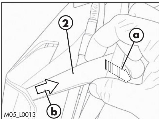
Remove the jumper **2** by pulling the rear portion towards you and slide it towards the rear.
