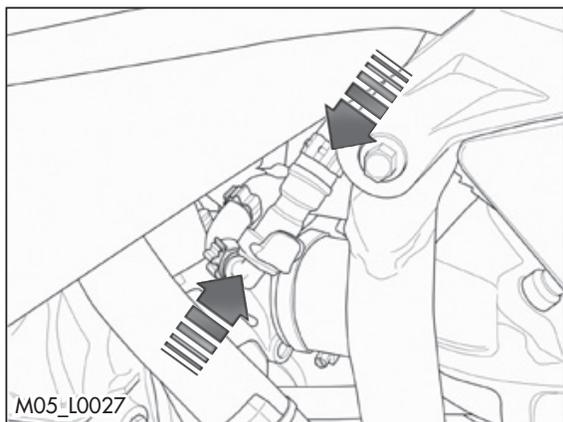
Connect the fuel connections by coupling them completely.
