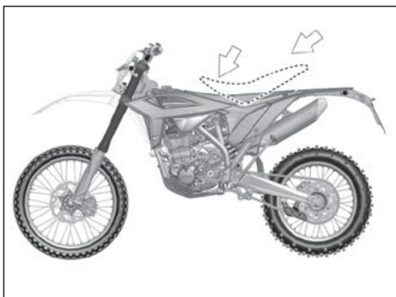
Press the saddle down in the middle and at the same time, push it forwards until the bayonet joint engages in its seat.
