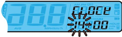
Press the to enter the **Adjust button** minute setting.
