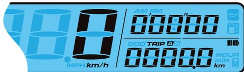
Press the **Select button** to switch from Stopwatch to Speed Record.
