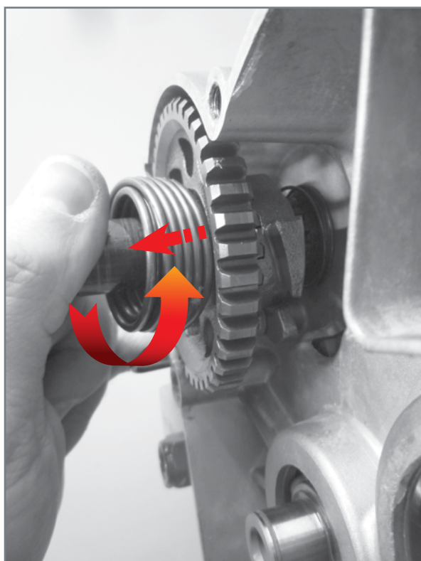
Extraction of shaft from crankcase.
