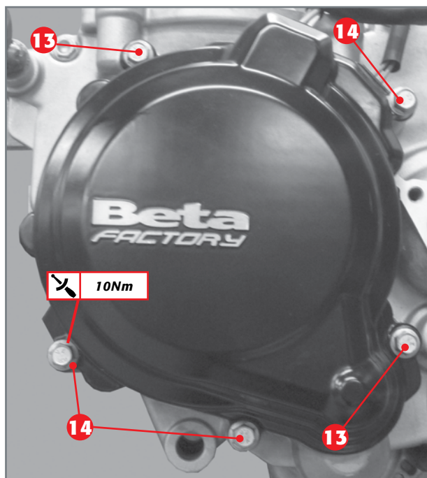
Flywheel cover coupled to crankcase.
