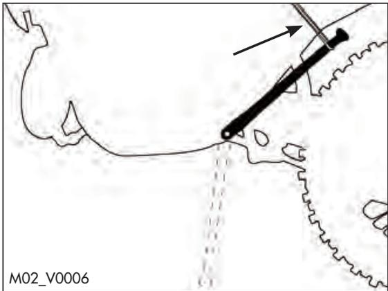
If the vehicle is used off-road, the closed stand can be further fastened by means of rubber band.
