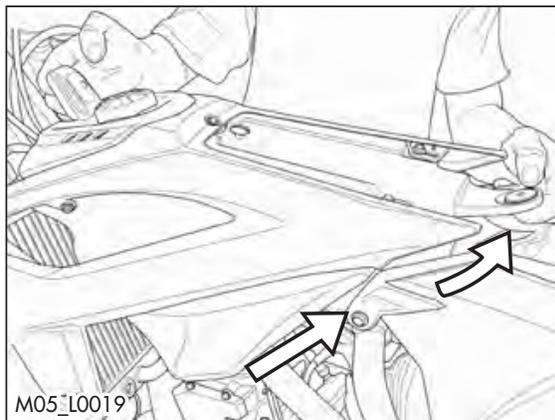
Lift the tank backwards and remove the tank towards the rear.
