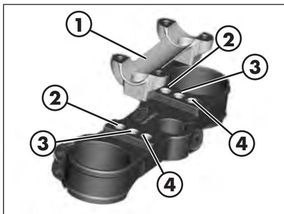
To adjust the position of the u-bolt remove the screws shown in the figure.
