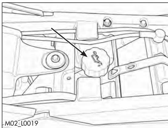
To open the fuel tank cap turn it anticlockwise.
