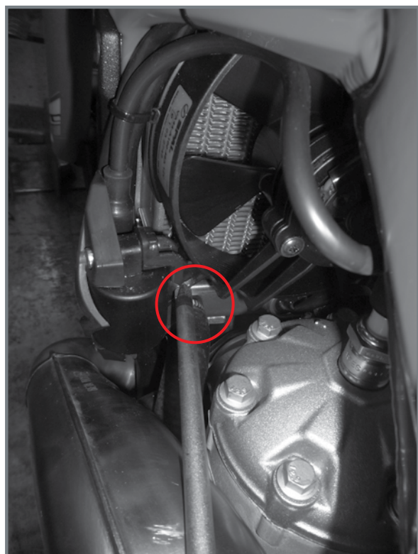
Reassembling the coil and support.
