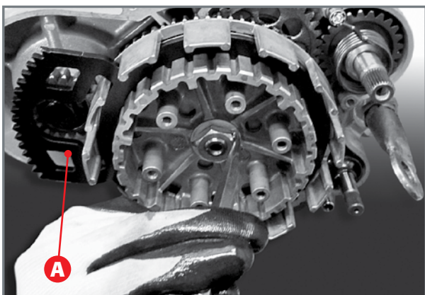
Opening the flaps of the safety washer.
