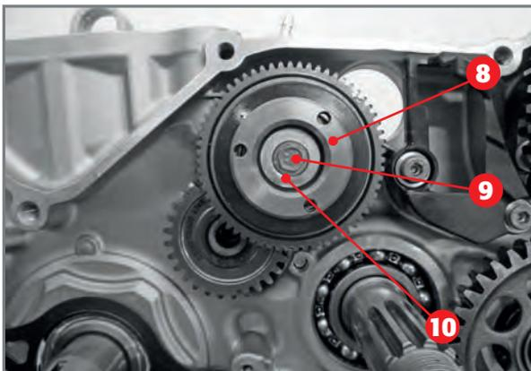
*Torque limiter 8, screw 7 and washer 9.*
