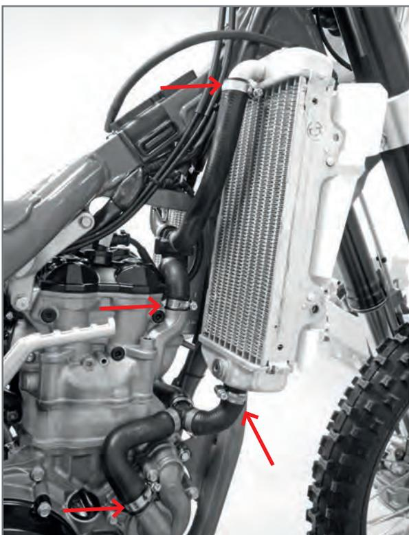
Connect the radiators to the engine.
