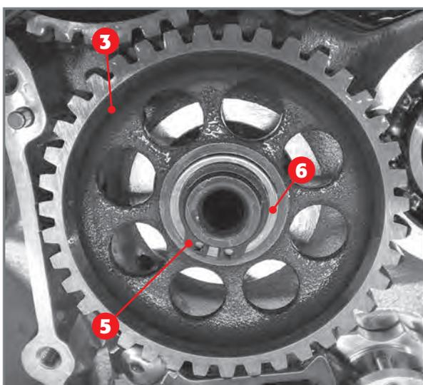
*Removal of circlip 5 of idler gear 3.*
