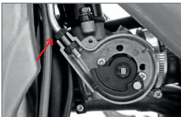
Loosen the adjustment nuts and release the gas cables.
