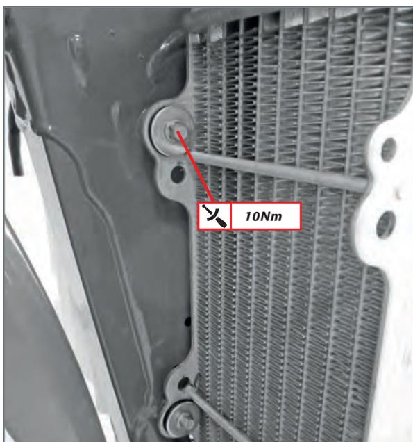
Apply the screws and fasten at 10Nm.
