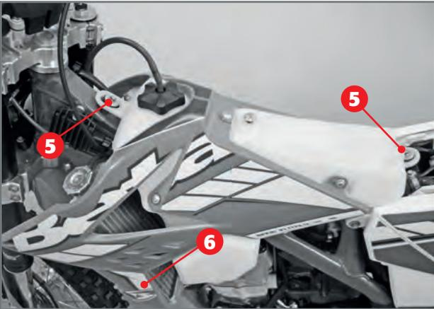
To dismount the tank, remove the seat, completely loosen the two screws **5** fixing the tank to the frame and screw **6** (one per side) which fixes the side to the radiator.
