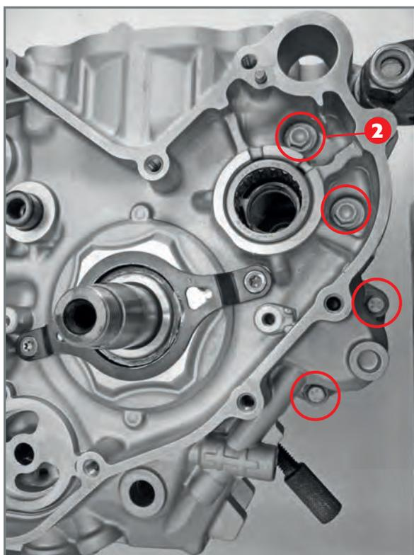
*Screws 2 for blocking right side casing.*
