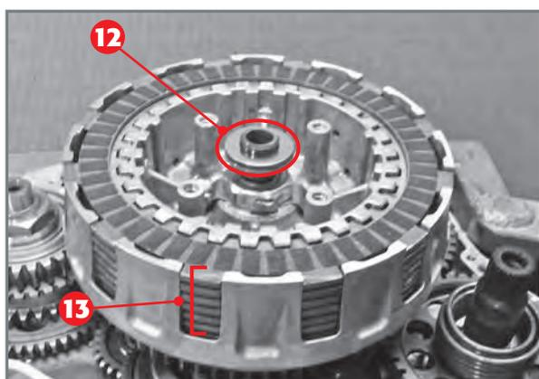
*Pressure plate unit 12 and clutch disc pack 13.*
