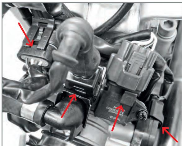
Connect the electric connectors indicated in the figure, relative to the throttle body.
