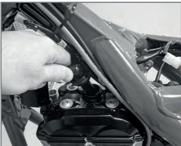
Disconnect the spark plug cap.
