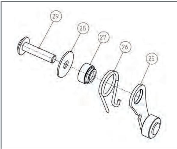
Keeping the tightener on the lever **25** facing towards the crankcase half, apply the spacer **27** onto it, by inserting the smaller diameter segment in the lever. Apply the spring **26** so that the hook inserts into the groove present on the lever **25** and then apply the washer **28** and the screw **29** M6x20 whose threading must be spread with medium strength threadlocker.
