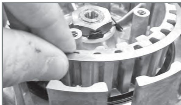
*Removal of disc spring assembly.*
