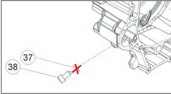
To block the crankshaft, apply only the screw 38 to the crankcase.
