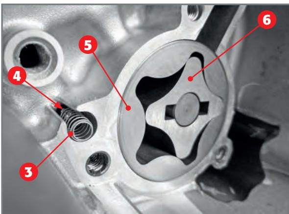
*Low-pressure oil pump and by-pass valve.*
