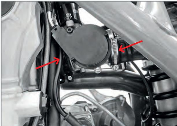
Loosen the throttle body straps from the air filter sleeve and from the manifold.
