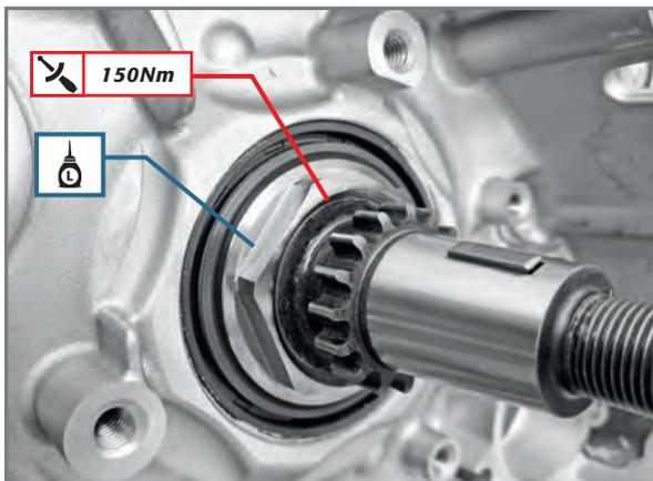
Nut on left side of crankshaft.
