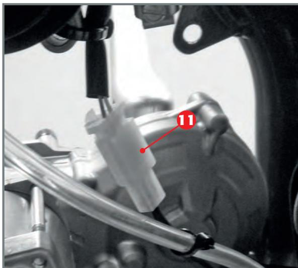
Disconnect the rear brake stop connector **11**.
