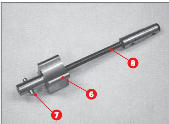
*Internal rotor 6, roller 7 and drive shaft 8.*
