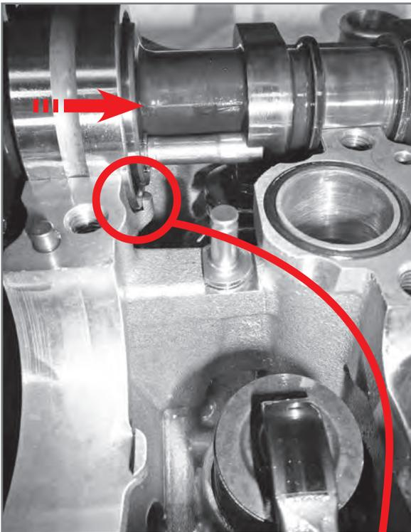
*Positioning camshaft bearing.*
