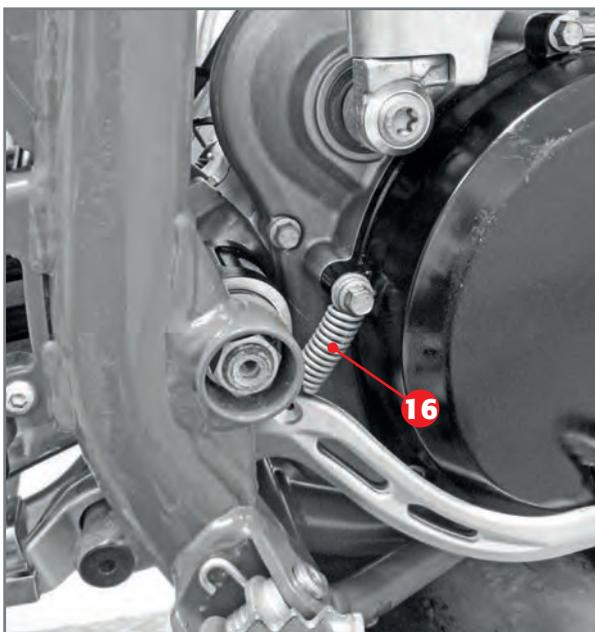
Release and remove the brake pedal return spring **16**.
