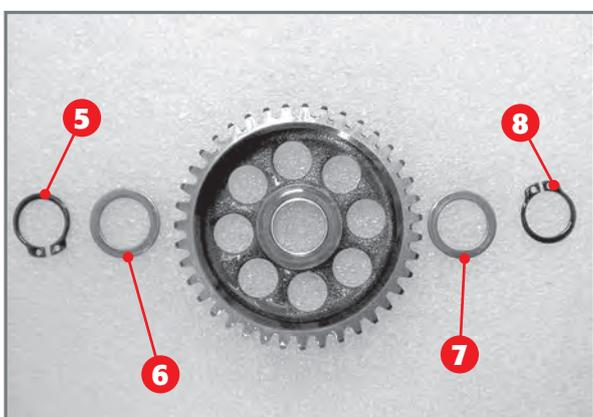
*Two circlips 5 and 8 and thrust washers 6 and 7.*
