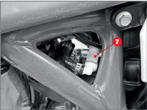
Disconnect the petrol pipe by pressing the relevant button of quick coupling **7**.
