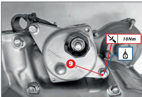
*The two fixing screws 9 of the start motor.*
