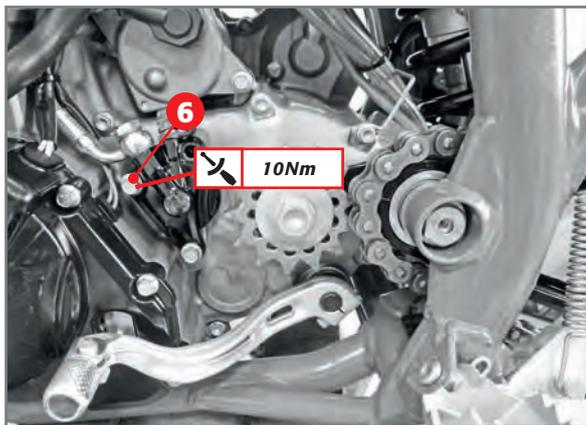
Apply the unit clutch actuator to the two fixing screws **6**.
