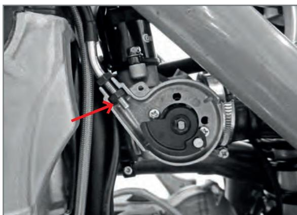
Set the gas cable on the left side of the frame and make it pass outside the head connection. Apply the gas cables to the throttle body and tighten the nuts.
