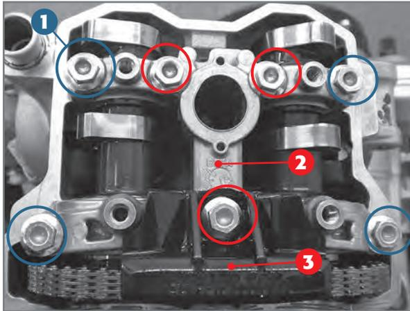
Fixing screws 1 camshaft support 2 and chain guide 3
