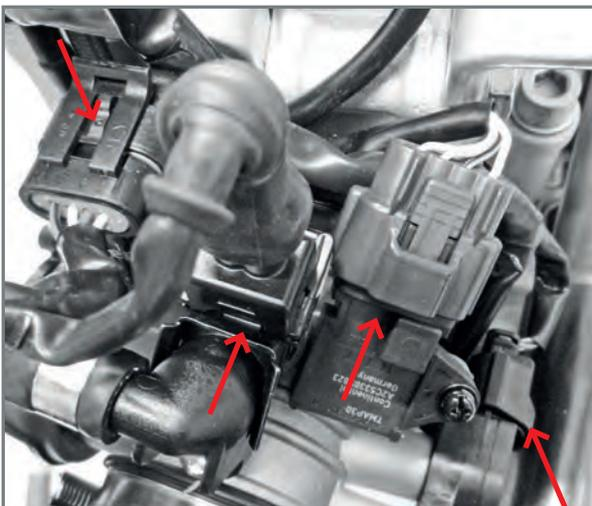
Disconnect the electric connectors indicated in the figure, relative to the throttle body.
