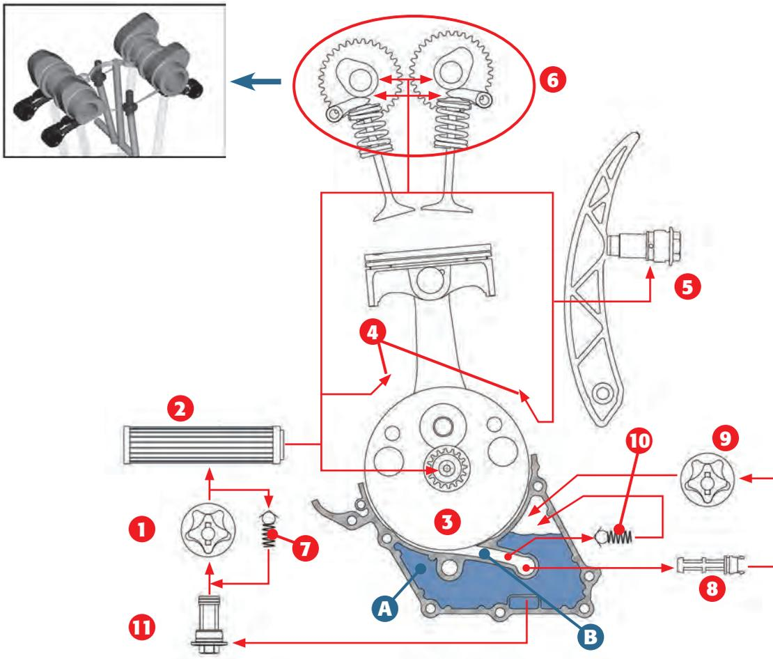
\* Part of the lubricant sent to the cylinder head is used for the hydrodynamic support of the camshafts.
