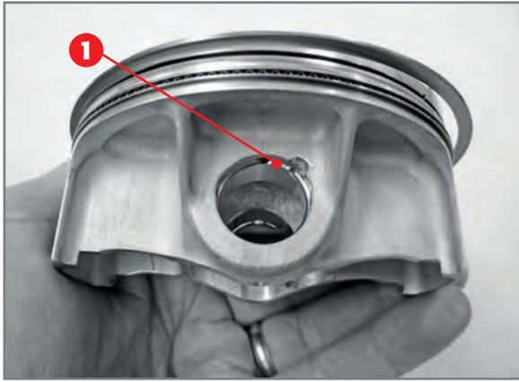
*Application of circlip 1 to piston.*
