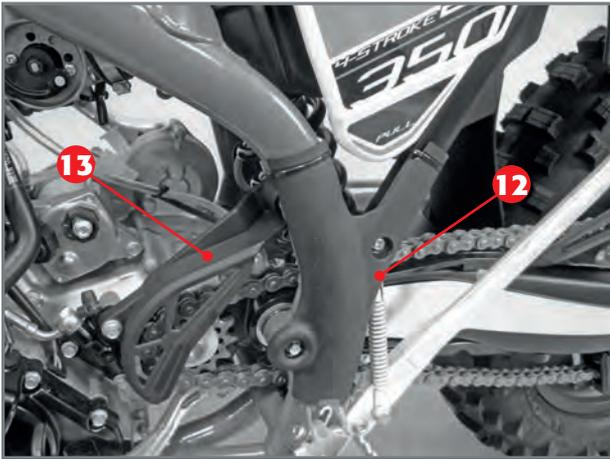
Remove the frame guards **12** (one each side) and the pinion guard **13**.
