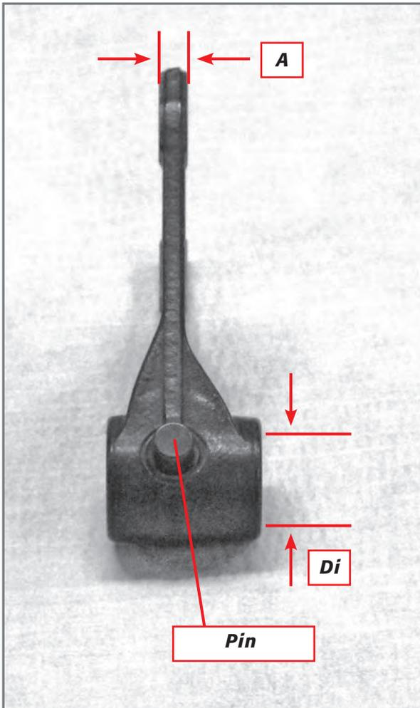
Make sure the distance **A** between the outer faces of the fork is not less than that indicated below:
