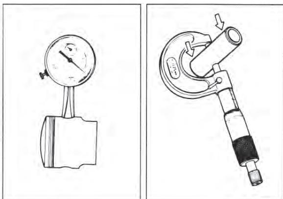
Measuring pin bolt seat and pin bolt.
