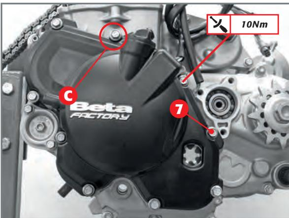
Grease the oil seals on the cover of the flywheel and secure it on the left guard using the nine **7** M6x25 screws.
