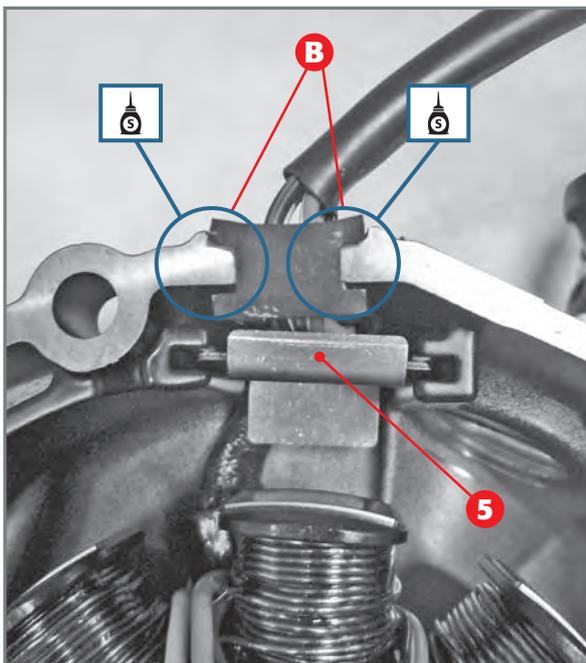
**Application of cable protection plate 5. Note the two zones B where a drop of gasket paste must be applied.**
