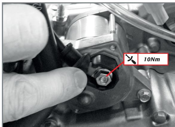
Apply the start motor cable and fasten the nut at 10Nm. Cover the connection using the specific protective cap.
