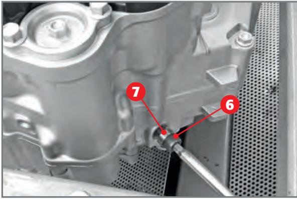
The crankshaft blocking screw 6 with copper washer 7.
