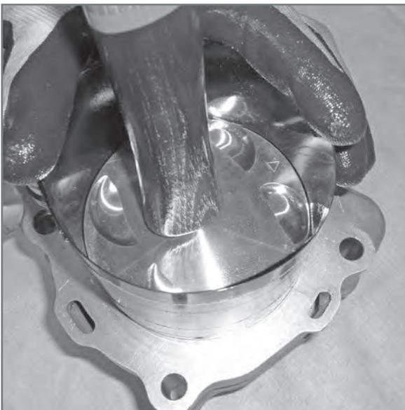
**Insertion of piston in cylinder.**
