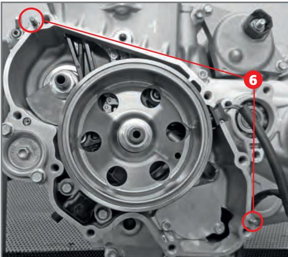
Insert the centring pins **6** on the crankcase and fasten a new gasket.
