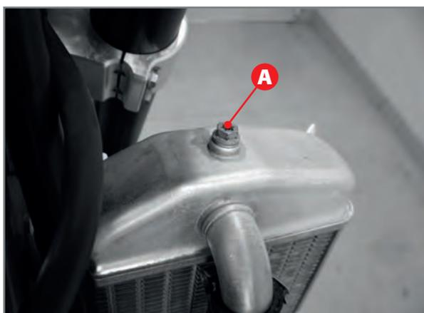
Apply the loading cap and fasten the bleed screw at 10Nm.
