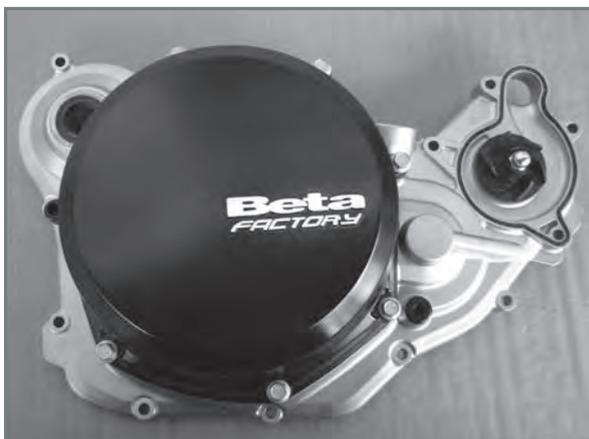
*Complete internal clutch cove of water pump.*
