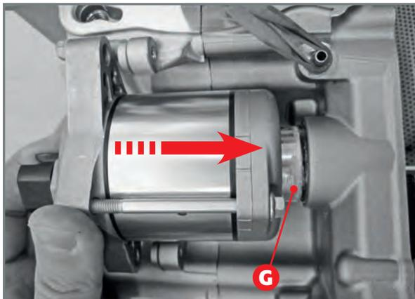
*Insertion of start motor in crankcase half.
