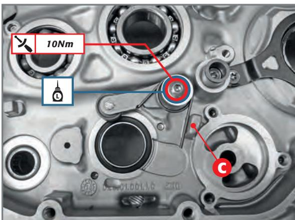
Apply the entire device on the crankcase half so that the straight segment of the spring rests on the stop **C**. Tighten the screw at 10Nm.
