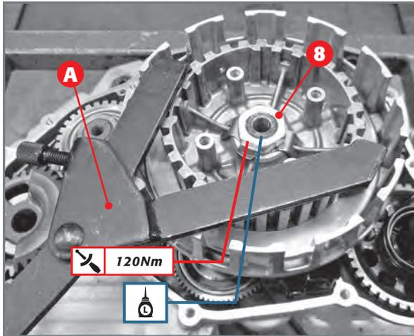
**Blocking inner hub with specific tool Code 0061400400.**
