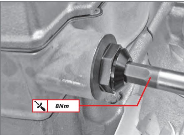
Insert the spring in the support and apply the cap to be tightened at a torque of 8Nm.
