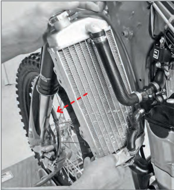
Remove the left radiator with pipes.
