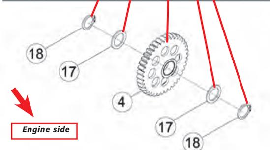
*Kickstart device unit coupled to the crankcase.*
