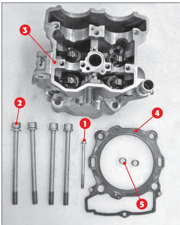
Remove the head gasket **4** and the two centring bushes **5**.
