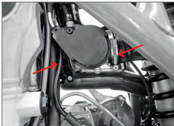
Make sure the filter box sleeve is correctly inserted inside the throttle body, fasten the two filter box side and manifold side straps.
