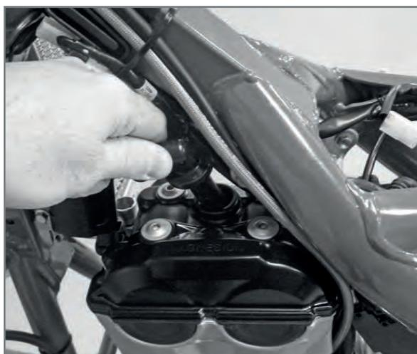
Apply the spark plug cap.
