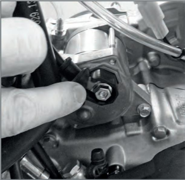
Remove the start motor cable fixing nut.
