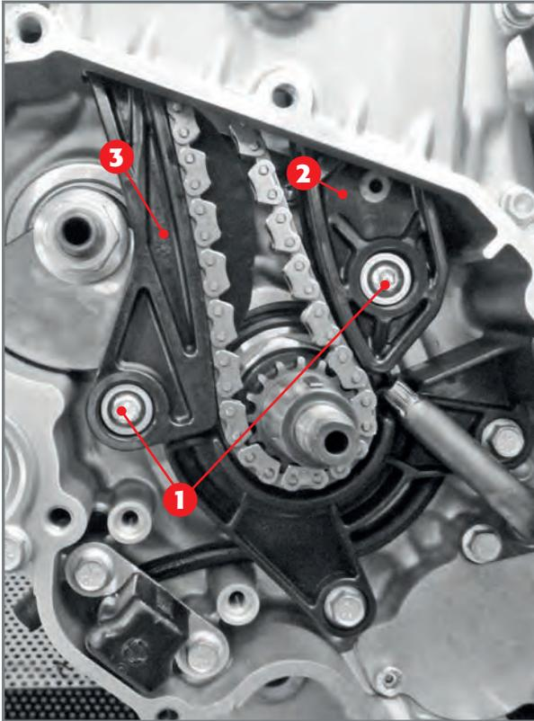
*Fixing screws 1 of mobile 2 and fixed pad 3.*
