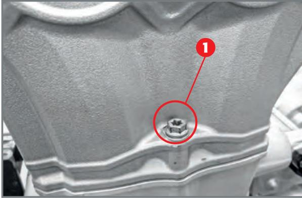
*Chain-side head fixing screw.*
