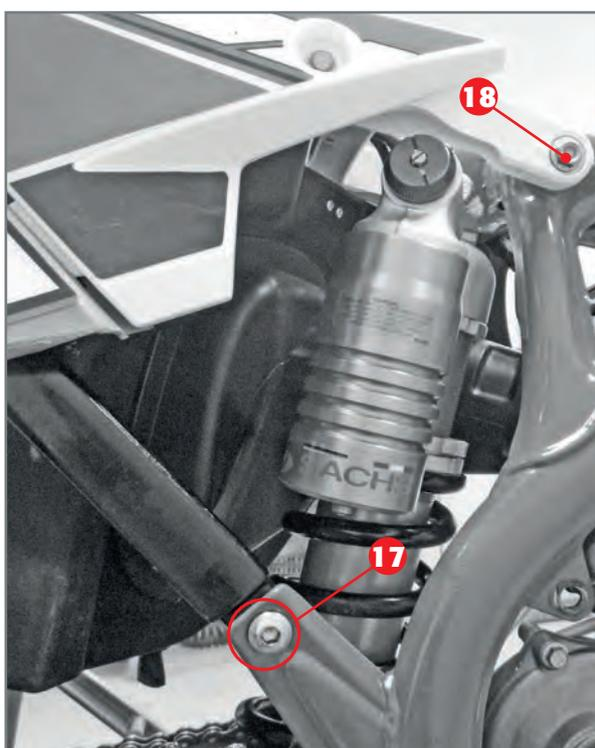
Remove the seat rail lower fixing screws **17** (one each side) and loosen the upper screws **18** (one each side).
