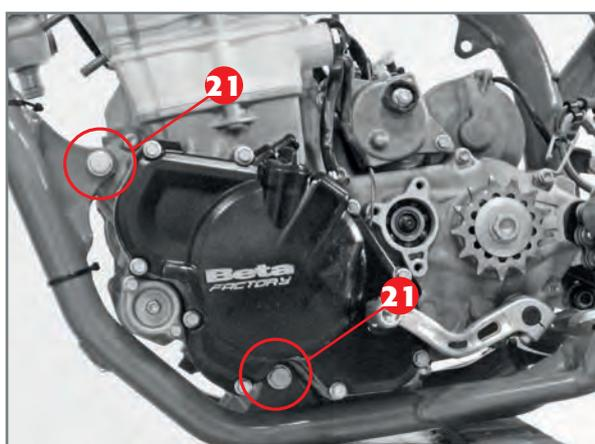
Remove the engine pins **21**.
