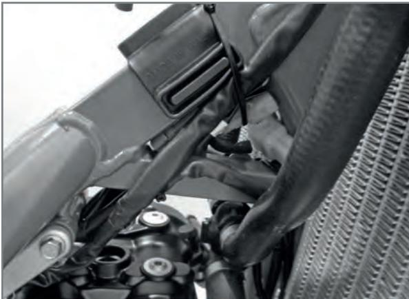
*Electric connectors in the recess (injection versions).*
