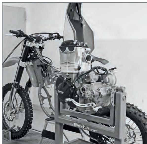
Extract the engine from the frame and apply it to the specific stand code 3625132 000 using specific front fixing bracket code 006140140 000.
