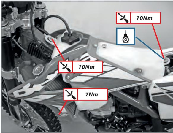
Grease the rear fastener and tighten the screws at the indicated torque values.
