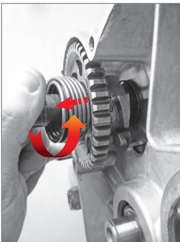
Extraction of shaft from crankcase.
