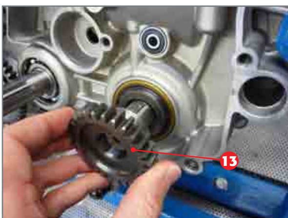
Removal of main gear.
