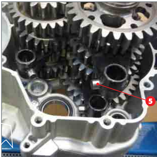
Extraction of forks from gearbox unit.
