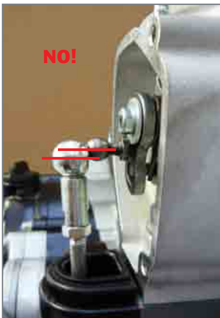
Incorrect positions of the control rod seat.
