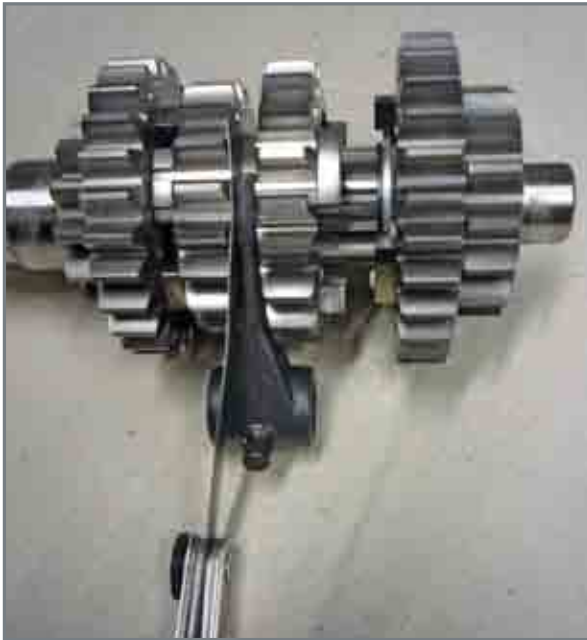
Check of wear of forks and gearwheels.
