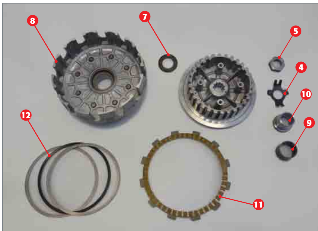
Safety washer 4 ; nut 5 ; washer 7 ; case 8 ; roller cage 9 ; centre bearing 10 ; special driven disc 11 ; disc spring assembly 12 .
