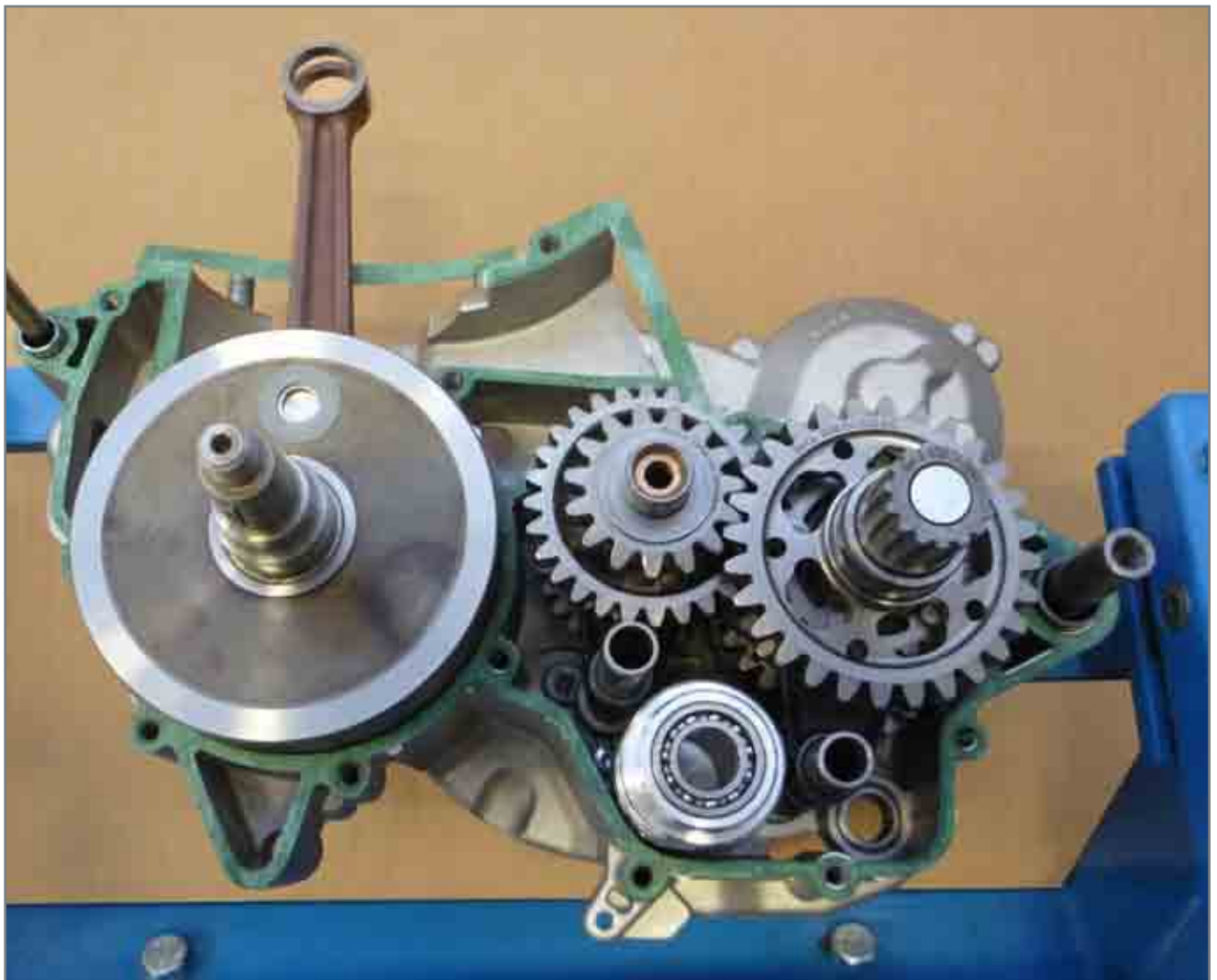
View inside the right crankcase with crankshaft, gearbox shafts complete with wheels, internal gearshift and gasket.
