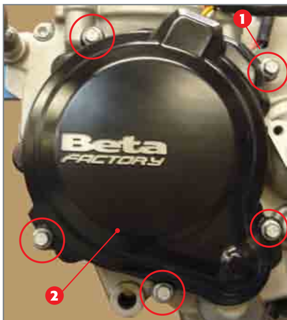
Fixing screws 1 of flywheel cover 2.
