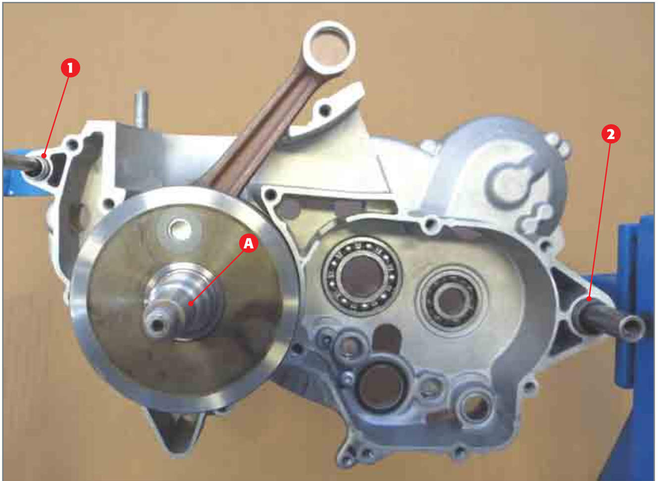
Insertion of crankshaft in right crankcase.
