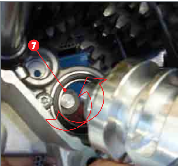
Insertion of desmodromic device in specific bearing. Note the rotation of the stop lever.
