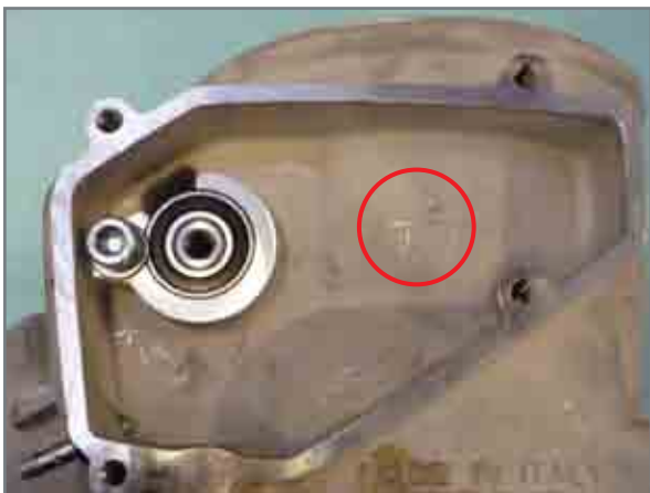
Punching of cylinder class.
