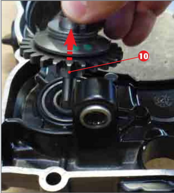
Extraction of centrifugal unit.
