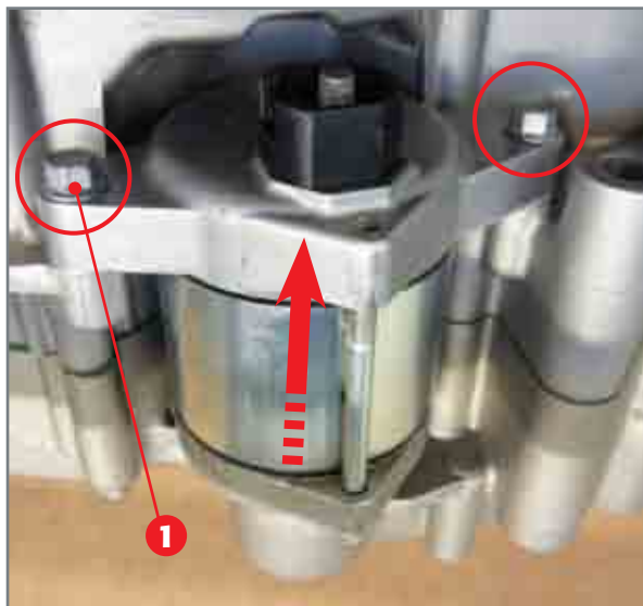
Removal of start motor.
