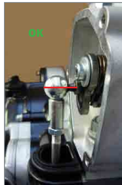
Correct position of the control rod seat.
