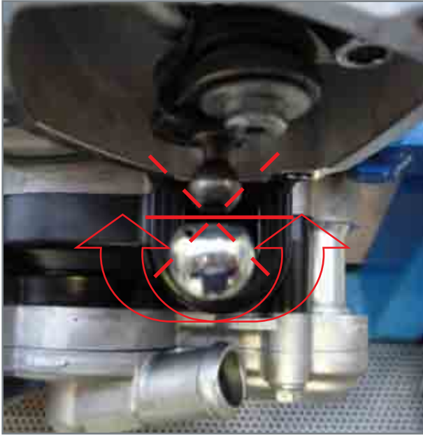
Check of control rod rotation.
