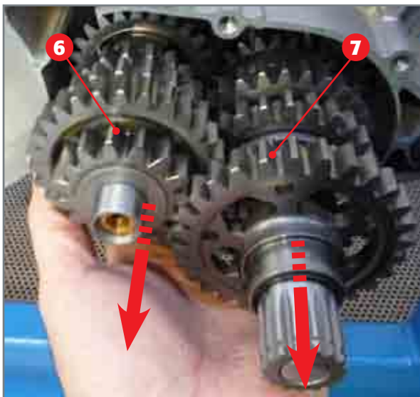
Extraction of complete gearbox unit: 6 main unit, 7 secondary unit.
