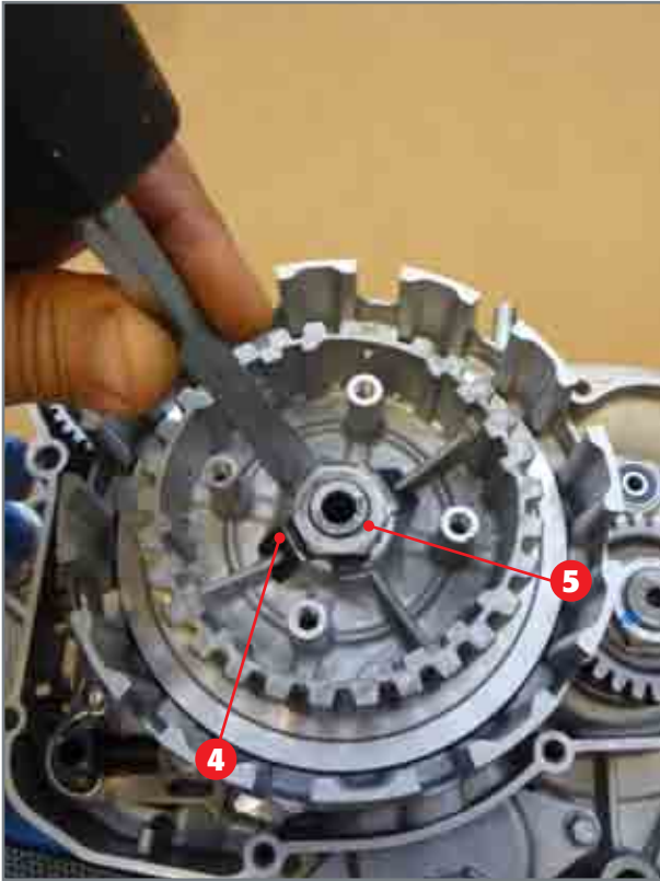
Opening of the safety washer with chisel.
