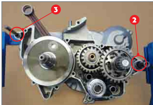
Crankcase half reference pins.
