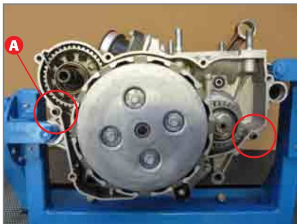
Two centring pins A for inner clutch cover coupling.
