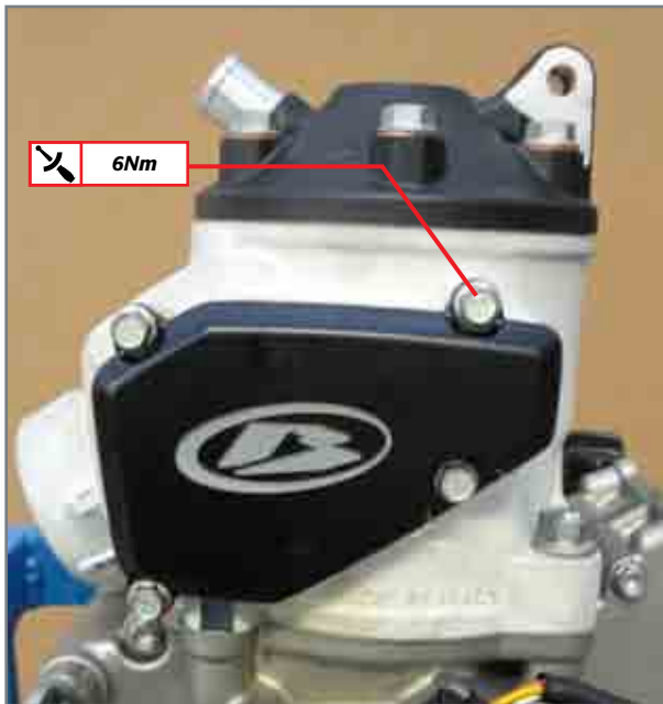
Application of resonance chamber cover and relative screws.
