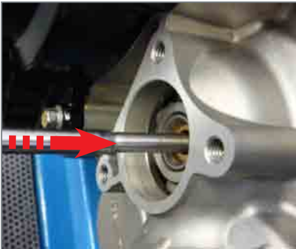
Insertion of clutch rod.
