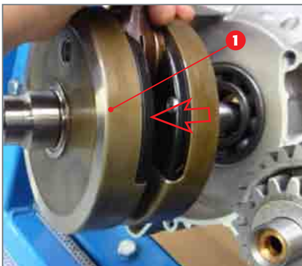
Removal of crankshaft.
