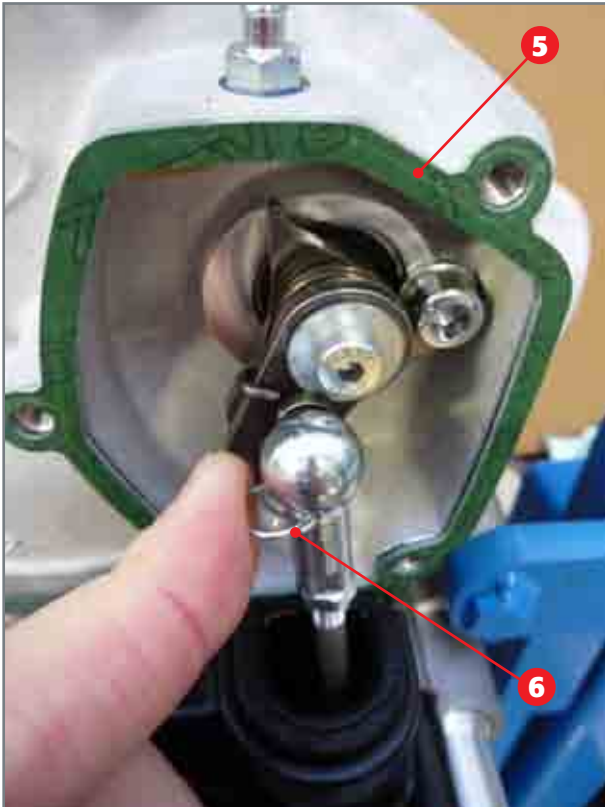
Insertion of control rod and application of stop.
