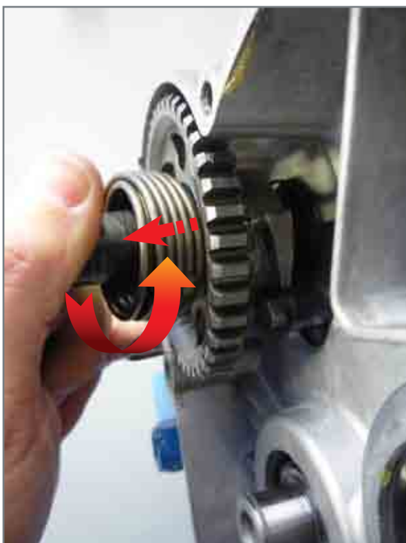
Extraction of shaft from crankcase.
