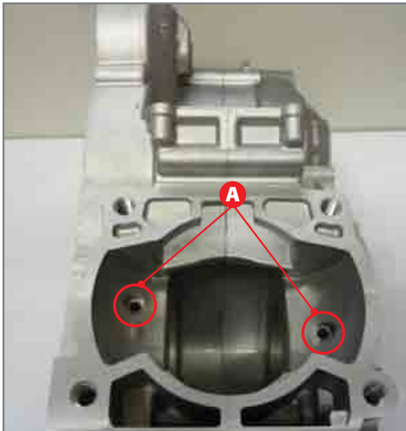
Crankshaft bearings lubrication holes.
