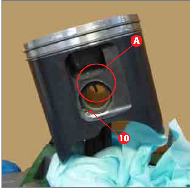
Removal of piston circlip.
