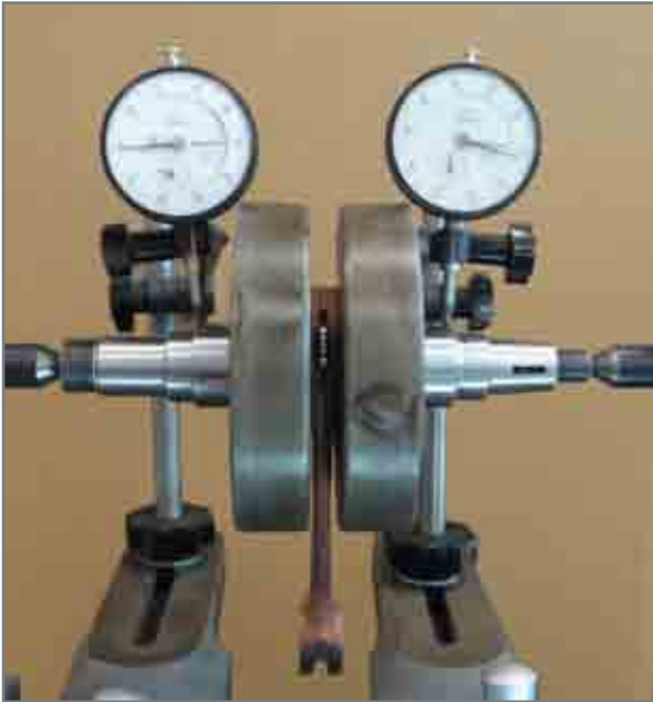
Deflection/Off-centring of crankshaft.
