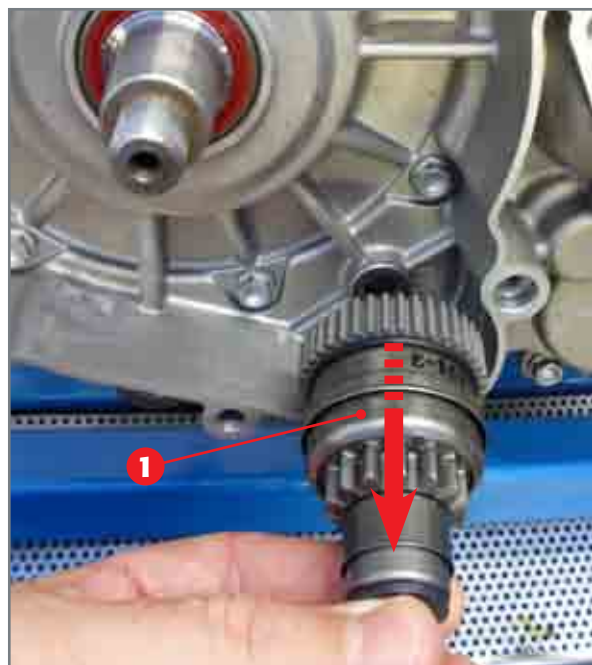
Removal of Bendix coupling.
