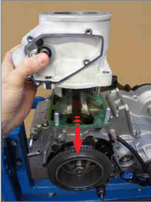
Coupling of cylinder to piston and crankcase-
