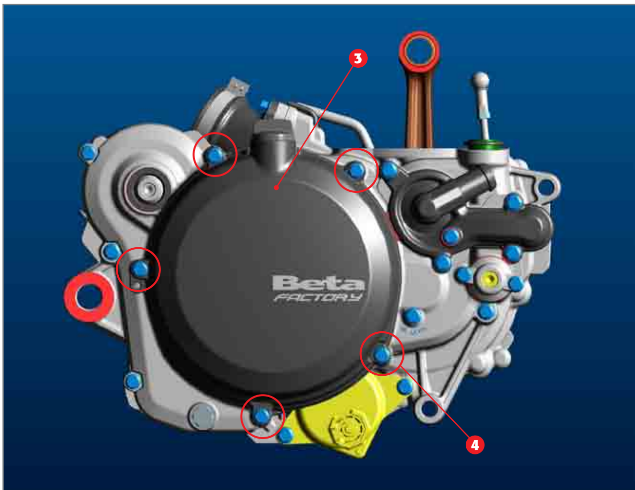
Outer clutch cover screws.
