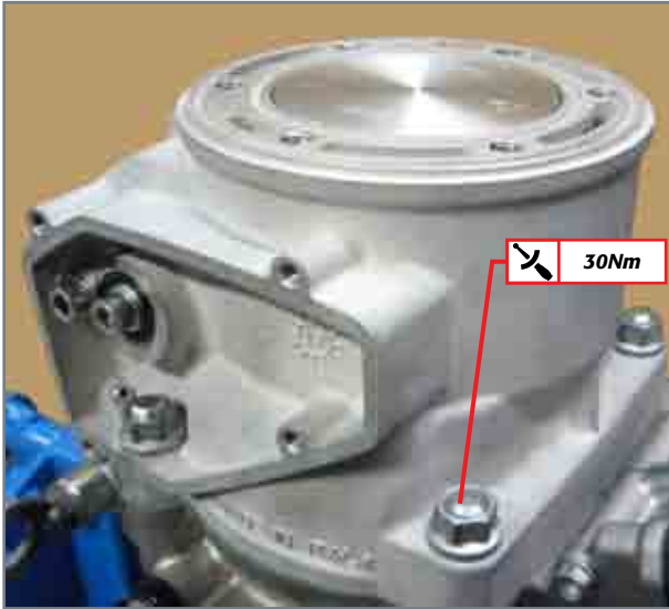
Fastening of cylinder nuts.
