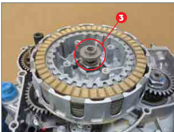
Pressure plate unit 3 and clutch disc pack.
