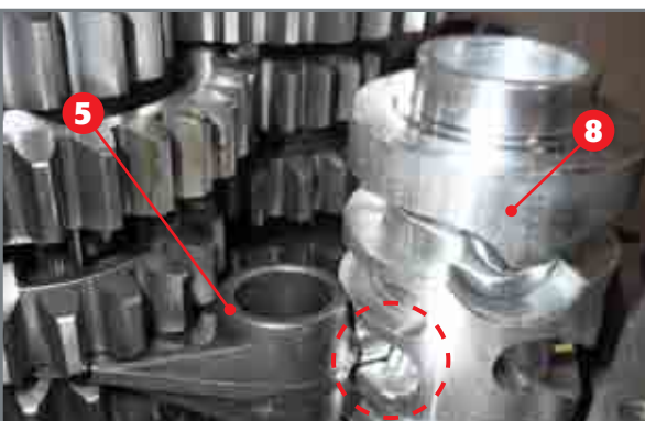
Place fork 5 of the primary unit in the central guide of desmodromic device 8.
