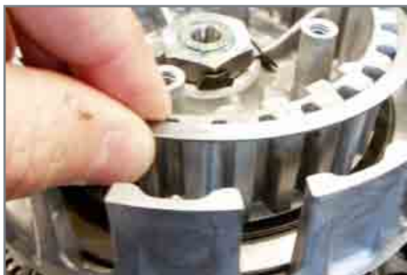
Removal of disc spring assembly.
