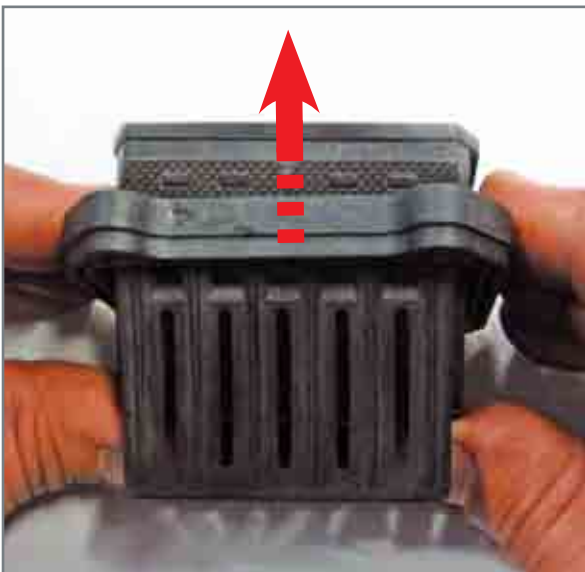
Disassembly of reed valve body.
