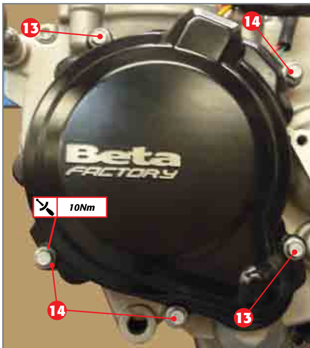
Flywheel cover coupled to crankcase.
