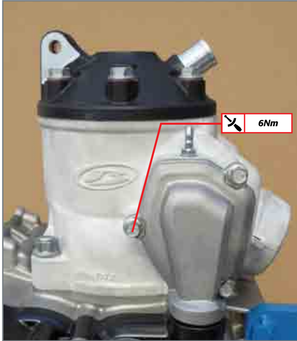
Application and fastening of valve control unit cover screws.
