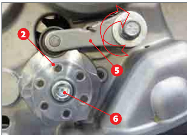
Disassembly of stop cam.
