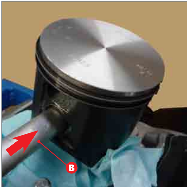
Removal of pin bolt.
