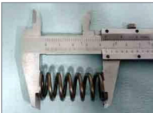
Clutch spring length measurement.
