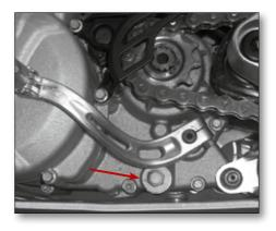
Unscrew the plug in the left-hand casing and use pliers to extract the filter. Clean it carefully and blow it through with compressed air. Check for damage to the O-rings, and replace them if necessary. Refit all the parts and tighten the plug to 15 Nm.
