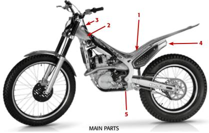
1 - Filter box 2 - Fuel tank 3 - Fuel filler cap 4 - Silencer 5 - Kickstart lever
