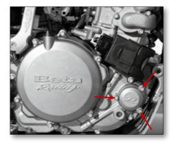
Extract the paper filter using pliers. Check the condition of the O-ring too, and replace it if necessary.
