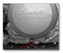
Execute same procedure for the filter located on the right side of crankcase.
