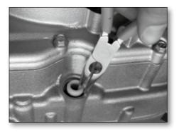
Put a drawn pan under the engine closer to the paper filter cover and then unscrew the cover.
