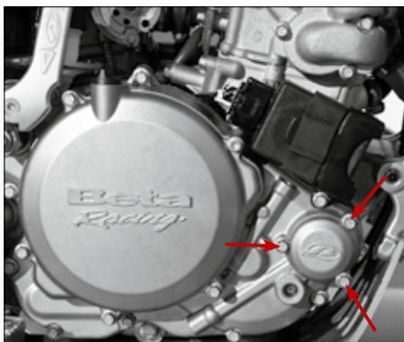
Put a drawn pan under the engine closer to the paper filter cover and then unscrew the cover.
