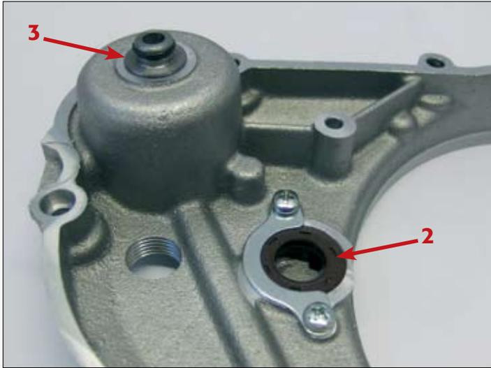
Fit the crankshaft oilseal (2) in its housing, with the open side facing inwards. Remember to grease the outer surface to facilitate seating. Then secure the oilseal with its retaining plate and tighten the screws to a torque of 3 Nm, after applying medium-strength thread lock.
