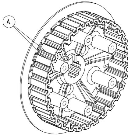
Lock the clutch hub with the special tool and tighten the nut to 90 Nm.
