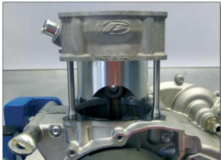
*N.B. Ensure that the cylinder base gasket is in position before fitting the cylinder.*
