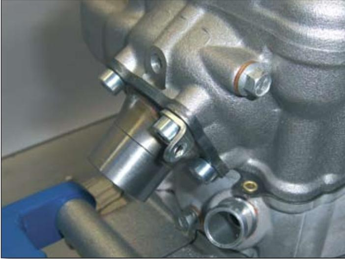
Fit the exhaust flange (12) with four M6x15 screws (14) tightened to 10 Nm. Under the heads of the screws fit the two plates (13) for anchoring the exhaust collector support springs. These plates are fitted to the top right and bottom left bolts, looking at the engine from the front (exhaust side).
