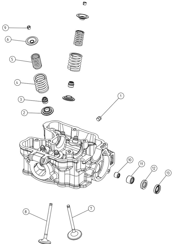
After you have greased the valves and fitted them into their guides (inlet 7, exhaust 8), secure them with the split collets (9) using the special tool (A). The operation must be carried out individually for each valve.
