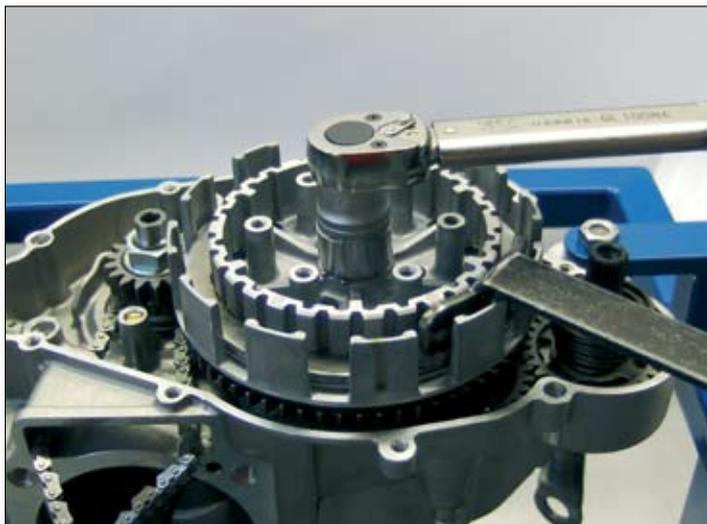
Which locks the retaining nut (9) for the clutch hub (11) and unscrew the nut, using the special tool for locking the clutch centre.
