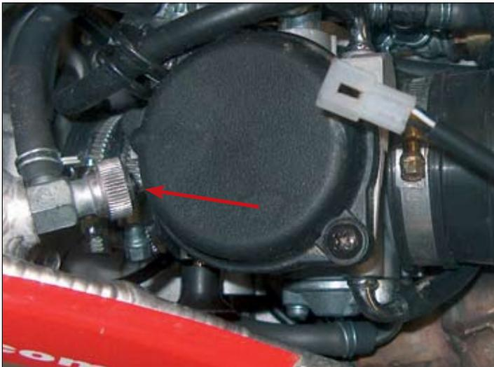
Close the tap on the fuel tank by screwing in the relevant knob.
