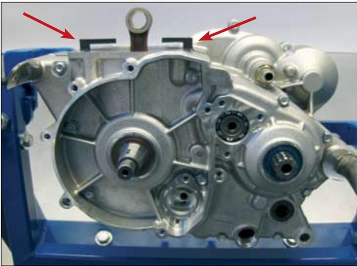
Accurately cut the protruding part of the cylinder base gasket, taking care not to damage the surface on which the cylinder will rest.
