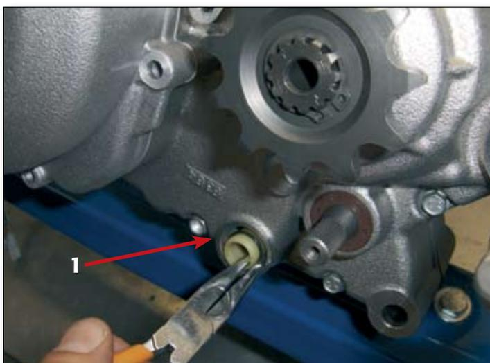
Take out the oil filters from the left-hand (1) and right-hand (2) crankcase halves after first removing the filter covers.
