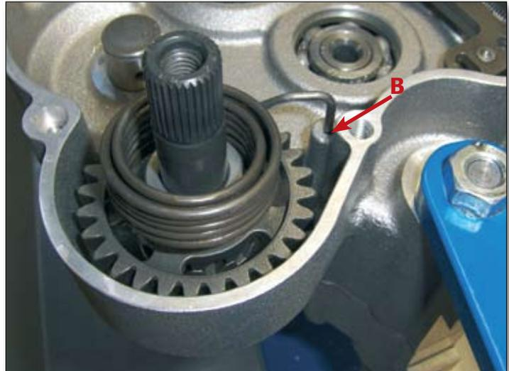
Fit the kickstart idler gear (17) on its shaft, together with the two 18x27x0.5 thrust washers (16, 18), after you have lubricated the parts in contact with each other, and secure it with the circlip (19). Ensure that the convex side of the gear is facing towards the crankcase.
