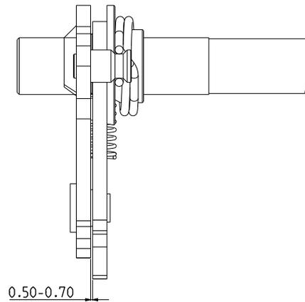
Position the spring (1) and the detent lever (2) in their housing and hold them in place with the idler pivot pin (3). Secure with the M6x25 bolt (4) tightened to 10 Nm after applying medium-strength thread lock.
