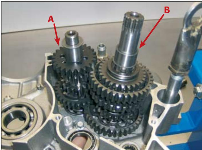
*N.B. Check that the gears slide correctly.*
