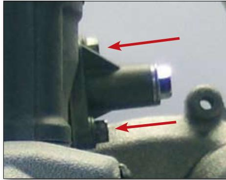
Remove the water pump shaft, taking care that the gear does not fall into the crankcase. Remove the fixed camchain guide.
