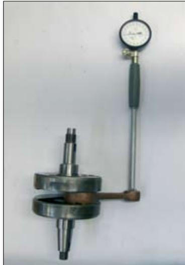
Measure the internal diameter of the conrod small end and then determine the play with the piston pin. If this value exceeds the limit, with the diameter of the piston pin within limits, replace the connecting rod.
