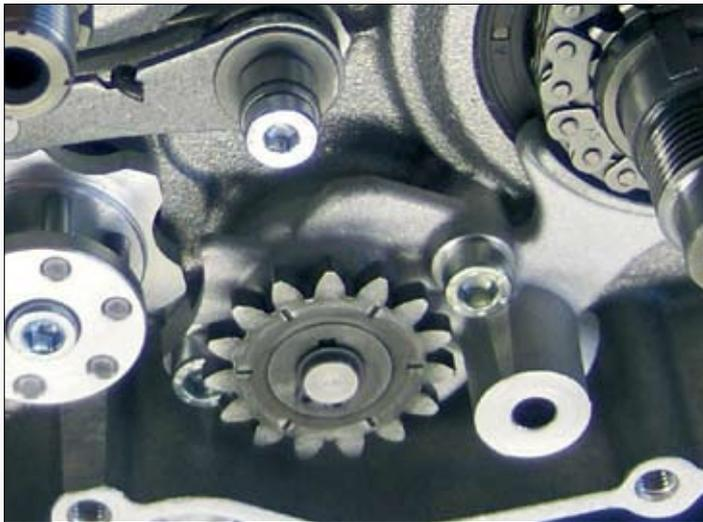
Refit the cover (4), after you have blocked the hole with the oilway expansion plug (5), and tighten the M6x20 screws (6) and M6x15 screws (7) to 10 Nm.
