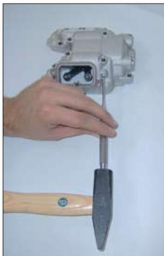
Fit the inlet rocker (2) and the exhaust rocker (3) as indicated in the photo, inserting the 12x17x0.5 thrust washers (7) between the rockers and the head cover, after you have lubricated them well with engine oil.
