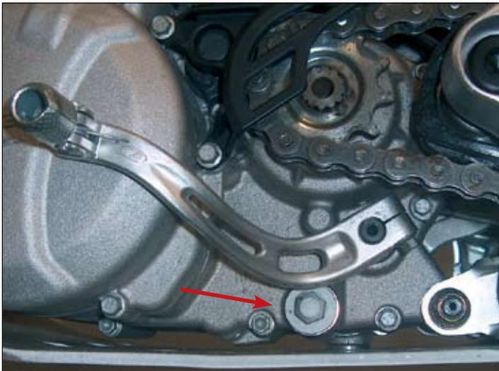
Unscrew the plug in the left-hand casing and use pliers to extract the filter. Clean it carefully and blow it through with compressed air. Check for damage to the O-rings, and replace them if necessary. Refit all the parts and tighten the plug to 15 Nm.
