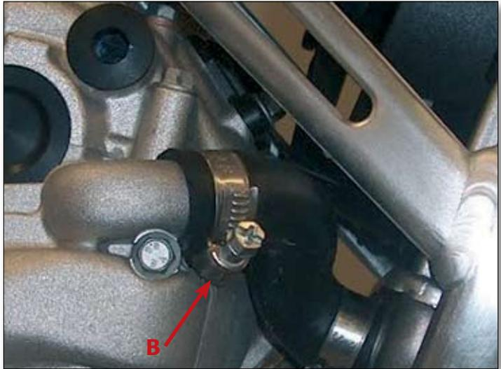
Loosen the clamps that secure the cooling system pipes respectively to the cylinder (A) and the water pump (B).
