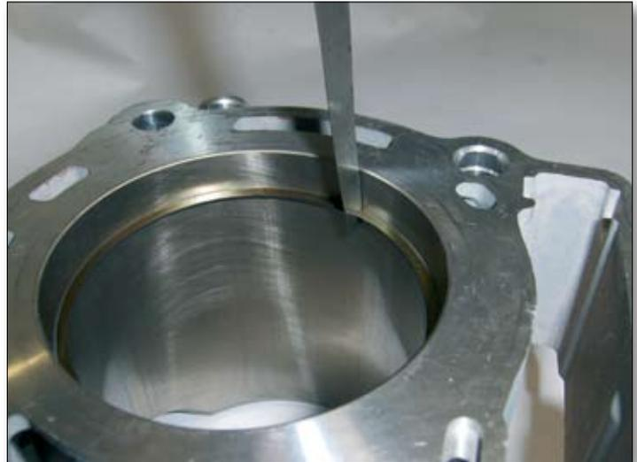
Use a feeler gauge to measure the play between the compression rings and the ring grooves in the piston. If these values exceed the maximum, with piston ring thicknesses within the prescribed limits, the piston must be replaced.
