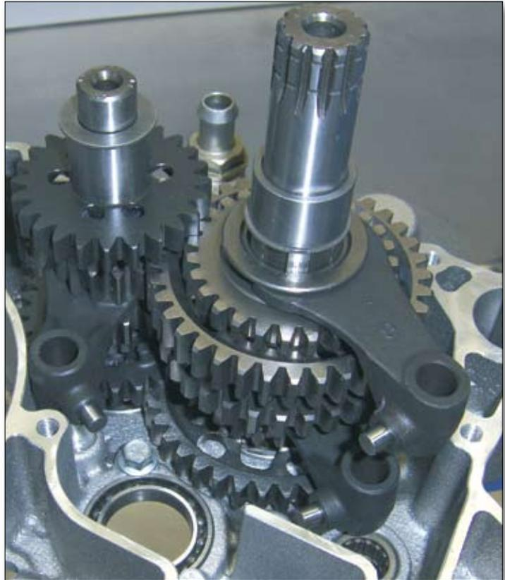
Check the wear on the guides in the selector drum. Locate the drum in its bearing and locate the pegs in the guides. Push the two pins through the forks, taking care to use the longer one for the forks on the secondary shaft.
