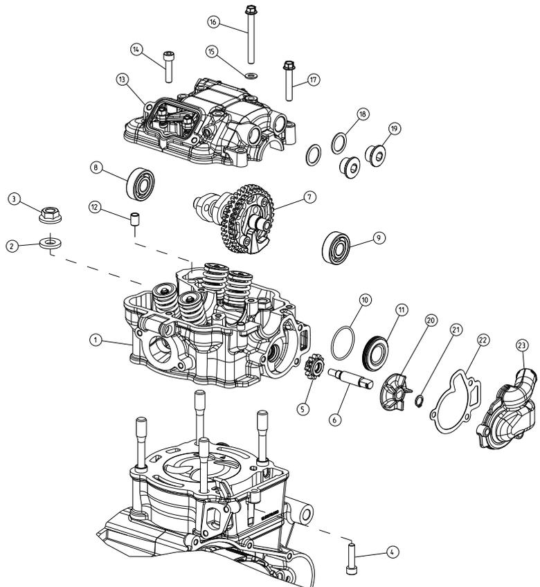
Fit the water pump drive sprocket (5) into its housing in the timing case, with the smaller-diameter face towards the inside, and then the water pump shaft (6) after you have lubricated it with oil.
