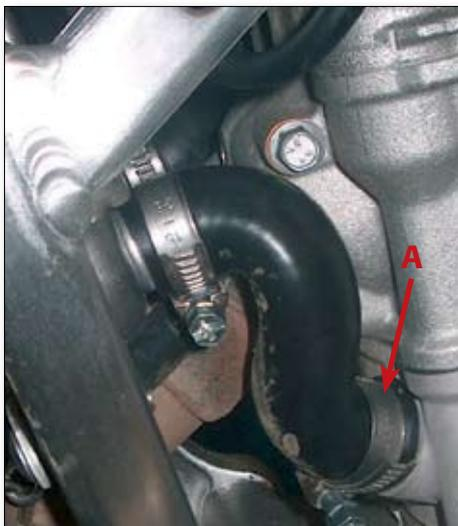
Pull off the sparkplug cap and unscrew the upper bolt (A) securing the coil support.
