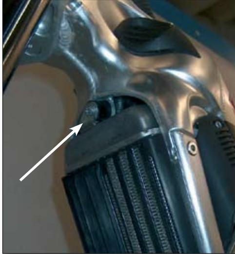
Unscrew the bolt securing the radiator and then remove the entire radiator/stay assembly after disconnecting the connectors for the electric fan and the radiator sensor.
