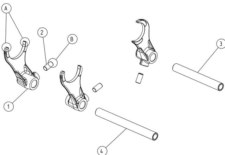
Check the state of wear of the contact areas between the selector forks and the grooves in which they run in the gears (A), and between the pegs and the grooves in the selector drum (B).
