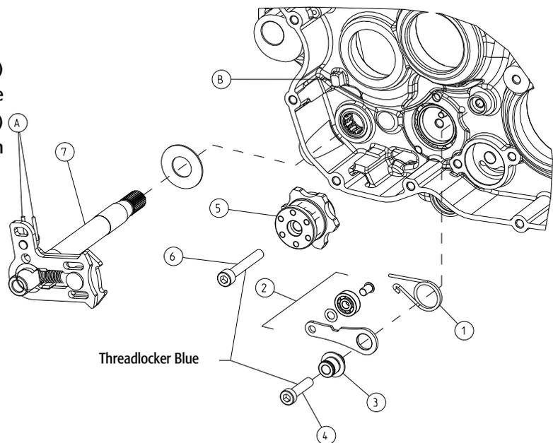
Move the detent lever out of the way and fit the detent cam (5). Secure with the M6x35 bolt (6) tightened to 10 Nm after applying medium-strength thread lock.
