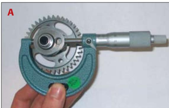
Measure the maximum length of the cams (A) and the diameter of the base circle (B).
