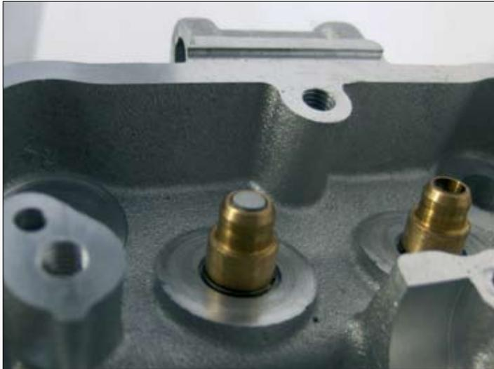
the seat. Then insert the valve into the guide until it is pressing against the seat, and rotate it on its axis. When the valve is removed, the dye will be missing on the contact area. The width of this contact area must fall within certain limits:
