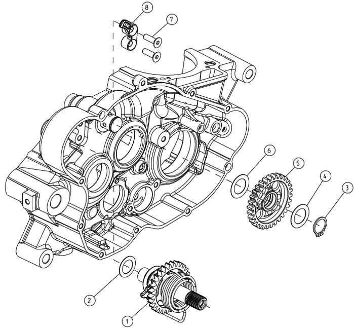
*N.B. Take care when extracting the kickstart return spring from its housing. Because it is under preload, it can cause injury as a result of rapidly springing back to its rest position.*
