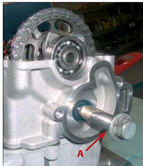
Remove the camchain tensioner by unscrewing the two retaining bolts.
