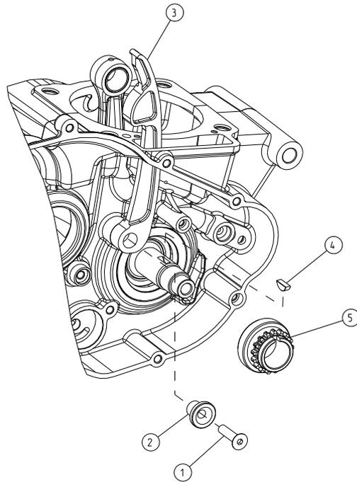
Use an engineering chisel to remove the woodruff key (4) from its housing in the clutch side crankshaft end, and then extract the timing gear (5).
