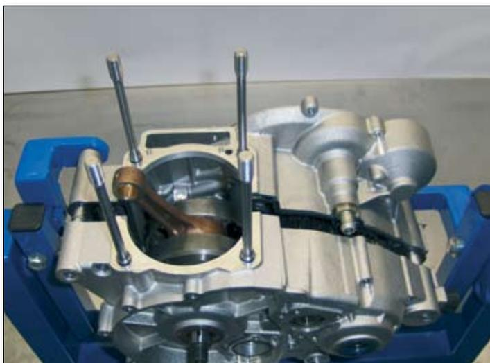
Then screw in the bolt at the end of the special tool until the two crankcase halves are separated, and manually take off the left-hand crankcase half.
