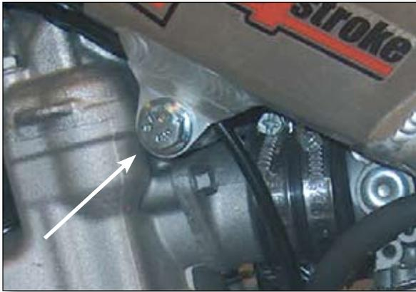
Take out the bolt securing the cylinder head to the frame.
