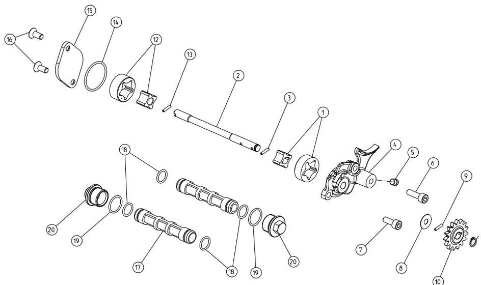
Use a feeler gauge to check the clearance between inner rotor and outer rotor. If you find that there is play beyond the permitted limits, replace the pump.
