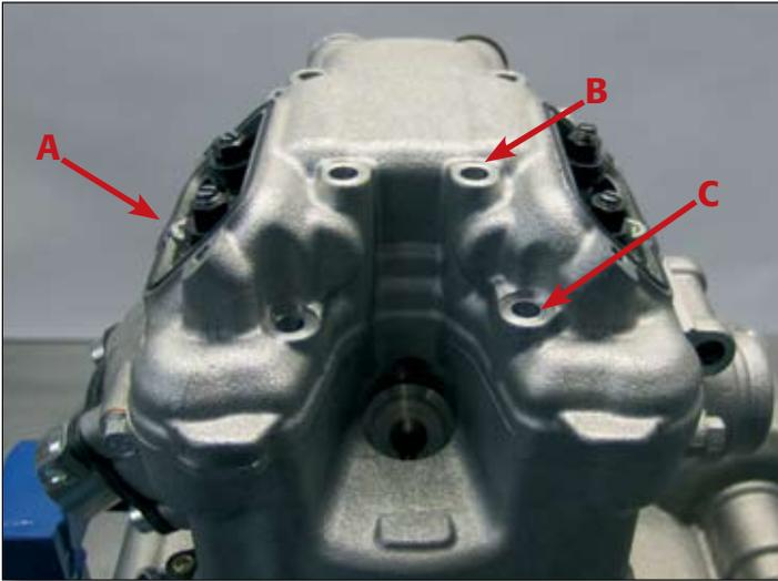
Remove the valve covers and then take out all the bolts securing the cylinder head cover: 2 M6x25 bolts (A), 4 M6x55 bolts (B) and 4 M6x35 bolts (C).
