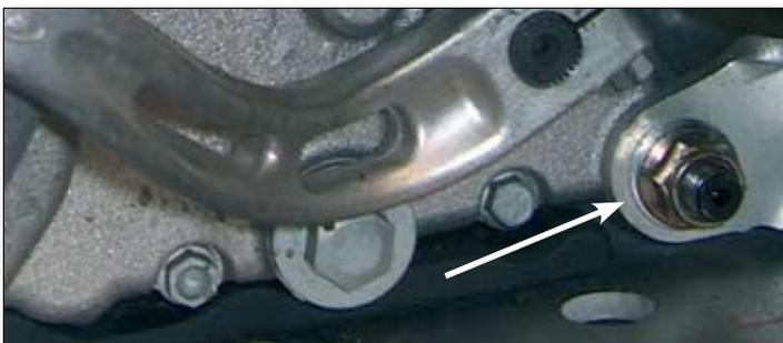
Slack off the nut securing the lower engine/frame mounting bolt.
