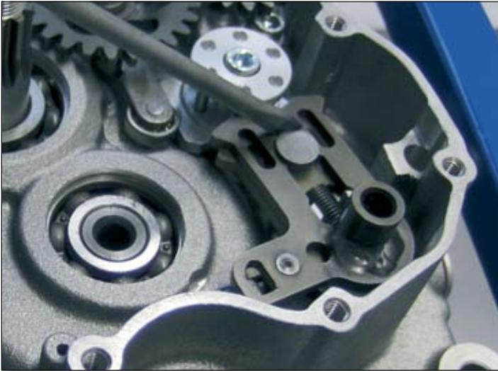
Take out the gearchange shaft (1), pushing back the movable pawl with a screwdriver to prevent it from interfering with the gearchange detent cam.
