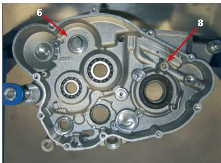
While the crankcase is still hot, use a press to fit the shaft (6) for the kickstart idler gear on the right-hand side.
