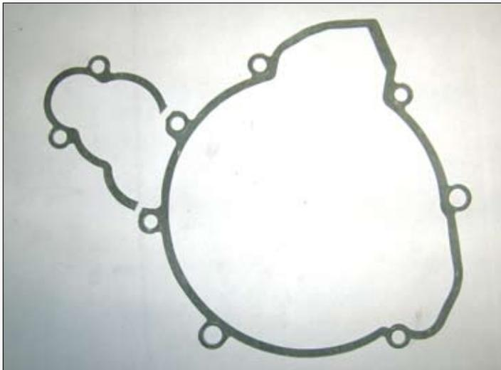
*N.B. Before you apply the gasket, cut off the excess section as shown in the picture above.*
