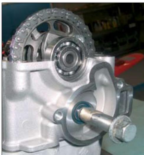
Screw the water pump shaft (6) into the gear (5) (which is locked by the camchain) using the appropriate special tool.
