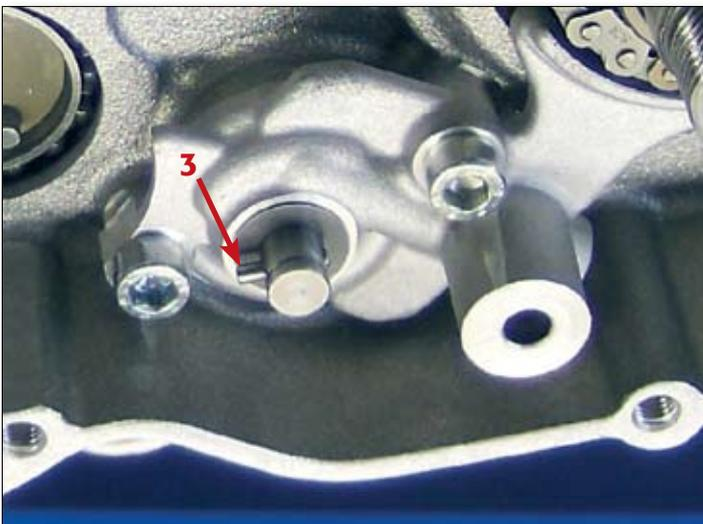
Remove the pin (3) which carries the drive from the gear (2) to the oil pump shaft (8), and then the thrust washer (4). Remove the oil pump cover (7) after first unscrewing the retaining screws (5, 6).
