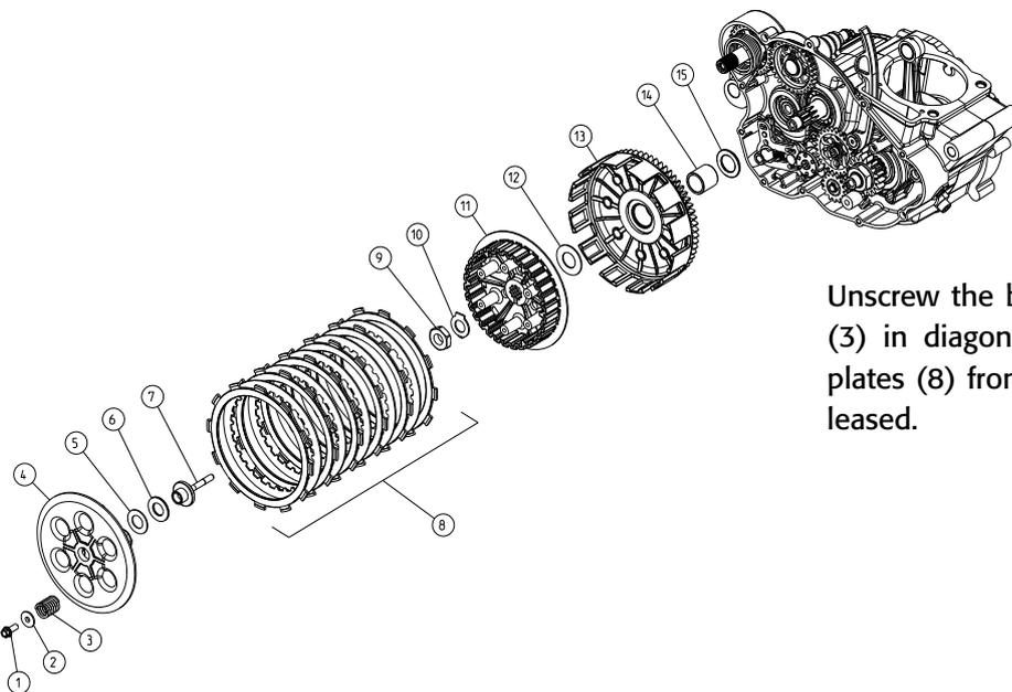
Unscrew the bolts (1) retaining the clutch springs (3) in diagonal sequence to prevent the friction plates (8) from jamming when the springs are released.
