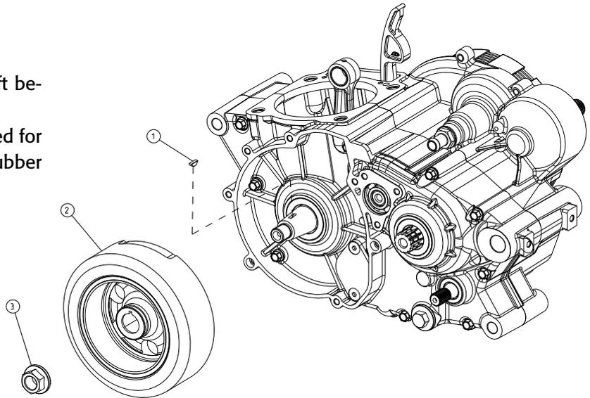
Fit the flywheel (2) and secure it with the flanged nut (3), tightening to a torque of 120 Nm.
