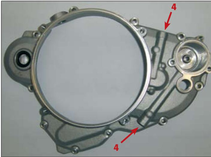
Close the oilways with the special oilway expansion plugs (4), using a pin punch.
