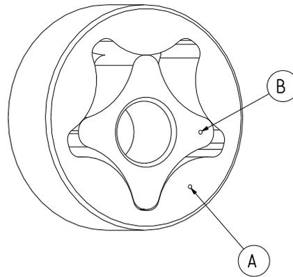
Position the engine bottom end with the outer side of the right-hand crankcase half facing upwards. Locate the pump (1) in its housing in the right half of the crankcase, after oiling it well, with the reference marks facing towards the inside, so that they are not visible once the pump is fitted.
