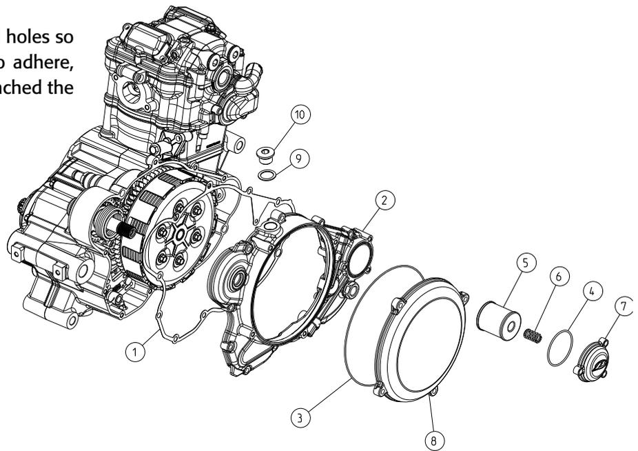
Fit the clutch casing (2) with its retaining bolts, tightening them to 10 Nm.
