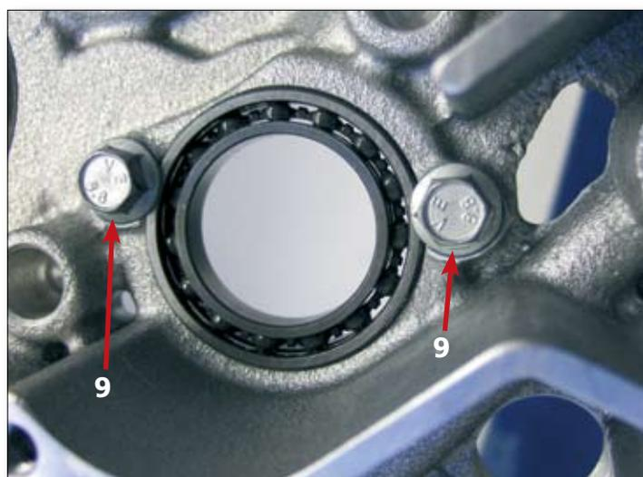
Fit the oil jets (8) and secure the selector drum bearing (4) with its retaining bolts (9), applying medium-strength thread lock tightening these to 10 Nm.
