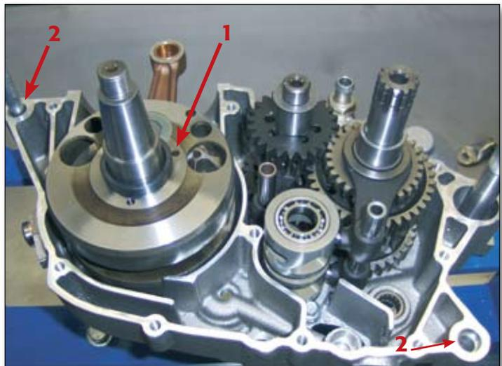
Grease the area of the crankshaft which needs to slide into the oilseal in the left-hand crankcase (1), and fit the crankcase centre gasket, cutting it in the cylinder area (2) to avoid interference with the connecting rod during assembly.
