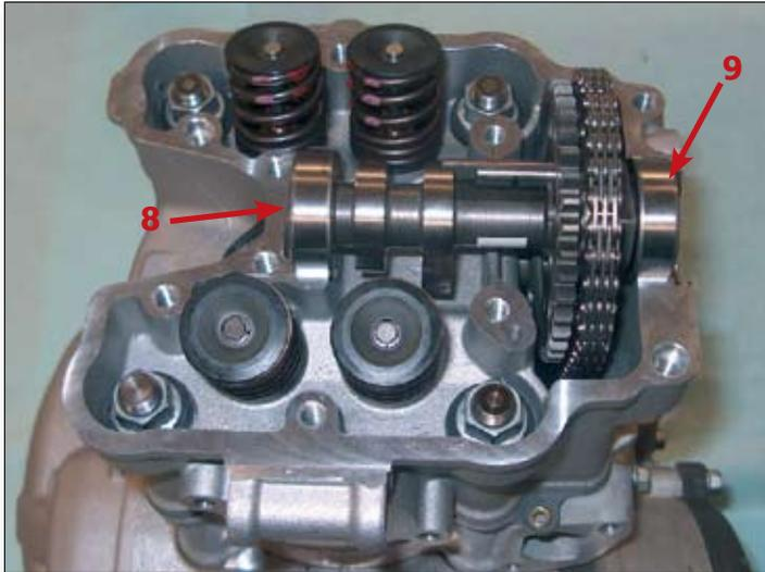
Pass the camchain around the camshaft sprocket, and fit onto the camshaft first the sealed bearing (8) and then the bearing on the chain side (9).
