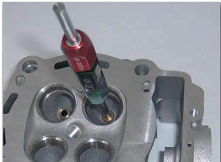
Check the valve stem/valve guide play. To do this, locate the valve in its guide with the top surface of the valve stem flush with the guide, and measure the maximum radial oscillation of the valve head.
