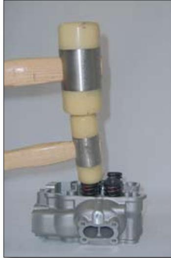
Apply a few taps to the upper spring caps with a double rubber hammer to help the split collets to settle.
