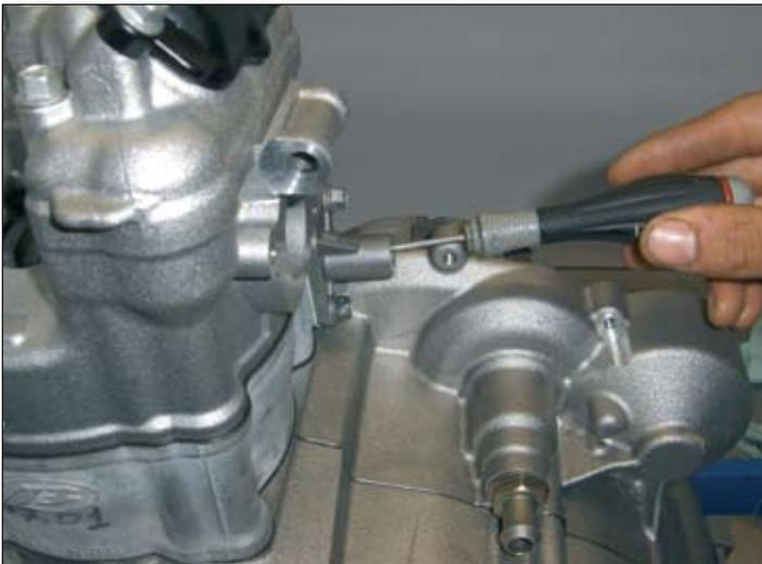
Fit the tensioner body and its gasket, retaining it with M6x16 bolts tightened to 8 Nm. Use a screwdriver to push the plunger so as to put the camchain under tension. Then insert the spring and washer and, finally, screw in the bolt.
