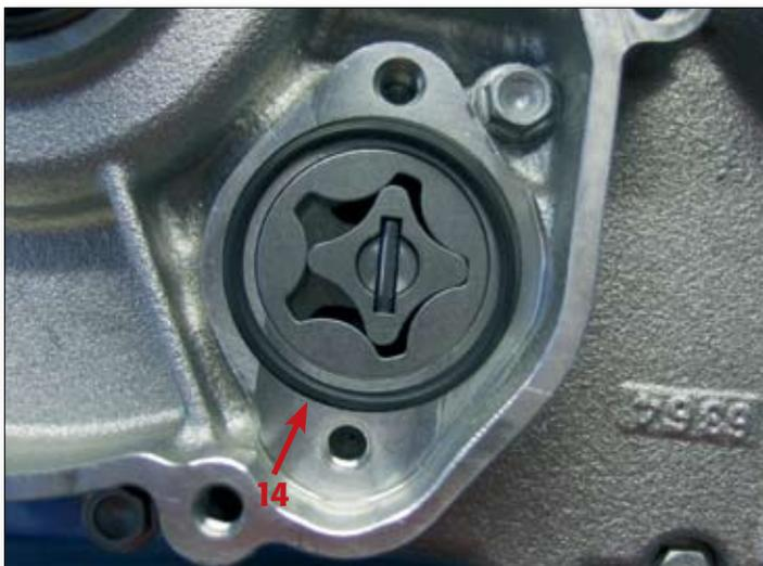
Fit the O-ring (14) into its seat and refit the cover (15) to the pump.
