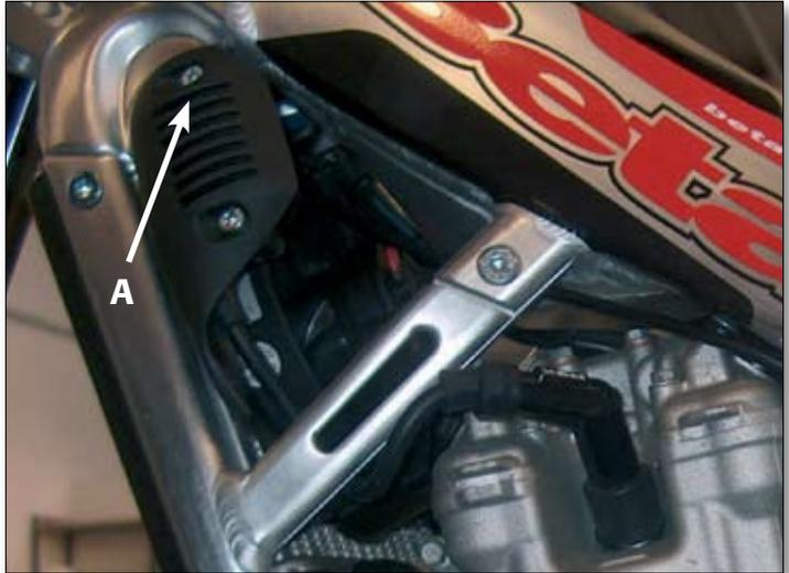
Unscrew the bolts that secure the stay to the frame (A) and take out the front engine mounting bolt (B) after unscrewing it.
