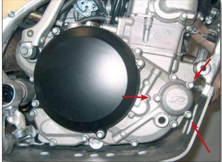
Then extract the paper filter using pliers. Check the condition of the O-ring too, and replace it if necessary. Change the filter and refit the cover, tightening the three M6x20 bolts to 10 Nm.
