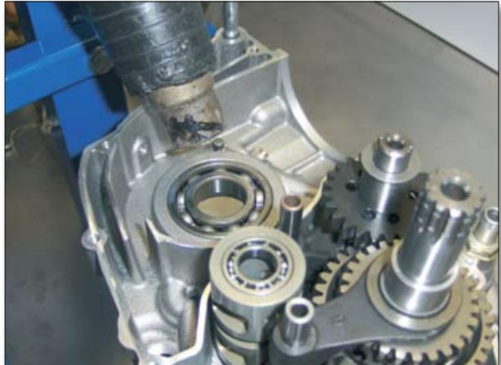
Fit the spacer (1) onto the crankshaft and the dowels into their housings (2).
