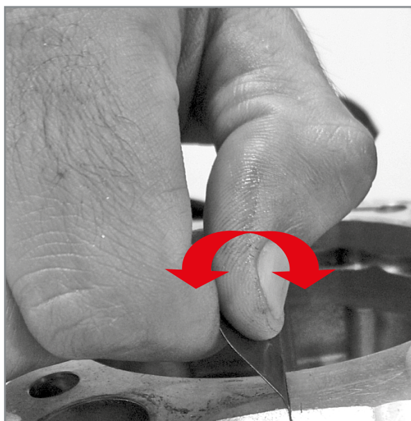
Cutting extra piece of gasket between engine crankcase halves.
