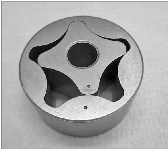
Oil intake pump: note the dot on the two rotors. The dot must face the inside of the engine.
