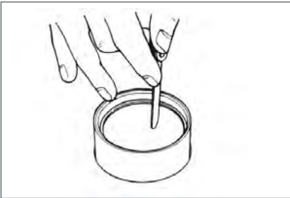
Elastic band wear limit check.
