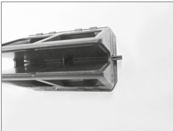
Disassembly of central wedges. The extraction of only one is shown in figure.
