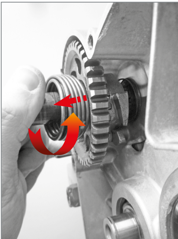
Extraction of shaft from crankcase.
