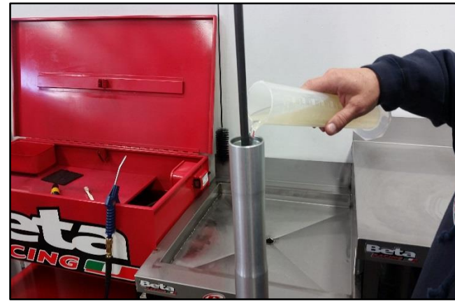
Fill the fork with high quality 5w fork oil to 500cc.
