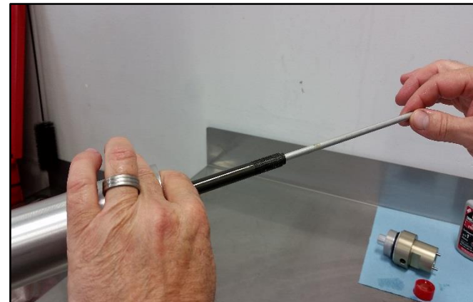
Grease and install the rebound adjuster rod.
