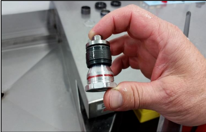
Apply high strength thread locking agent to the base valve threads.
