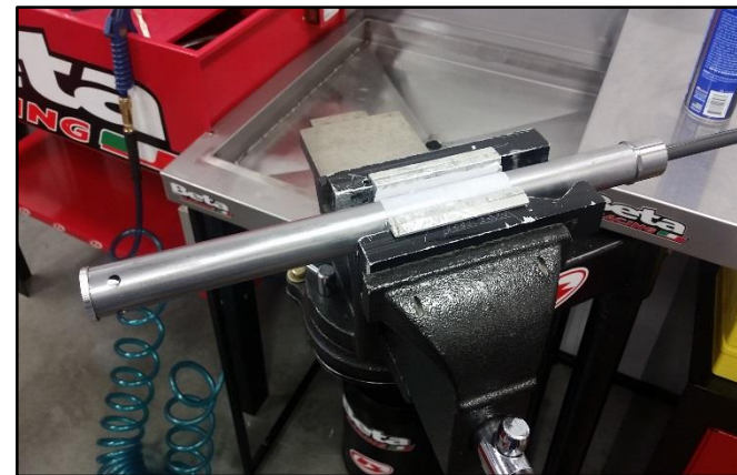
CAUTION: Hold the cartridge in the soft “V” jaw vice using paper between the jaws and cartridge and use only enough pressure to hold the cartridge, do not tighten or damage will occur.
