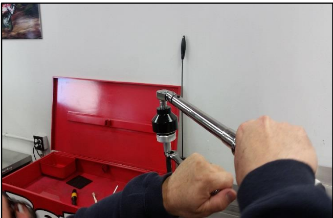
Reinstall the fork cap threading it on until it bottoms out. Run the nut up to the cap and tighten to 16Nm.
