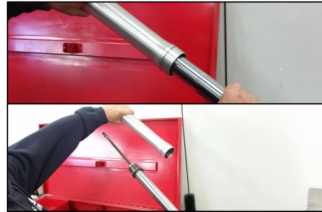
Holding the fork with both hands and with one quick motion, pull the tubes apart.
