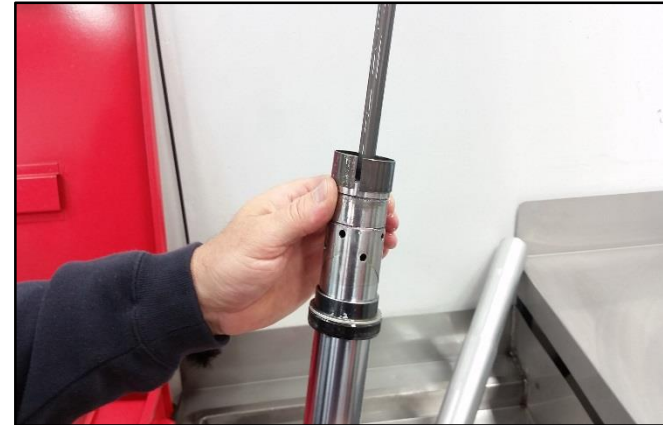
Remove the bushings, retaining washer, fork seal, retaining clip and dust seal paying attention to the order of removal and orientation. Clean and inspect all parts, replace worn bushings and seals.
