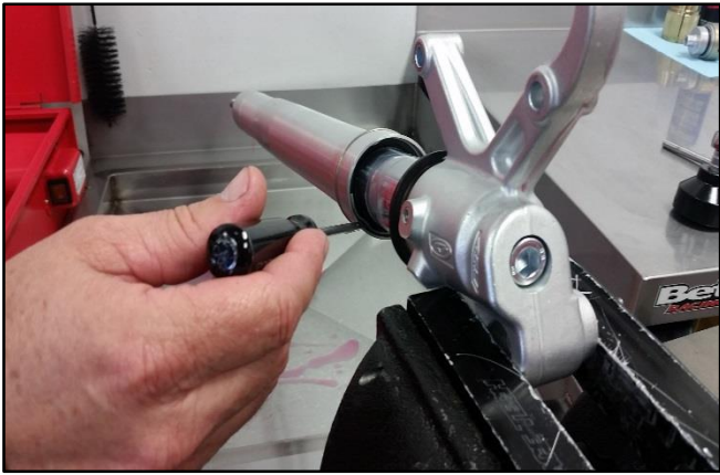
Remove the fork seal retainer clip.
