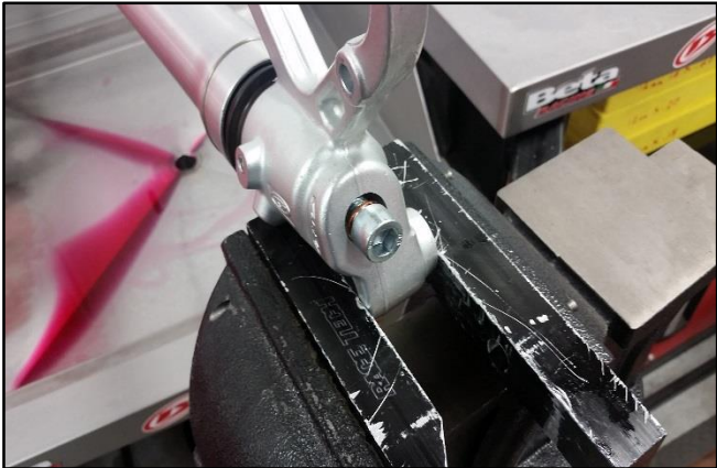
Remove the 10mm Allen bolt and copper washer from the bottom of the fork.
