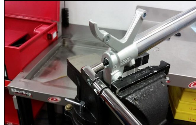
Insert the 10mm Allen bolt and copper washer and torque to 40Nm.
