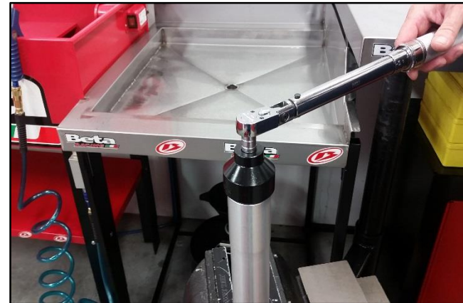
Put a drop of high strength thread locking agent onto the threads of the spring retainer cap and install, tighten to 40Nm.
