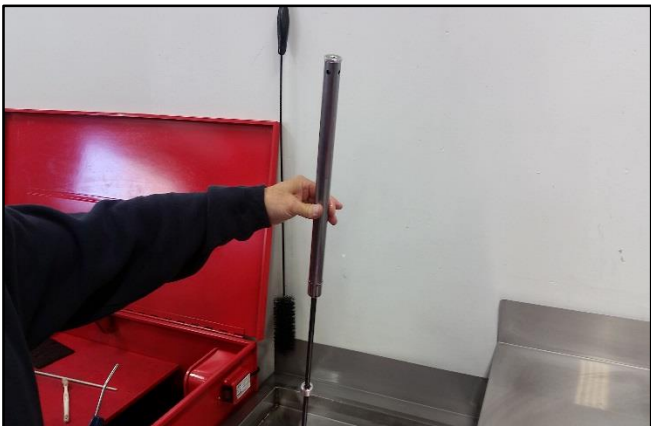
Remove the cartridge from the fork.
