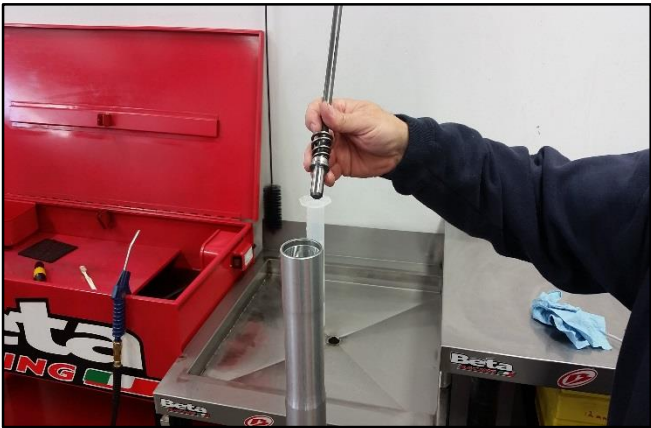
Insert the metering rod.
