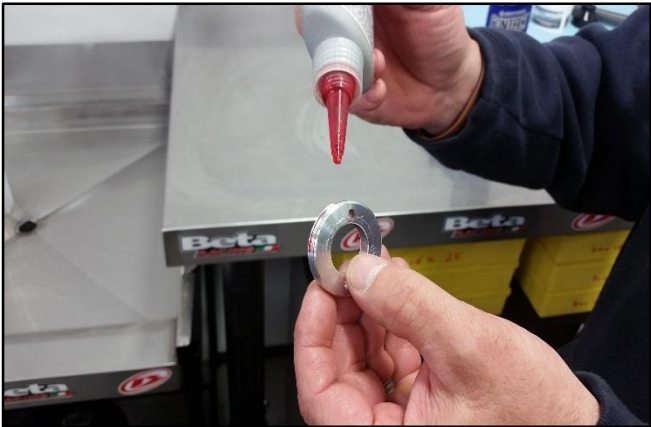
Put a drop of high strength thread locking agent onto the threads of the spring retainer cap and install, tighten to 40Nm.
