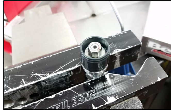
Put a drop of high strength thread locking agent on the nut and tighten to 10Nm.
