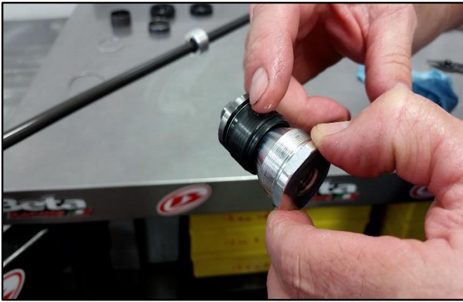
Apply oil to the base valve piston seal.
