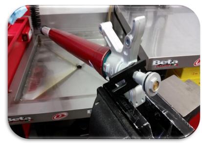
Press in on the cartridge exposing the cartridge rod, insert the holding tool.
