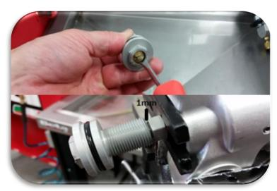
Back the rebound adjuster all the way out (counter clockwise).
