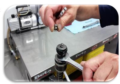
While holding the 17mm hex on the post, loosen and remove the 13mm shoulder nut.
