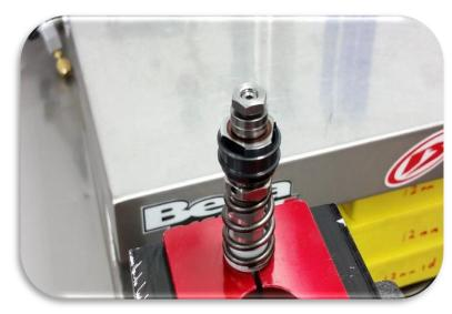
Remove the nut and apply 1 drop of red loctite. Carefully check that the delta shim is aligned then install the nut and torque to 5Nm.
