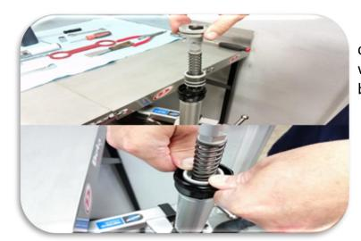
Carefully install the compression assembly without dislodging the bushing.
