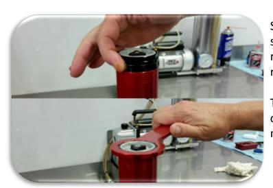
Secure the outer tube in the soft jaw vise. Apply seal and Oring grease to the top cap Oring and threads.
