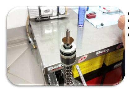
Clean the post then reinstall the shims in the order they were removed.
