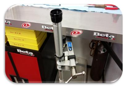
Secure the inner cartridge with a soft jaw vise or clamp.
