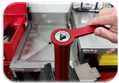
Unscrew inner cartridge from outer fork tube.
