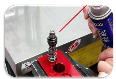
Loosely install the nut then thoroughly clean the stack with contact cleaner then blow off with air.
