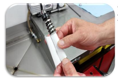
Wrap the top of the dampening rod with white paper to protect it.
