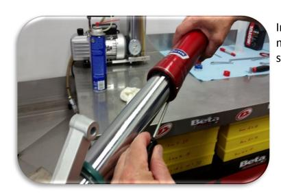
Install the retaining clip making sure it is fully seated into the groove.
