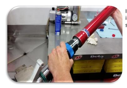
Install the fork seal and bushing into the outer tube using the seal driver.
