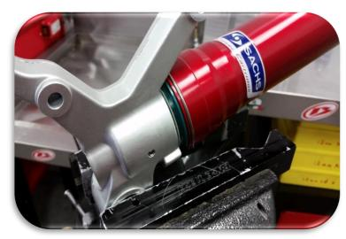
With the dust seal sitting against the fork lug, slide the outer tube down until the dust seal is seated.
