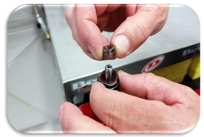
Remove the spacers making sure there are no shims stuck to the bottom.
