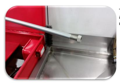
Thread the 15mm nut all the way onto the rod until it stops.
