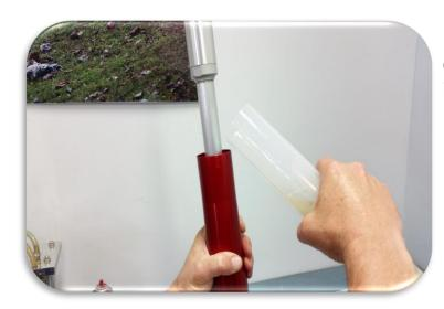
Measure out 350cc's of high quality 5w fork oil and pour it into the outer fork tube.
