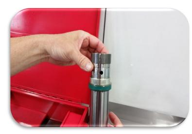
Remove the bushings, retaining washer, fork seal, retaining clip and dust seal paying attention to the order of removal and orientation.
