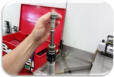
Remove the compression assembly from the cartridge.
