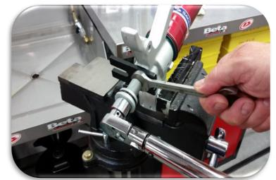
Turn the 15mm jam nut counterclockwise holding the rebound assembly with a torque wrench. Tighten to 10Nm.
