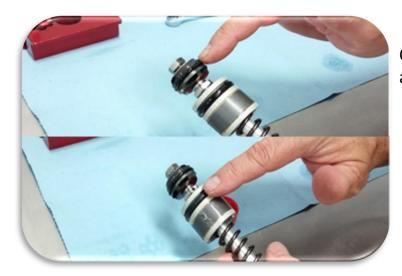
Apply 5w fork oil to the O-ring and floating piston assembly.
