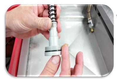
Apply suspension grease to the O-ring and threads
