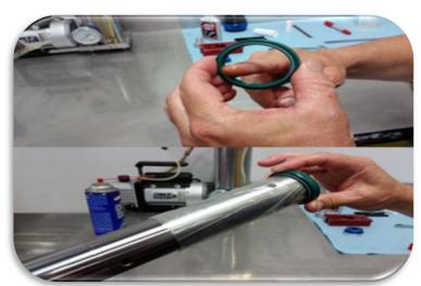
Apply seal and O-ring grease to the fork seal then slide it on the fork leg noting the orientation.
