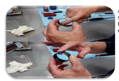
Apply 5w fork oil to both sides of the inner and outer bushings and install in there respective positions.
