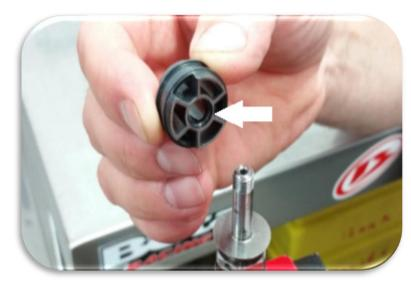
Install the rebound piston with the recess facing down.
