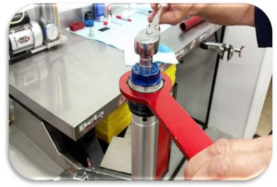
Unthread the compression assembly from the cartridge.
