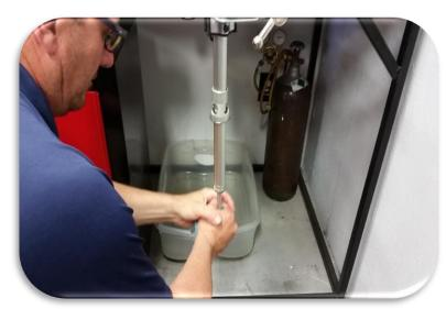
Slowly spin the dampening rod while gently moving the rod up and down roughly half of the travel from the fully-extended position to remove air bubbles.
