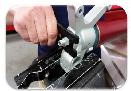
Press in on the cartridge to release pressure on the holding tool, remove the tool.
