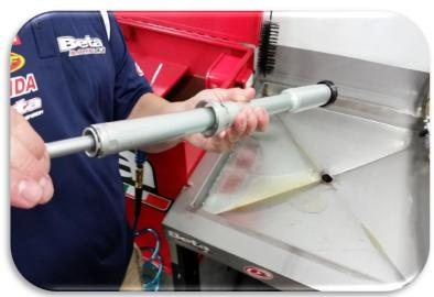
Drain the oil from the cartridge.
