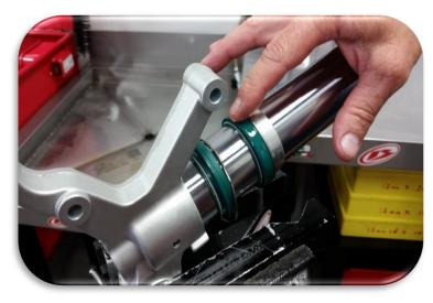
Apply 5w fork oil to the outer edge of the fork seal.
