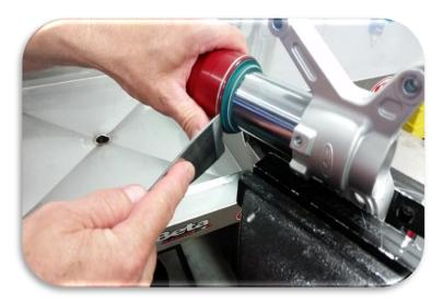
Separate the dust seal from the outer tube.
