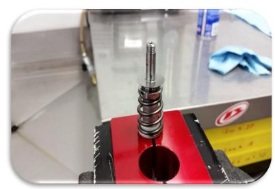
Carefully inspect the mid valve assembly then reinstall the shims and spring in the order they were removed.
