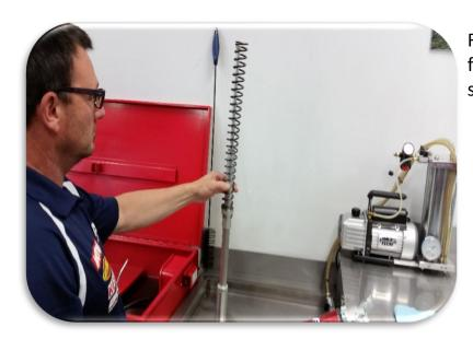
Remove the cartridge from the fork and the spring from the cartridge.
