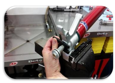
Press in on the cartridge and remove the holding tool.
