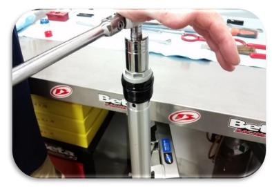
Using the compression assembly holding tool, apply pressure while turning to thread the compression assembly into the cartridge.
