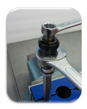
Carefully remove the 11mm nut while holding the 17mm on the dampening rod post as shown.
