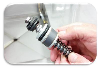
Inspect the O – ring and bushing, replace if damaged or worn.
