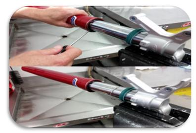
Unseat the seal retaining clip using the clip tool.
