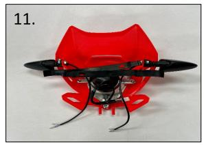
10. Install front blinkers onto headlight mask!
