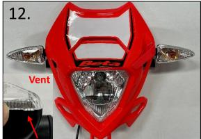
11. Make sure there is a vent facing the ground to provide draining when excess water enters blinker see image 12.
