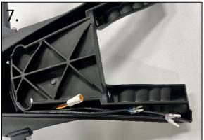
6. The wires should be oriented down the canal shown in image 7.
