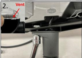
2. Begin installation of blinker lights on the provided rear fender extension. Install the blinkers as seen in image #2. Make sure to have the proper blinker in place. There should be a vent facing the ground to provide draining from water build up!
