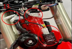
12. Locate the connections for blinker and relay in the wire cluster behind headlight. See image 13!
