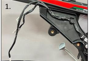
1. Remove the rear fender from the subframe.
