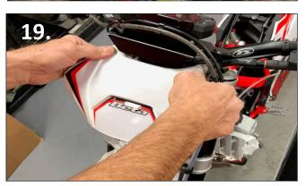
19.Connect the headlight plugs then insert the headlight mask locating pins into the front fender locating holes. Push down on the top of the mask bending it down then move it behind the black bracket and release it. Secure the mask straps.
