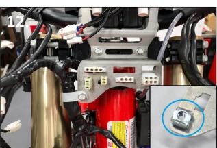
12.Install the main harness plugs into the slots of the stainless bracket. Remove the harness clamp nut from the stock bracket and install it into the stainless bracket.
