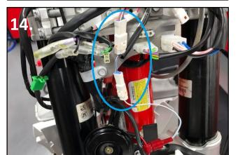
14.Connect the larger plug from the indicator lamps to the correct plug of the main harness and the other to the "T Tap". (Photo)
