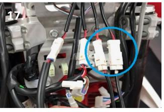
17.Connect the tach sensor and temperature sensor wires to the correct plugs of the dock.
