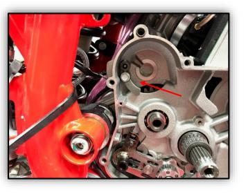
**5.** Remove the throw out assembly, then using the clutch holding tool Remove the 27mm nut, lock washer, flat washer and the complete clutch pack.
