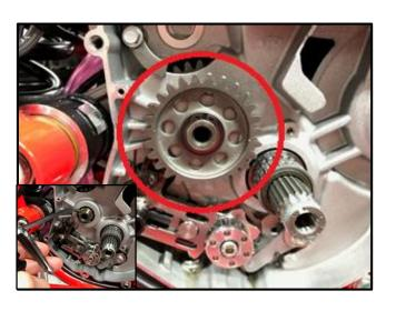
**7.** Apply oil to the transmission shaft then install the idler gear, washer, and clip.
