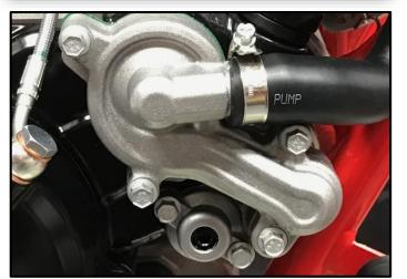
**15.** Install the water pump cover and radiator hose.
