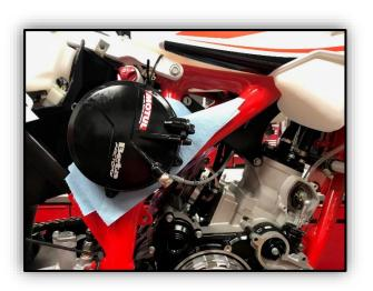
**4.** Remove rear brake pedal return spring and outer clutch cover bolts. Zip tie the cover up out of the way making sure not to lose the locating dowels.
