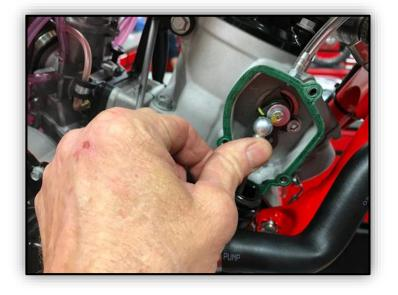
**16.** Push the power valve control rod head onto the ball end , re insert retaining clip. Apply high temp silicone on the lower power valve cover edges. Install cover and bolts, tighten bolts to 6 nm.
