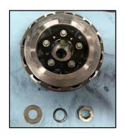
**6.** Use the provided 6mm bolt with Loctite to secure the return stop. Torque to 10Nm.
