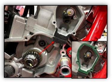
10. Apply high temperature silicone to the center case and cylinder where they meet at the power valve area. Reinstall the powervalve gasket.
