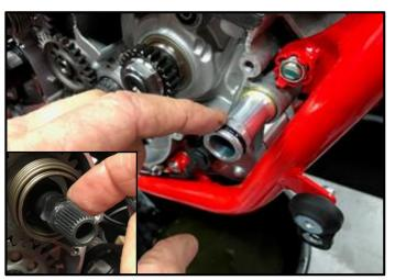
**11**. Apply grease to the coolant O-ring and kick start shaft.
