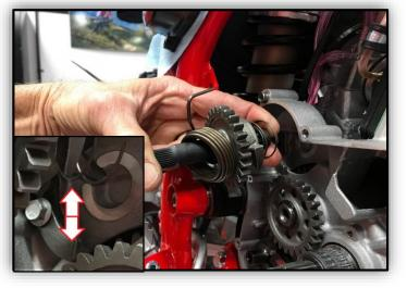
**8.** Install the kickstart assembly with the pawl just to the right of the stop.
