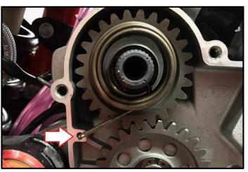
**9.** Making sure the return spring is centered around the shaft, rotate the spring clockwise until the end of the spring is aligned with the retention hole in the center case. Fully insert the the spring end into the hole, again checking to make sure your spring is centered around the shaft. The gears should spin freely.
