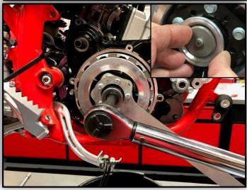
14. Reinstall the clutch assembly, flat washer, lock washer, and nut using blue Loctite. Use the clutch holding tool and tighten the nut to 120 nm. Install the throughout assembly. Install the outer cover and bolts leaving them loose and making sure the outer cover O-ring is in place.
