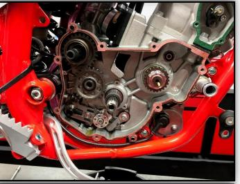
**13.** Install the inner clutch cover gasket making sure the alignment dowels are in place. Install the inner cover and leave the bolts loose.
