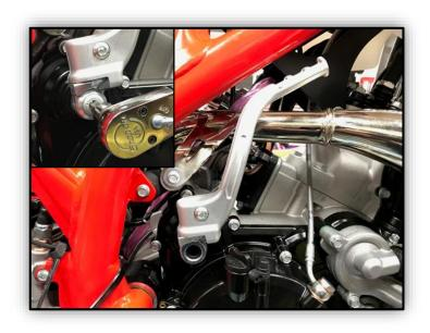
17. Reinstall the pipe and muffler. Carefully install the shaft seal. Install the kick starter lever on the shaft in a position where it clears the pipe. Install the washer and bolt using blue Loctite then tighten it to 25 nm.
