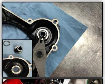
**12.** Remove the circlip from the back of the kick start plug located in the inner clutch cover, then push the plug out.
