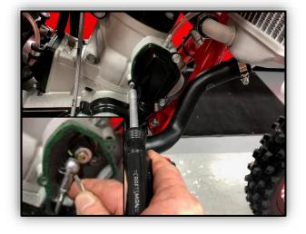
**3.** Remove Power valve cover (#3 tamper proof allen required) Remove control rod retaining clip from the control rod seat. Pry the control rod seat away from the ball head.
