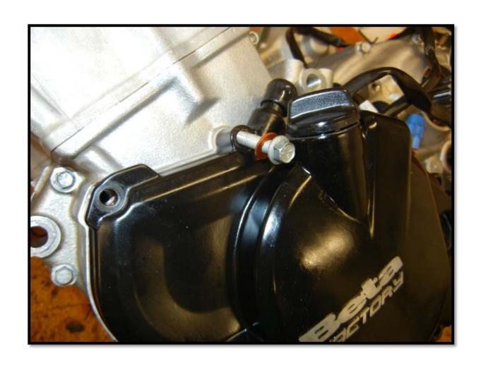
Remove the engine lock bolt, reinstall the thick copper washer and re-install the bolt.
