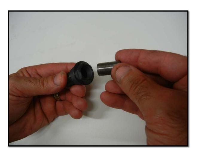
Install the assembly with oring into the cylinder.
