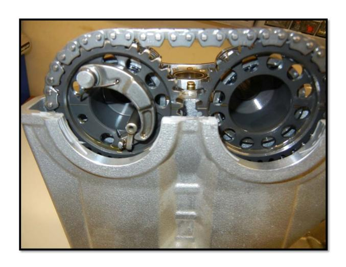
When cams are correctly timed, lobes will be in a 10:00 and 2:00 position with the timing marks aligned.
