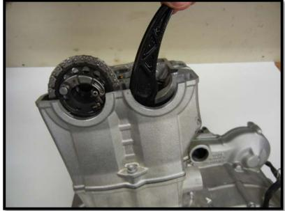
Install the new style rear cam chain guide. Note that you will need to remove the spacer from the bolt as the new guide is supplied with one. Be sure to apply red loctite to this bolt! This new guide has a built-in steel support designed to work with the new tensioner.
