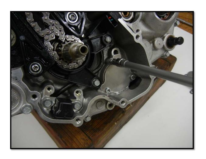
Important note! There is a check ball and spring behind the oil pump plate. Make sure these parts do not fall out major engine damage will result if not installed
