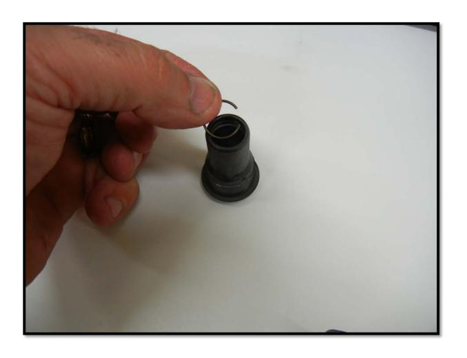
Apply a small amount of engine oil on the outside of the piston sleeve and install it into the back of the tensioner with the cup (hole for spring) facing towards the rear
