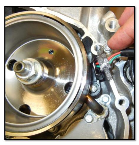
Make sure the copper washer is installed on the top cover bolt as shown.
