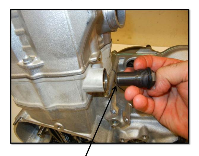
Make sure sleeve is flush with housing
