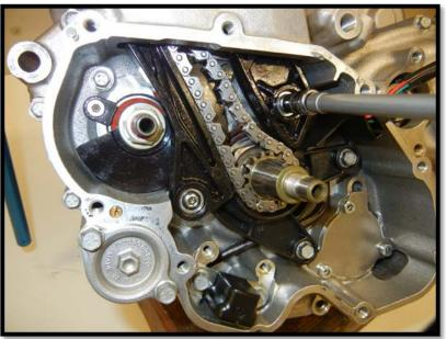
Remove the lower cam chain guide and replace with the new one supplied in the kit. <u>Use red loctite on these two bolts!</u>
