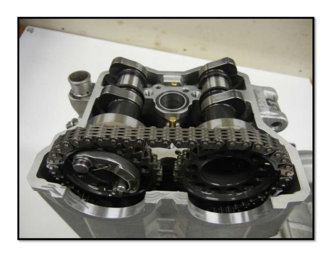
Important! Make sure the camshaft bearing housing is mounted against the lip in the cylinder head and there is no gap between them.
