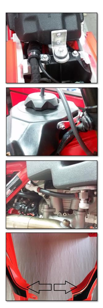
Step 14: Reconnect the battery, reinstall your seat. Fill the motorcycle with fuel and check for leaks before riding.
