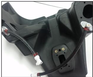
Step 3: Remove the regulator assembly along with the low fuel sensor from the stock tank. Pull the two hoses and the wire coupler far enough out to disconnect.
