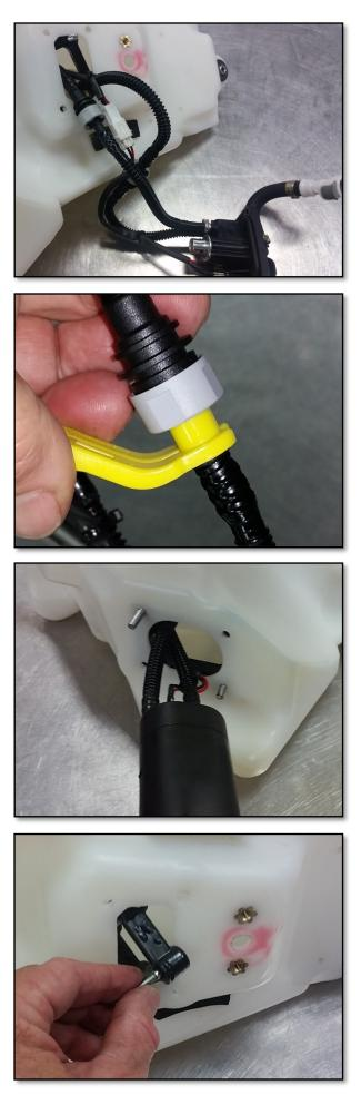
Step 7: Install the two inner support housings into the new tank. A tip is to install a couple of the nylock nuts finger tight to help keep them from falling inside the tank. You can remove them when you are ready to install the components.
