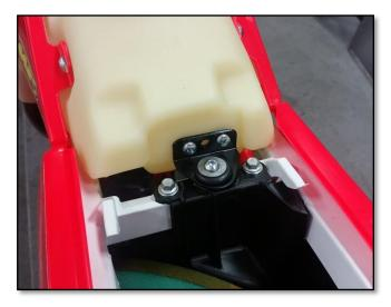
Step 5: With a razor, carefully trim both radiator shrouds at the top as shown in the photo. This will allow proper clearance to fit the tank.
