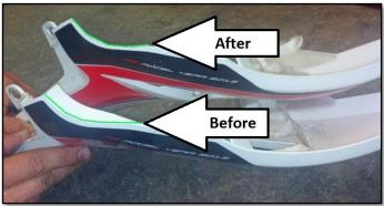
Step 6: Install the shrouds using the stock hardware everywhere except the rear mounting point which uses the remaining two 6x12 button head bolts and the two plastic washers. Install the seat hook screw from the stock gas tank.
