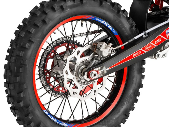
Metzeler Tires & ZF Anodized Aluminum Core/Steel Teeth Sprocket
