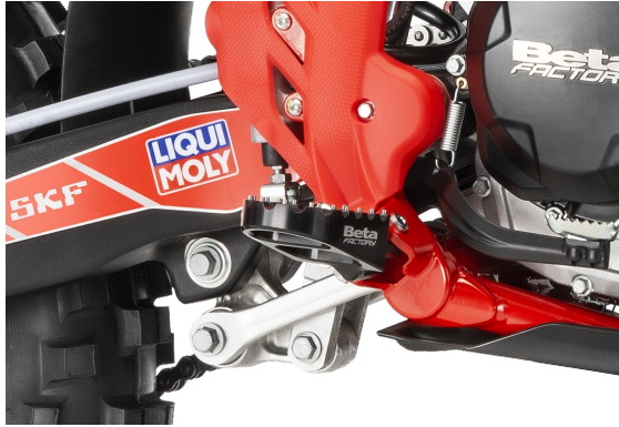
Billet Aluminum Foot Pegs & Rear Suspension Linkage
