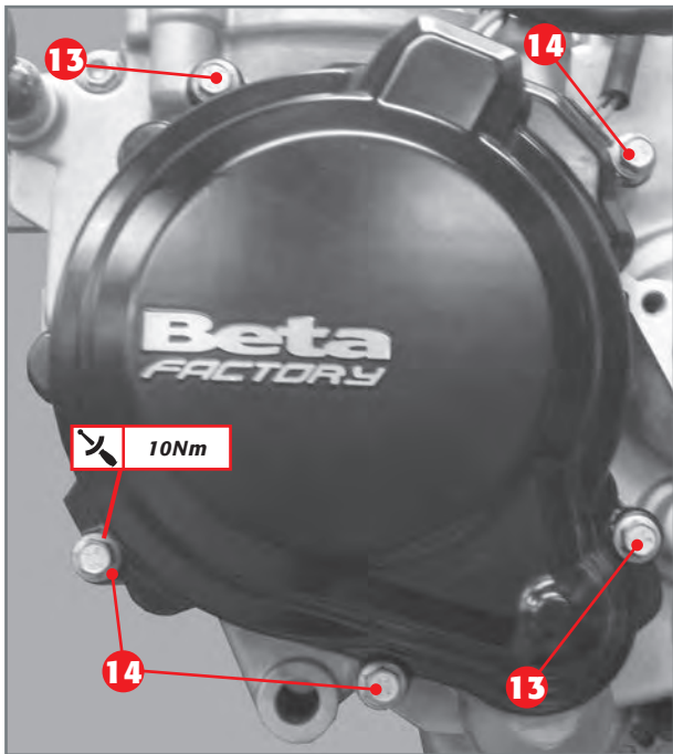
Flywheel cover coupled to crankcase.
