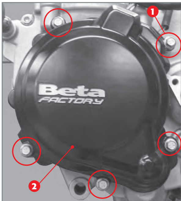
Fixing screws 1 of flywheel cover 2.
