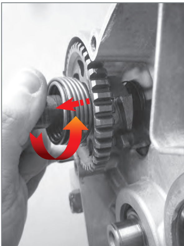
Extraction of shaft from crankcase.
