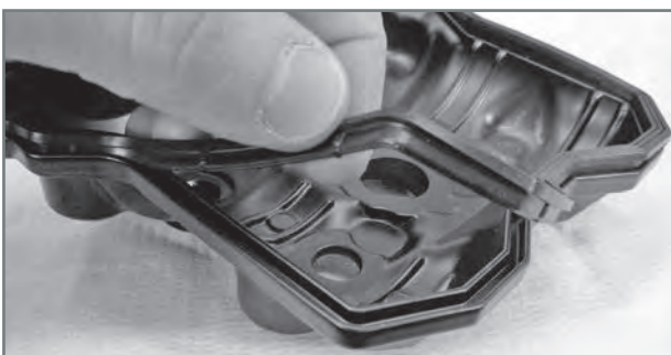
Insertion of gasket in groove on cylinder head cover.
