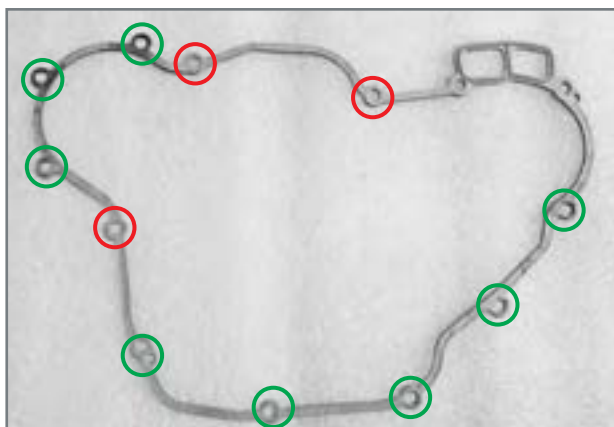
Positioning of M6x25 screws.
