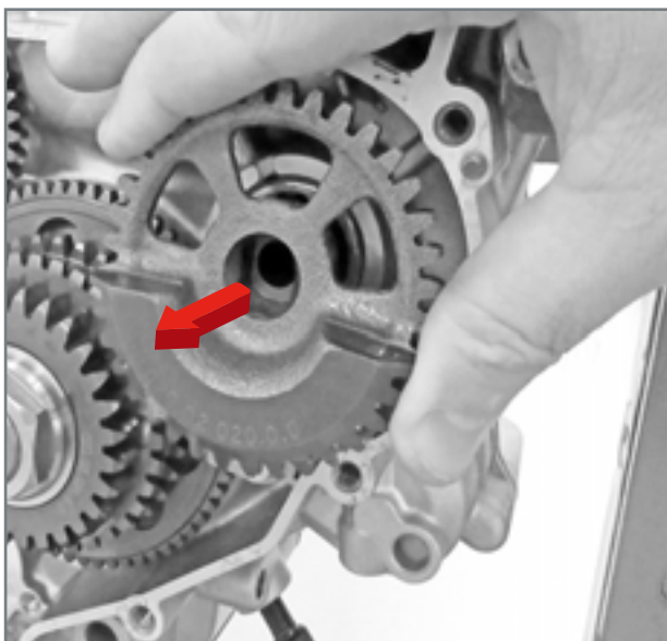
Extraction of countershaft.
