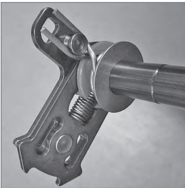
Gearshift drive shaft: note the gearshift return spring position.
