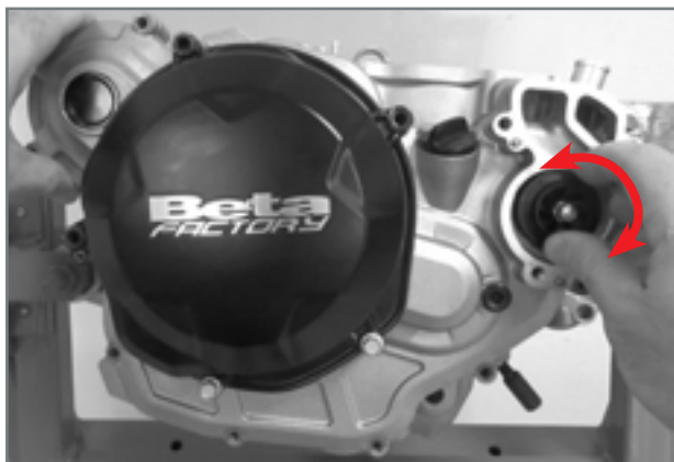
Application of complete inner clutch cover on right crankcase.
