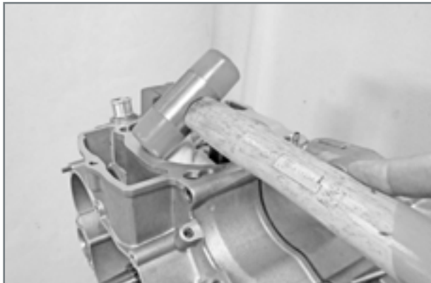
Disassembly of crankcase.
