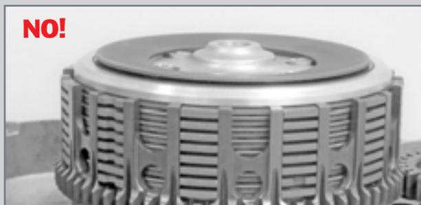
Detail of incorrect fitting of the spring washer.
