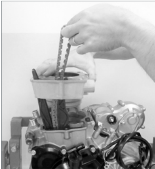
Passing the chain through the cylinder.
