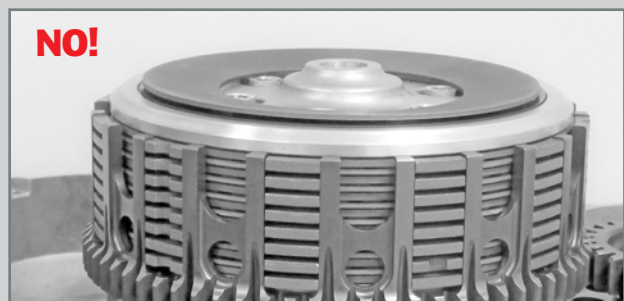
Detail of incorrect fitting of the spring washer.
