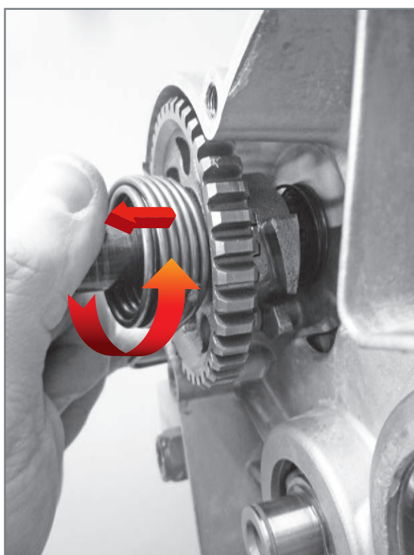
Extraction of shaft from crankcase.
