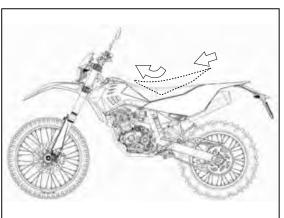
Press the saddle down in the middle and at the same time, push it forwards until the bayonet joint engages in its seat.
