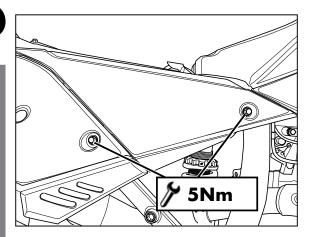
Put the screws back in and tighten to the specified torque.
