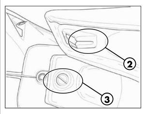
To re-assemble: Insert the cavity **2** of the saddle in slot **3**.
