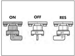
**OFF**: fuel supply closed. Fuel cannot pass from the tank to the carburettor.
