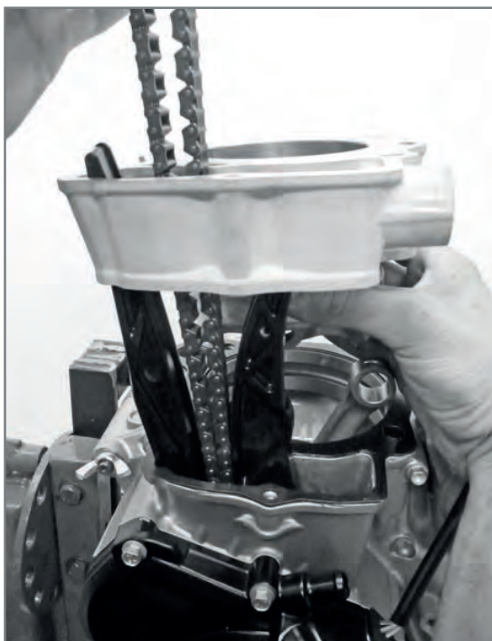
Passage of chain in cylinder.
