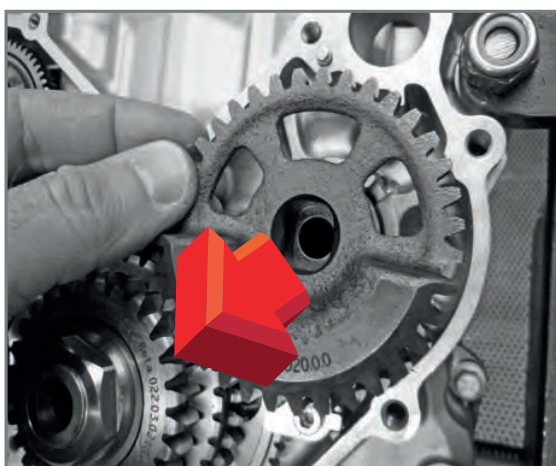
Extraction of countershaft.
